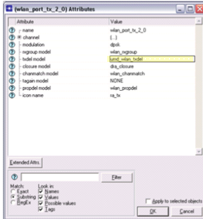
Figure B-3. The ‘txdel model’ file controls the delay between packets for the transmitter. To enable unique data rates, this file needed to be modified for the hybrid linking scheme.
