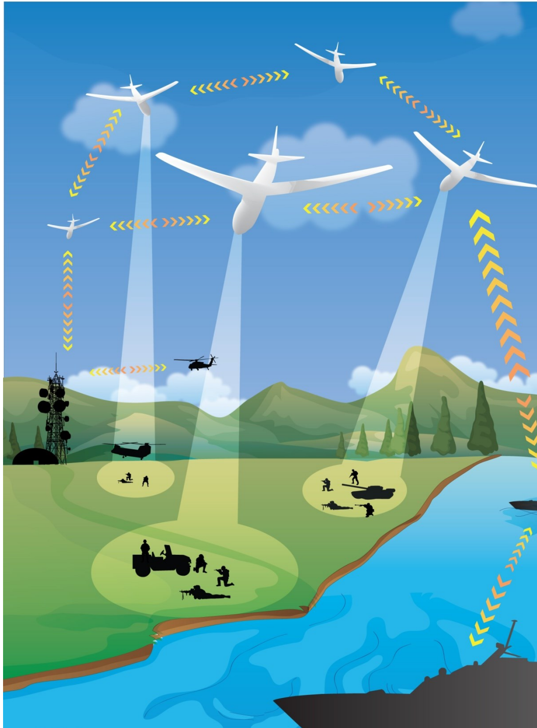
Figure 1-1. A two-tier directional wireless backbone network architecture consists of 1) airborne, maritime, and ground units using directional point-to-point links acting as the backhaul entities and 2) numerous terrestrial end-users using RF subnets. This serves as the network framework for this dissertation.
