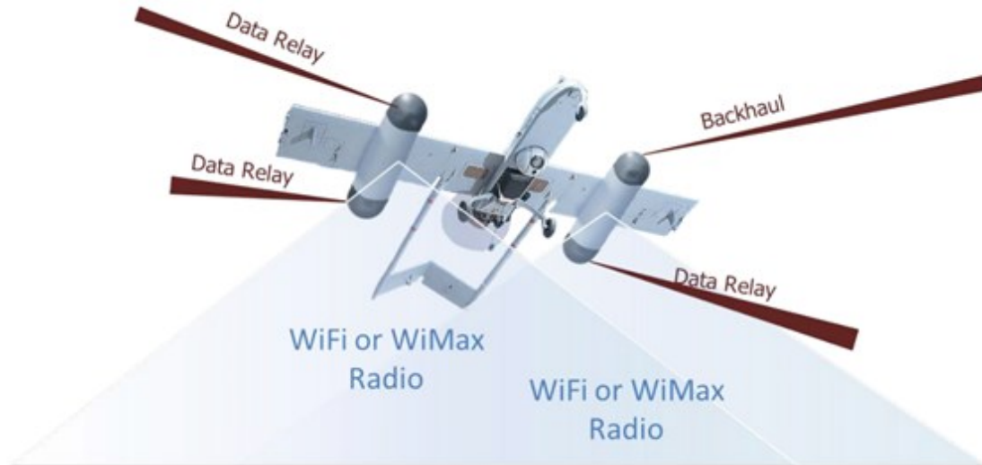
Figure 3-2. The AAI-RQ7 Shadow unmanned autonomous system (UAS) is the preferred platform by DARPA for current DWB network research. A notional drawing of the UAS includes four directional antennas for data relay and backhaul support and two Wi-Fi or WiMax radios for cross-tier communication. This image is provided in [5].
