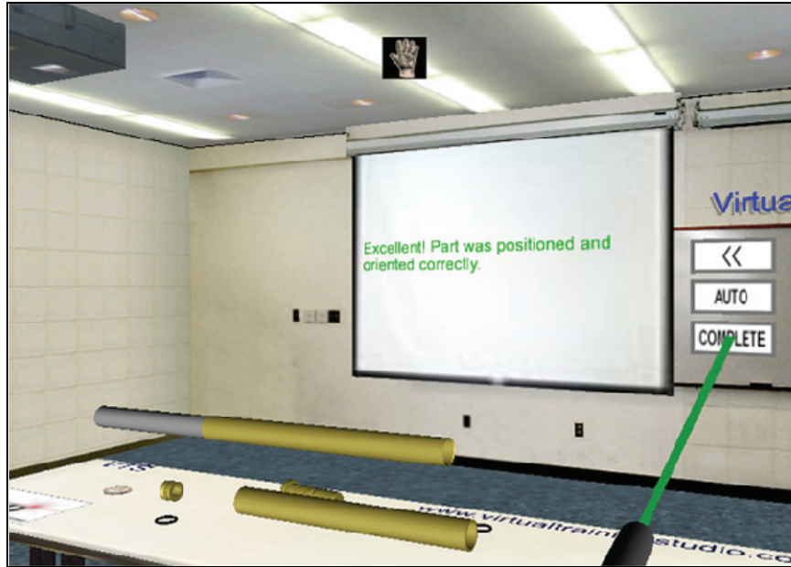
Plate 11: Placement of propellant grain at its alternate position
