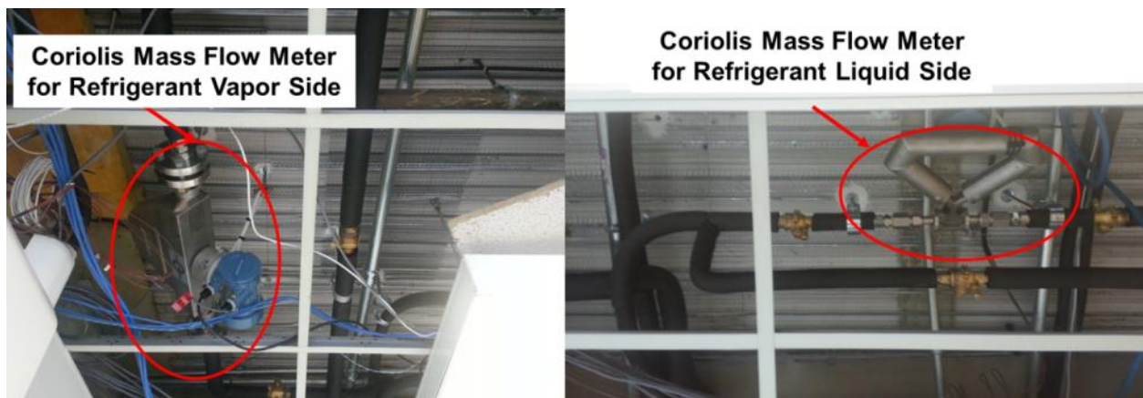
Figure 3.21: Photos of Coriolis mass flow meters in refrigerant-side
