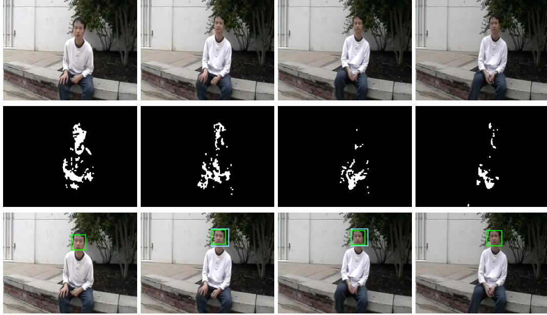
Figure 3.6: Top: frames from video used in face detection. Middle: output of IAGMM. Bottom: output of the face detector.
