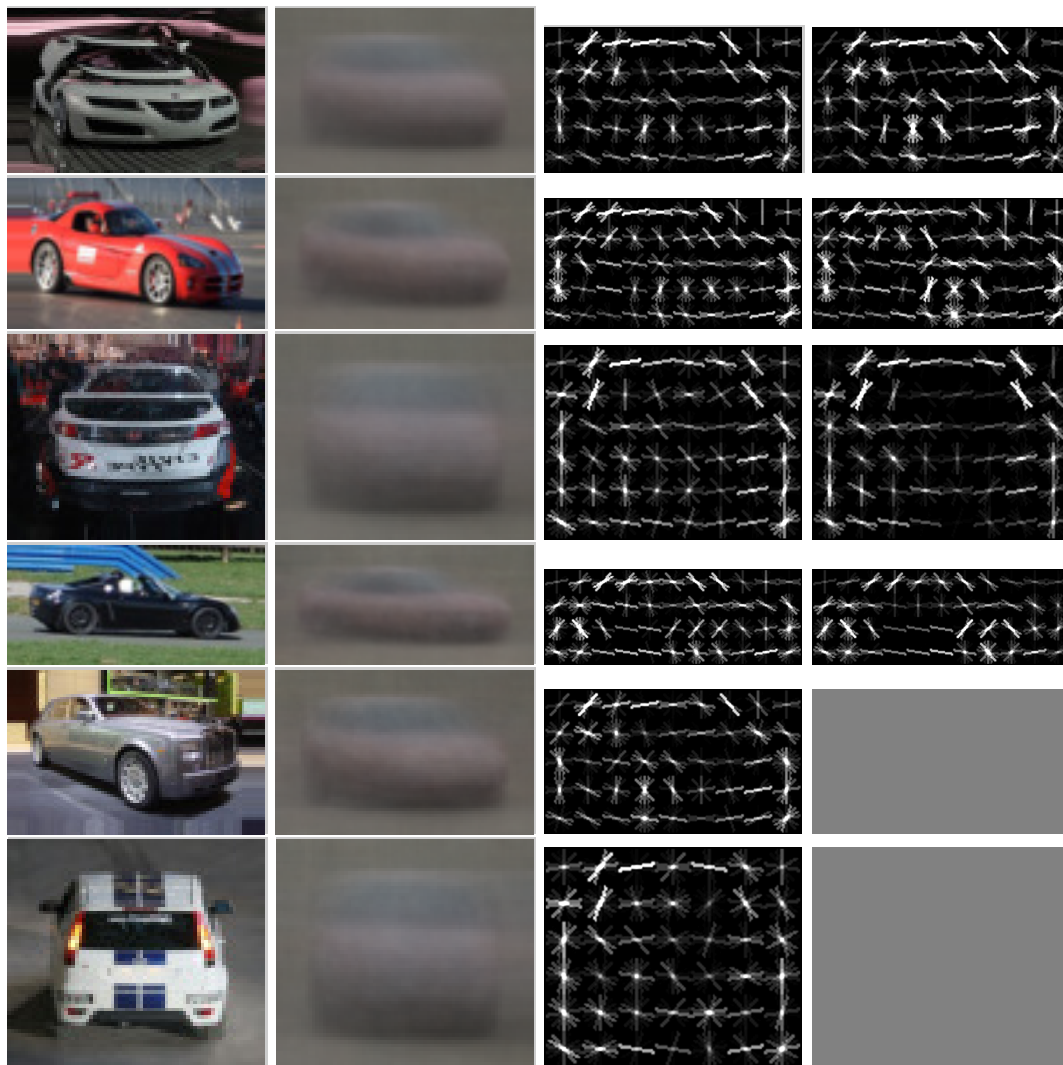
Figure 4.8: Mixture of root model before and after the training regularized by group norm for car category. Each row shows the information for a component and its symmetric counterparts are not shown to save space. Starting from the left, the first column shows a positive example from the cluster which produces the component. The second column shows the average image of the cluster. The third column shows the root filter of the component before the training. The last column shows the root filter after training. A complete gray image indicates the filter is sparse and will be removed from training the part filters and displacement parameters.
