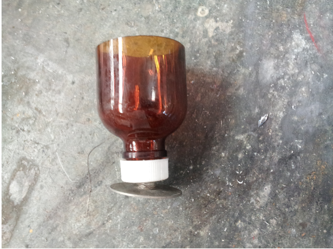
Figure A.4: Sawn-off half bottle can be seen here with electrode fit snugly into cap
