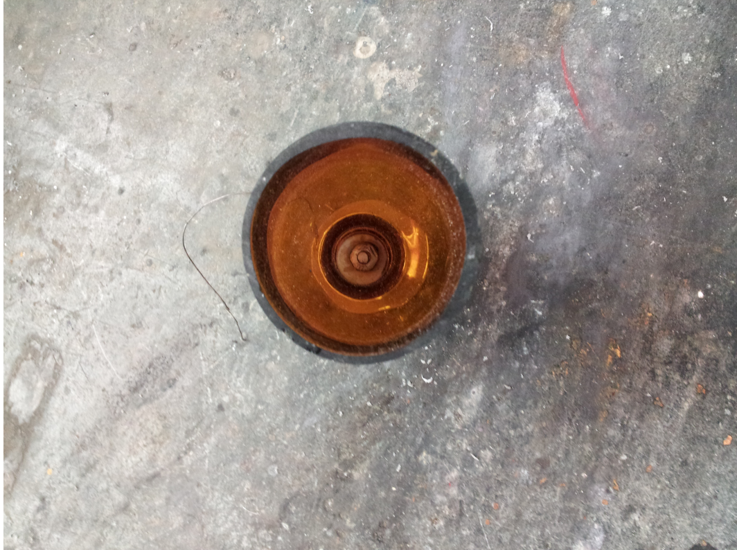
Figure A.5: Stainless steel disk, then disk, then silicon washer, should be placed onto cap (before being screwed on)
