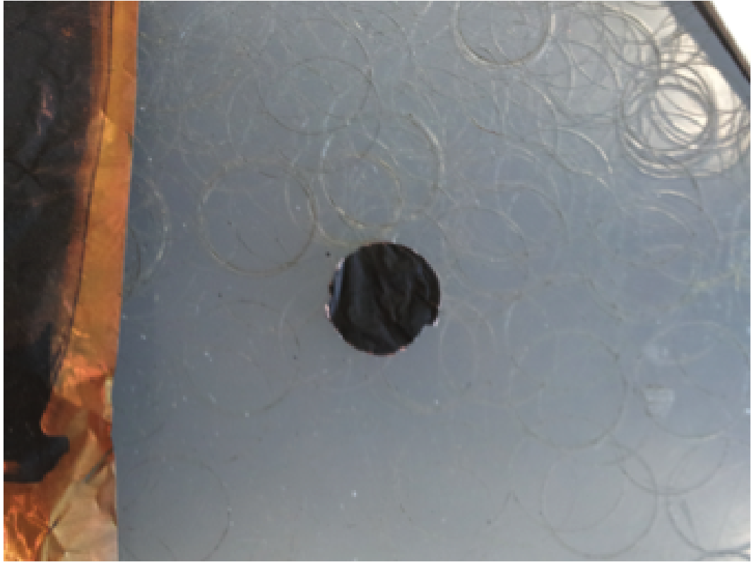
Figure A.3: Copper should not be visible after cutting disk from sheet
