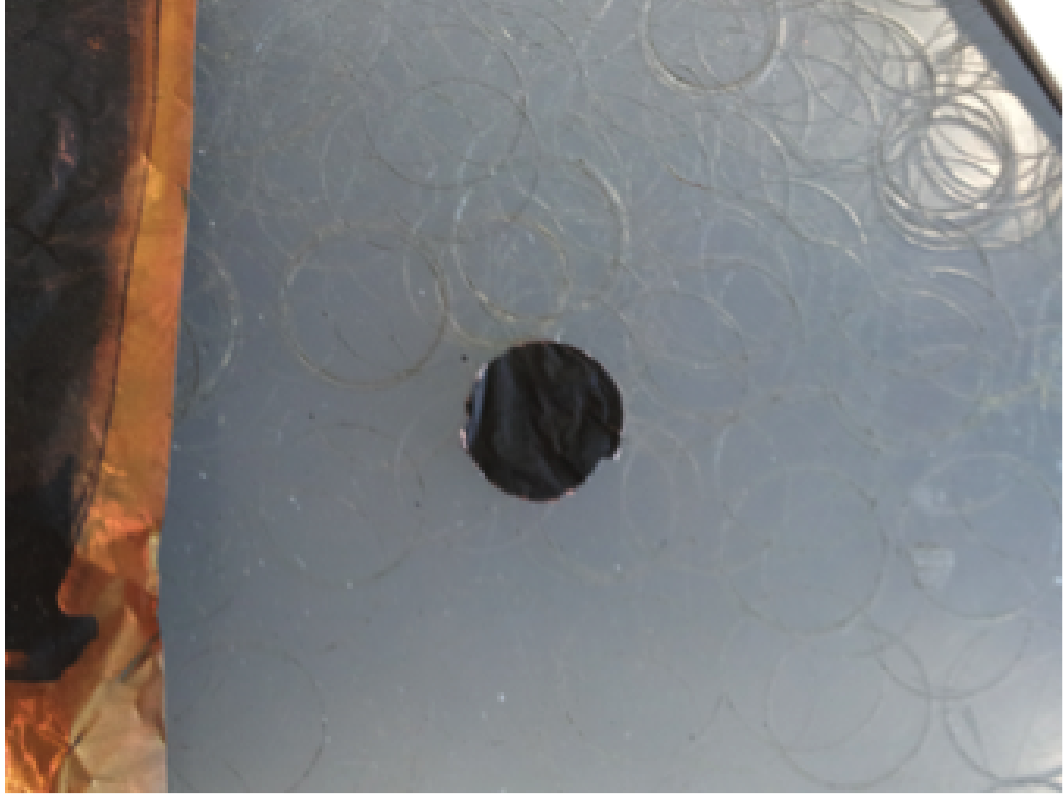
Figure A.2: Copper should not be visible after cutting disk from sheet
