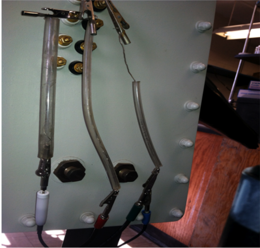
Figure A.6: External wiring that connects deposition cell to Gamry Reference 3000
