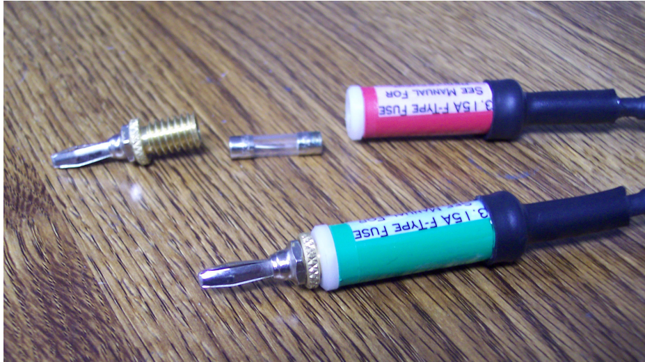
Figure 5-1 Open Fuse-holder Showing Fuse
