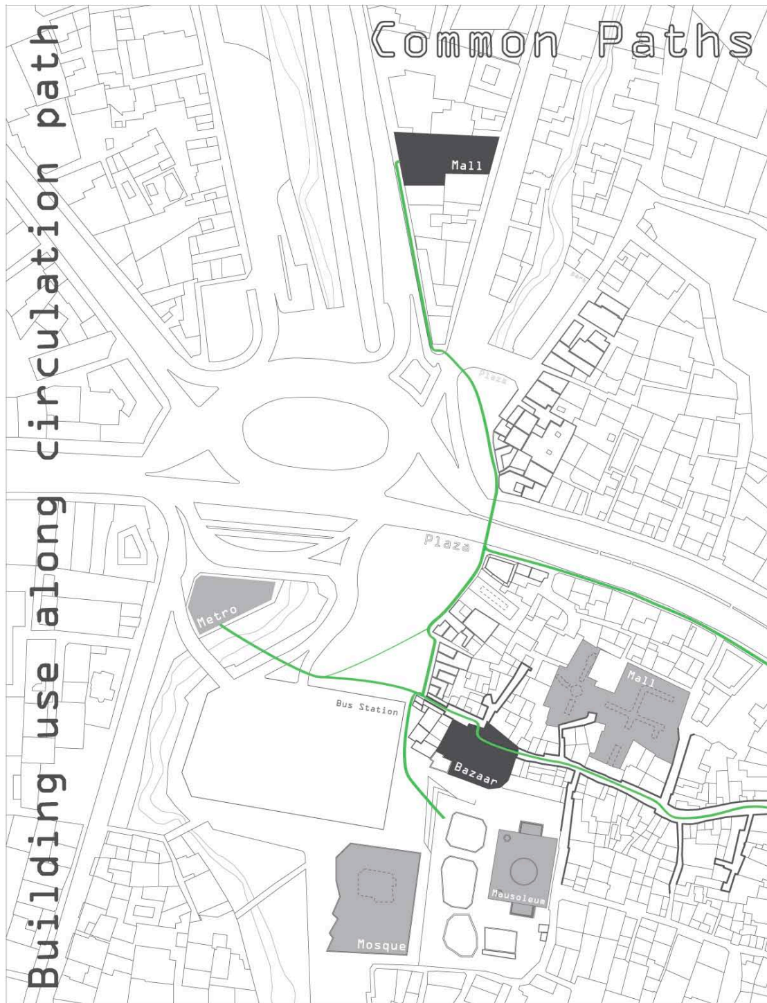
Figure 50 Redesigned, proposed site plan allowing for the creation of an open plaza and separating the circulation of the buses to the bus-station from the pedestrians accessing the Bazaar and the Mausoleum. This minor expansion provides an ample amount of space for other activities such as resting, eating, greenery, and mere circulation that is quite congested in this area. The circulation path demonstrates the path most commonly taken by the pedestrians to and from the Mall and the Bazaar and into the Future addition of the Tajrish Metro Station. [image provided by author]
