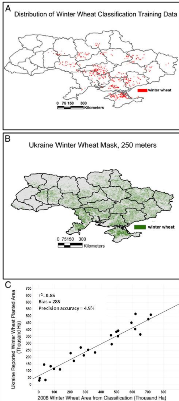
Fig. 3.2 Ukraine winter wheat mask. Panel (A) shows the distribution of the training data collected from AWiFS imagery for 2008 winter wheat crop type map for Ukraine. Panel (B) is the 2008 classified Ukraine winter wheat map at 250 m resolution. Panel (C) is the validation of the winter wheat classification map (X-axis) against the official Ukrainian SSC winter wheat oblast-level, planted area statistics (Y-axis). When compared at the oblast level, the area computed from the classified mask had a bias of 28% (SSC area=Classified_Mask_estimate * 0.72) and a precision accuracy of 4.5% relative to the official national level wheat area statistics.
