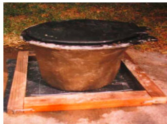
Figure 5-11: Completed pedestal placed in wooden mold
