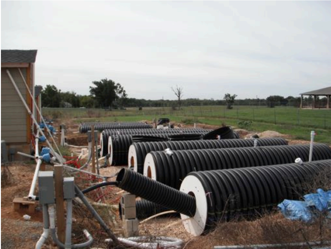
Figure 2-1 - Pilot-scale digesters developed by the University of Maryland
