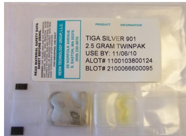
Figure 4.18: Silver conductive epoxy
