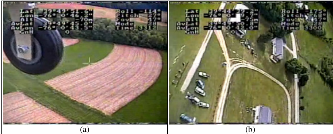
Figure 4.16: Heads Up Display in D-STAMP video stream with camera facing (a) right landing gear and (b) RC Park Facilities.
