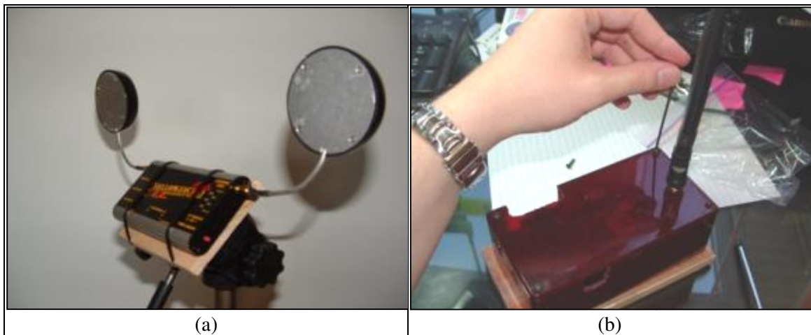
Figure 4.11: New antenna arrangement: (a) assembled directional video receiver turret and (b) serial modem mount construction.
