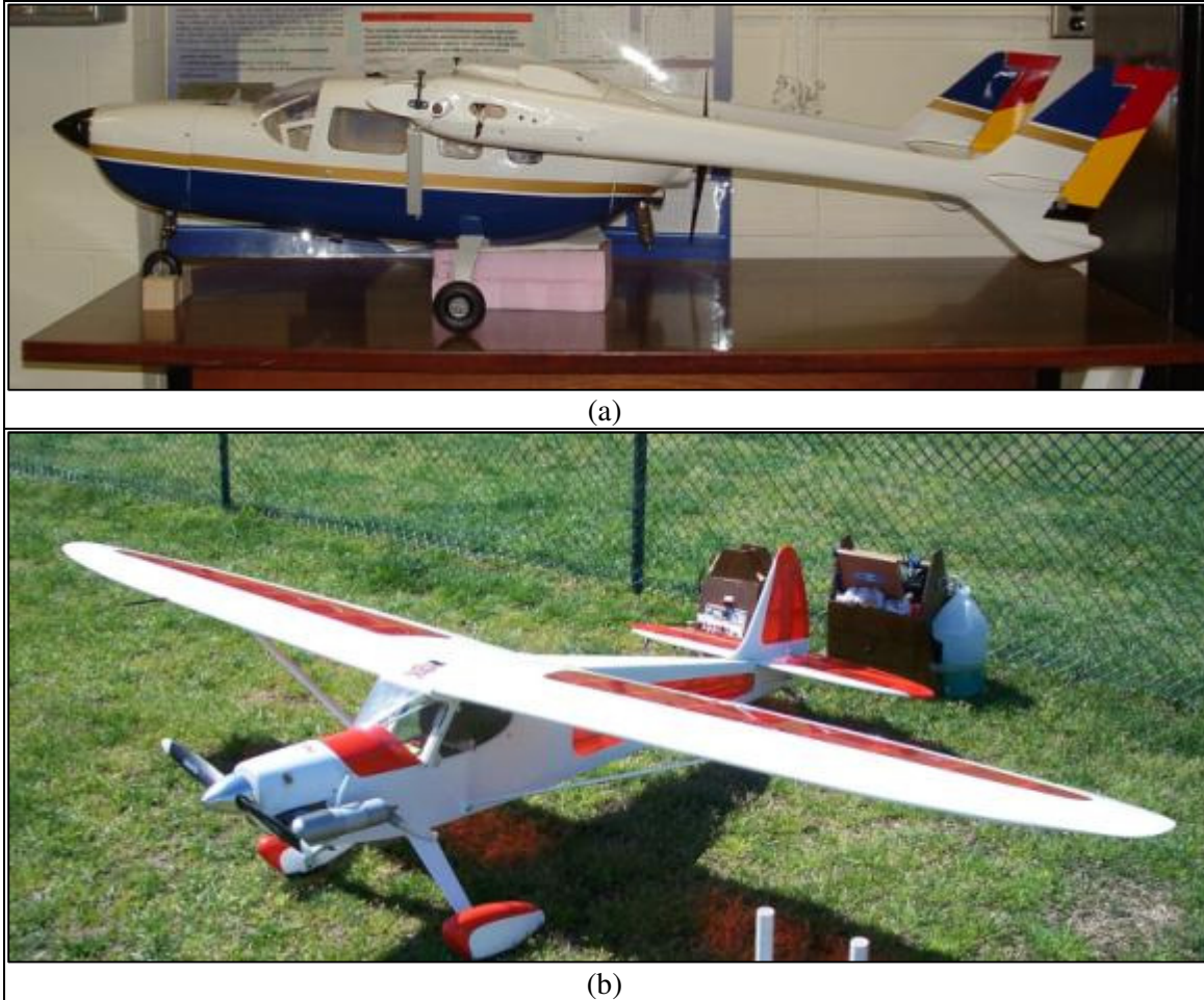
Figure 3.2: Candidate UAV airframes: (a) Cessna 337 Skymaster Model and (b) Sig Rascal 110.
