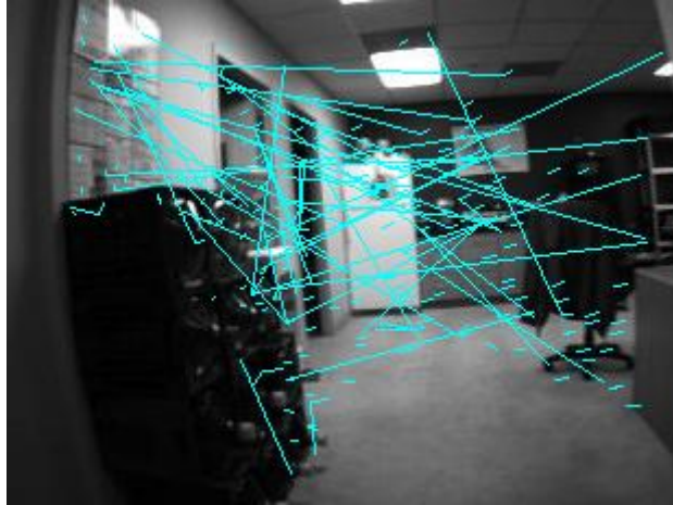
Figure 33 - Screenshot of using SURF for optic flow
