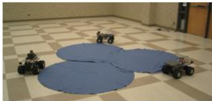
Figure 24 - Indoor experimental setup for perimeter detection [64]
