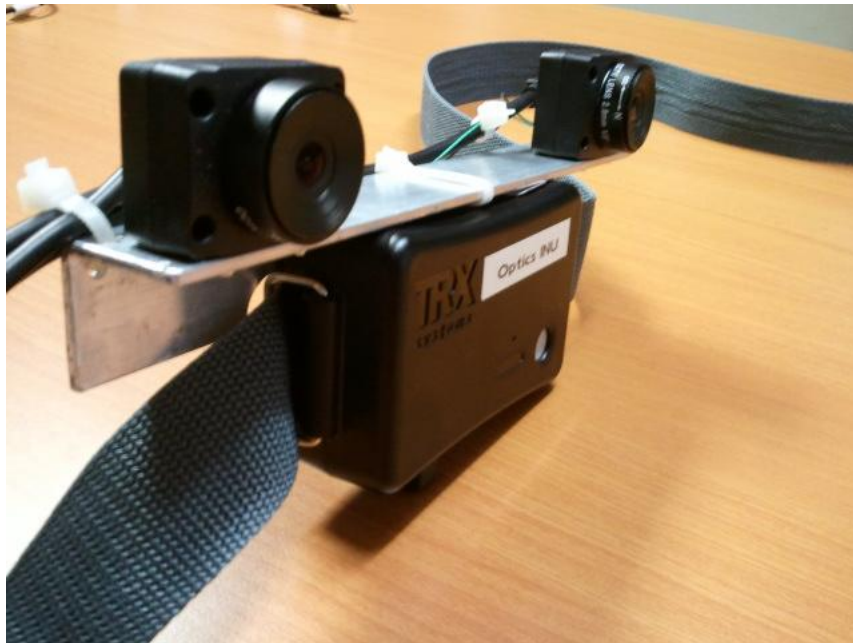
Figure 65 - Close view of the TRX INU with Point Grey cameras, the Optical INU
