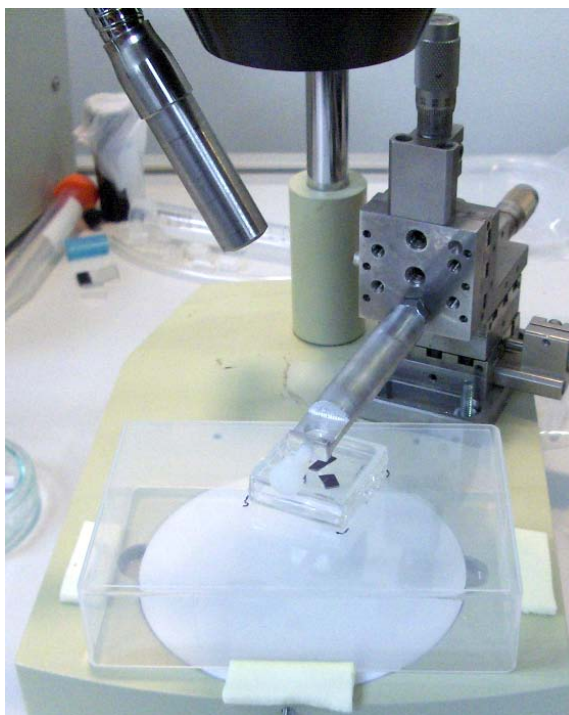
Figure 88. Cup attachment rig (courtesy Prof. Gomez). This setup gives the user a microscopic bird's eye view to precisely position the adhesive-laden reservoir over the active area of the chip without bumping into the fragile bond wires.
