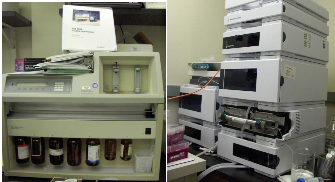
Figure 51. (left) Applied Biosystems ABI 433A Peptide Synthesizer used to make probe PNA. (right) Agilent 1200 series HPLC used for purification of crude PNA.
