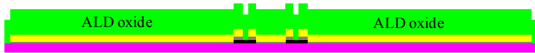
Figure 21. Illustration of cross-section of transistor after atomic layer deposition (ALD) of top-gate oxide. The oxide layer (green) is depicted as unidirectional, but actual ALD films are conformal and anisotropic.
