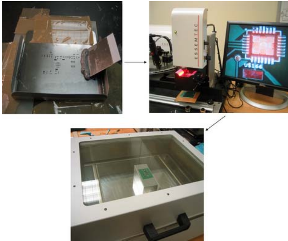
Fig. 6.19: The process to solder surface amount components on PC Boards precisely.
