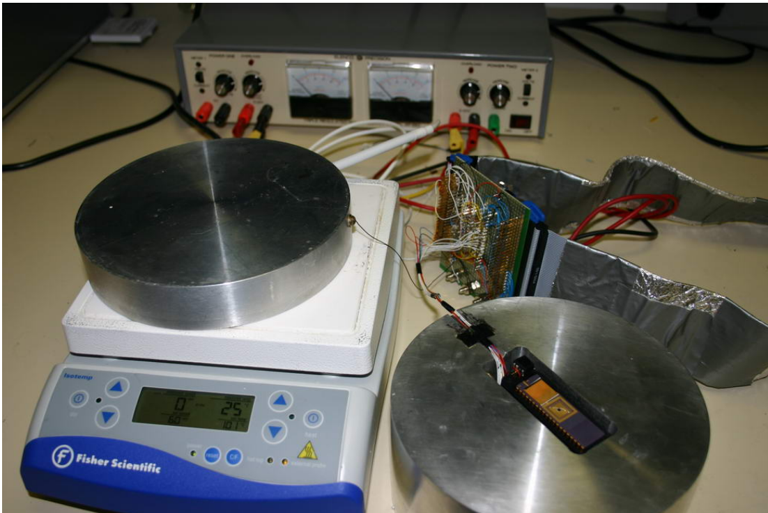
Fig. 5.7: Experimental setup for the temperature sensor.
