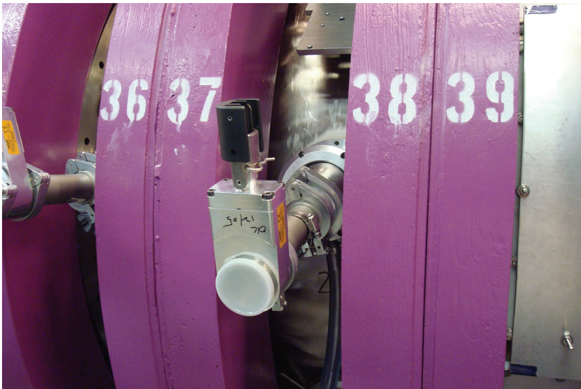
Figure 2.3: LAPD machine port equipped with ball joint and gate valve, which allows for insertion and two-dimensional movement of diagnostic probes.
