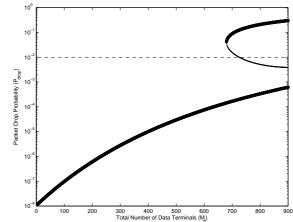
Figure 3.10: Bifurcation diagram for packet drop probability with state estimation control (maximizing throughput)( $p_{max} = 0.9$  and  $M_d$  is bifurcation parameter)
