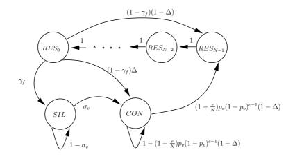
Figure 2.6: Markov Chain Model for PRMA Voice System over Random Packet Error Channel.
