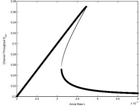
Figure 4.9: Bifurcation diagram for channel throughput  $(S_{out})$  when arrival rate  $(\lambda)$  is bifurcation parameter. M =100, p = 0.025, L = 5.
