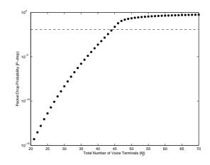
Figure 2.12: Bifurcation diagram for packet drop probability with state estimation control (minimizing  $P_{drop}$ )
