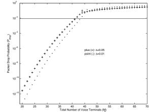
Figure 2.16: Bifurcation diagram for packet drop probability with state estimation control (maximizing throughput) ( $\Delta = 0.05$ ,  $\Delta = 0.01$ ,  $p_{v_{max}} = 0.9$ )
