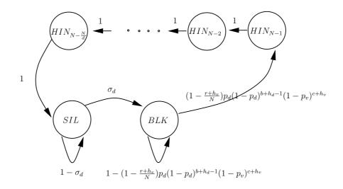
Figure 1.4: Markov chain model for PRMA-HS data subsystem.
