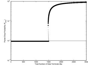
Figure 5.15: Bifurcation diagram for packet drop probability with no control  $(p = 1, M_v = 100, M_d \text{ is bifurcation}$ parameter)
