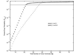
Figure 3.14: Bifurcation diagram for packet drop probability with control  $(\Delta = 0.1, \Delta = 0.01, \alpha = 0.0532, \beta = \xi = 1)$
