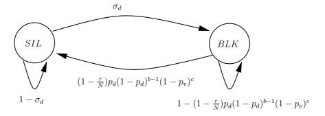
Figure 1.2: Markov chain model for PRMA data subsystem.
