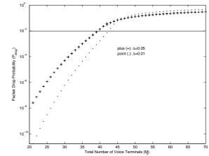
Figure 2.29: Bifurcation diagram for packet drop probability with control  $(\Delta = 0.05, \Delta = 0.01, \alpha = 1.04, \beta = \xi = 1)$
