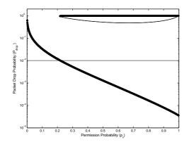
Figure 2.19: Bifurcation diagram for packet drop probability with no capture
