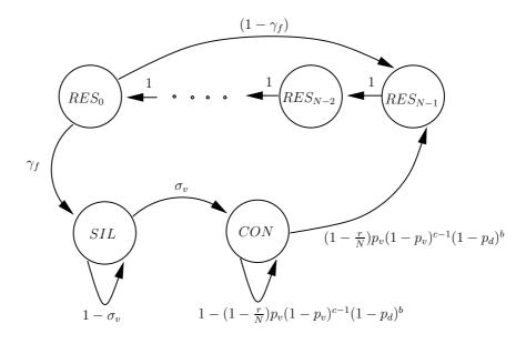
Figure 1.1: Markov chain model for PRMA voice subsystem.
