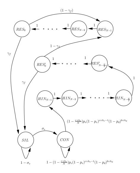
Figure 1.3: Markov chain model for PRMA-HS voice subsystem.
