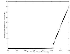
Figure 5.9: Bifurcation diagram for the number of contending terminals with no control ( $p = 1, M_d = 100, M_v$  is bifurcation parameter)
