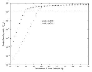
Figure 2.15: Bifurcation diagram for packet drop probability with control  $(\Delta = 0.05, \Delta = 0.01, \alpha = 0.114, \beta = \xi = 1)$
