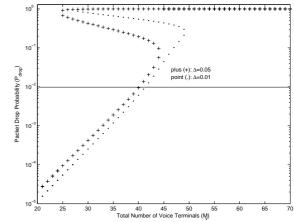
Figure 2.13: Bifurcation diagram for packet drop probability with no control ( $\Delta$  is bifurcation parameter,  $p_v = 0.3$ ,  $M_v = 25$ )
