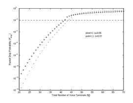
Figure 2.17: Bifurcation diagram for packet drop probability with state estimation control (minimizing  $P_{drop}$ )  $(\Delta = 0.05 \text{ and } \Delta = 0.01)$
