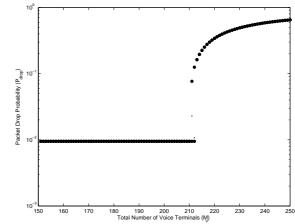
Figure 5.1: Bifurcation diagram for packet drop probability with no control  $(p_v = 1 \text{ and } M_v \text{ is bifurcation parame$  $ter})$
