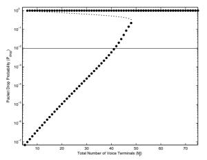
Figure 3.5: Bifurcation diagram for packet drop probability with no control  $(p = 0.3 \text{ and } M_v \text{ is bifurcation parameter})$
