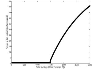
Figure 5.17: Bifurcation diagram for the number of contending terminals with no control ( $p = 1, M_v = 100, M_d$ is bifurcation parameter)
