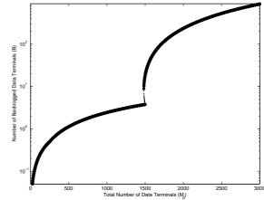
Figure 5.21: Bifurcation diagram for the number of backlogged data terminals with no control ( $p = 1, M_v = 100, M_d$  is bifurcation parameter)
