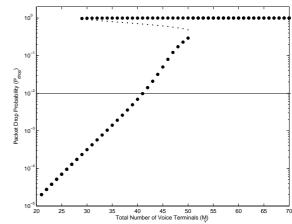
Figure 2.21: Bifurcation diagram for packet drop probability with no control  $(p_v = 0.2)$
