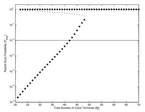
Figure 2.23: Bifurcation diagram for packet drop probability with no control  $(p_v = 0.4)$
