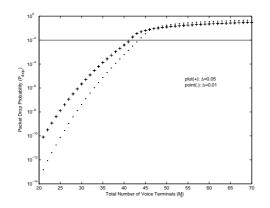
Figure 2.31: Bifurcation diagram for packet drop probability with state estimation control (minimizing  $P_{drop}$ ) for  $\Delta = 0.05$  and  $\Delta = 0.01$ .
