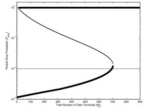
Figure 3.6: Bifurcation diagram for the packet drop probability with no control  $(p = 0.2 \text{ and } M_d \text{ is bifurcation parameter})$
