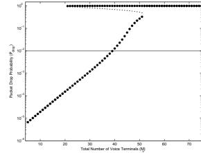
Figure 3.3: Bifurcation diagram for packet drop probability with no control  $(p = 0.1 \text{ and } M_v \text{ is bifurcation parameter})$
