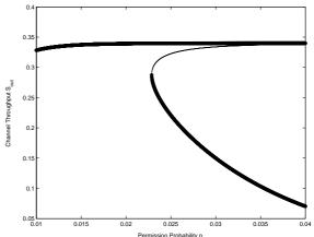
Figure 4.5: Bifurcation diagram for channel throughput  $(S_{out})$  when permission probability (p) is bifurcation parameter.  $M = 100, \lambda = 0.0034,$ L = 5.
