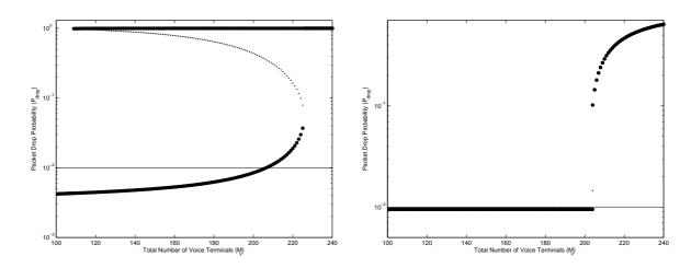
Figure 5.7: Bifurcation diagram for packet drop probability with no control  $(p = 1, M_d = 100, M_v \text{ is bifurcation}$ parameter)
