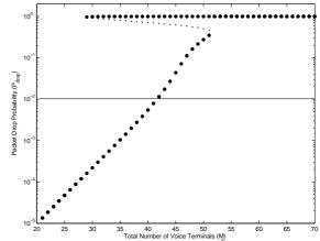
Figure 2.7: Bifurcation diagram for packet drop probability with no control  $(p_v = 0.2)$
