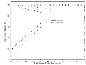
Figure 2.28: Bifurcation diagram for packet drop probability with no control  $(p_v = 0.3 \text{ and two different values for} \Delta)$
