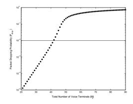
Figure 2.18: Bifurcation diagram for packet dropping probability with power capture  $(q_1 = 0.2 \text{ and } q_2 = 0.8)$
