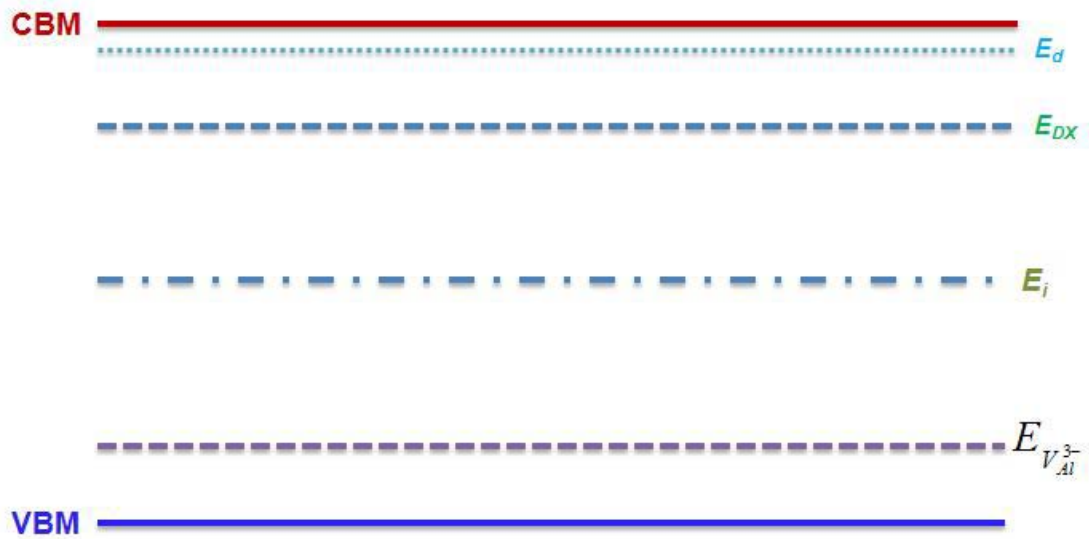
Fig. 3.13: Energy band diagram of In_xAl_{1-x}N film resistor[90, 91]
