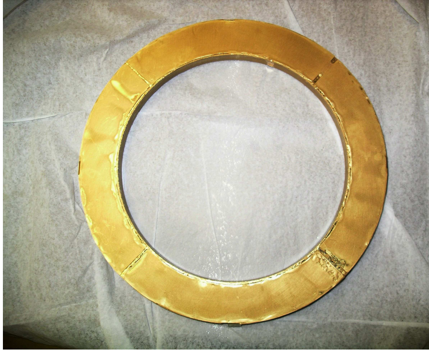
Figure 2.8: Capacitor plates with gold-coating.
