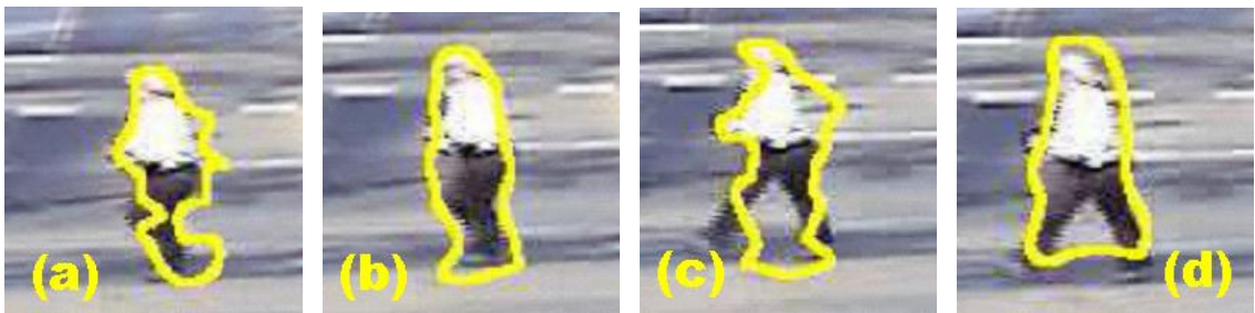
Figure 3.7: Comparisons between tracking results with and without subspace regulation. (a) and (c) are without regulation, (b) and (d) are with regulation.
