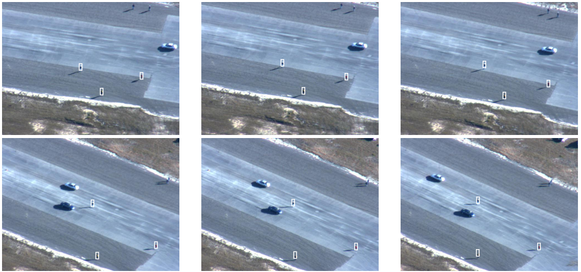
Figure 2.6: Multiple-target tracking in an airport. In this sequence, as the intensities of the targets are different from the background, the appearance cues become dominant in the observation model.
