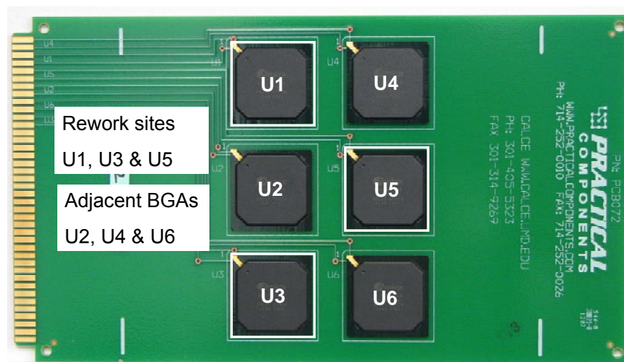
Figure 64: Test vehicle with 6 BGAs on a PCB
