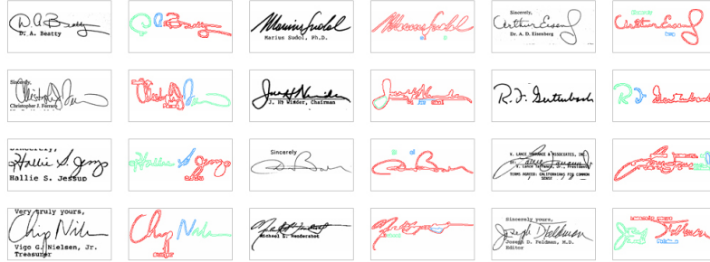
Figure 3.10: Examples of detected signatures from the Tobacco-800 database, together with their saliency maps. The top three most salient parts are shown in red, green, and blue, respectively.
