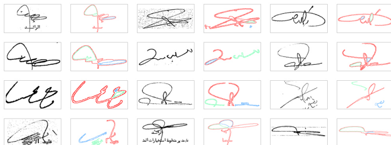
Figure 3.11: Examples of detected signatures from the Maryland Arabic database, together with their saliency maps. The top three most salient parts are shown in red, green, and blue, respectively.
