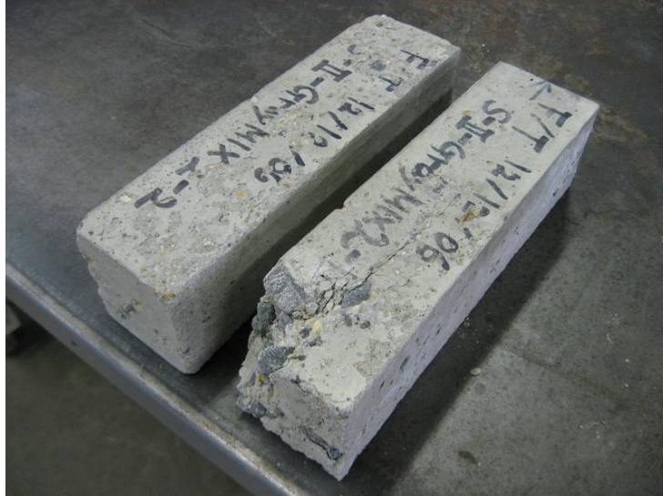
Figure 4.2 7 MPa CCA at 356 kg/m 3 Mixture after 300 Freeze Thaw Cycles
