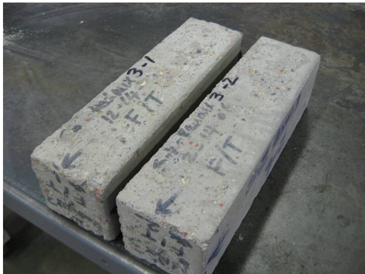
Figure 4.3 21 MPa CCA at 356 kg/m 3 Mixture After 300 Freeze Thaw Cycles
