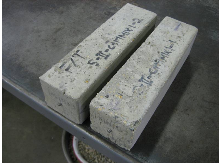
Figure 4.1 Control Mixture after 300 Freeze Thaw Cycles
