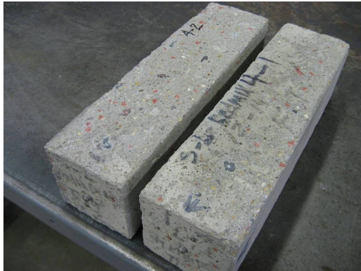
Figure 4.4 21 MPa CCA at 100% Coarse Mixture After 300 Freeze Thaw Cycles
