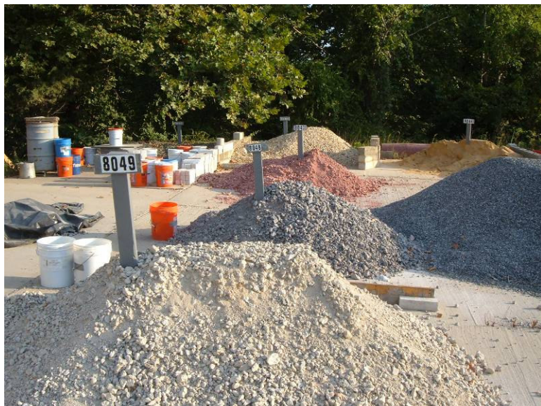
Figure 3.2 CCA pigmented with different colors (Red=21 MPa at far back, Black=34 MPa in the middle, Gray=7 MPa in the front)
