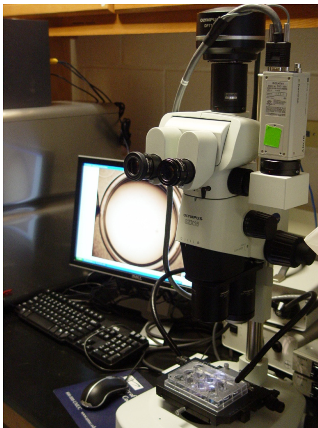
Figure 2-3. Set-up for microscopy video evaluation of C. virginica settlement behavior.
