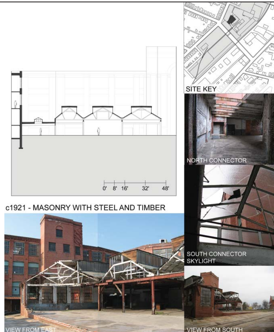
Figure 89: Building 7 Documentation. This building is one of the most damaged and partially collapsed. [Images and photographs by author.]
