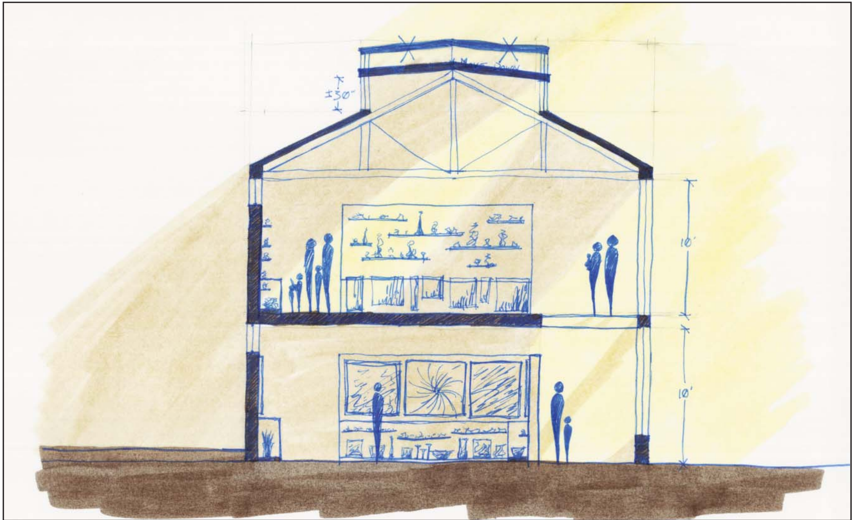
Figure 146: Sectional Light Study. This sketch shows some of the interior character of the building and the way in which natural light impacts the spaces. [Image by author.]
