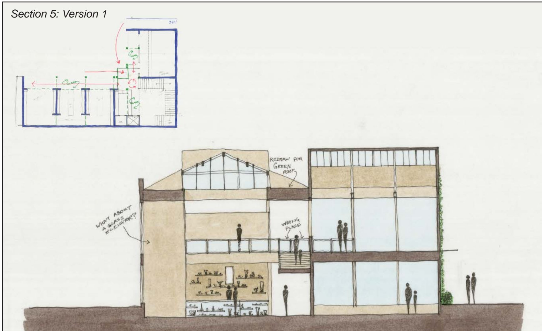
Figure 142: Plan and East-West Section of an Early Scheme. This early take on an L-shaped building used a corner entry and lobby with wings for gallery space. The corner entry was problematic and later abandoned for a more straightforward entry. [Image by author.]
