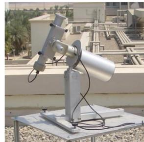
Figure 4: Pyranometer and Pyr heliometer
