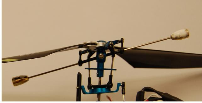
Figure 1.3: Flybars are used to mechanically stabilize helicopters.
