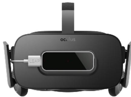
Figure 8: Front view of Leap Motion Controller attached to the Oculus Rift (Hunt, 2016).
