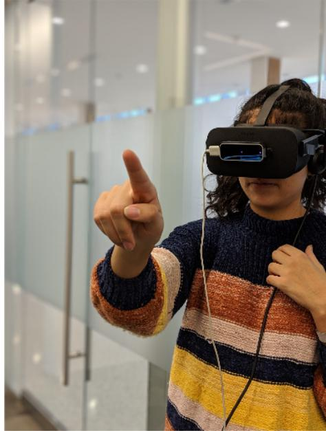
Figure 9: Example of a user operating the Oculus Rift with the Leap Motion Controller attached in front.
