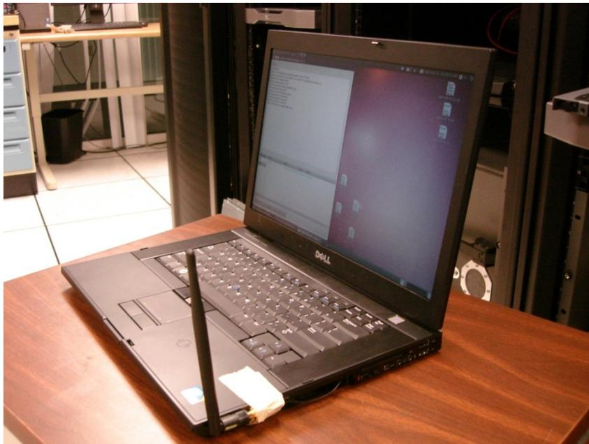
Figure 4.1: Dell Latitude Showing Antenna Mount
