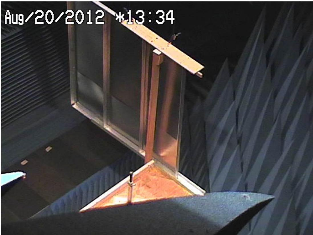
Figure 5.11: Anechoic Chamber used to Measure Antenna Gain Patterns
