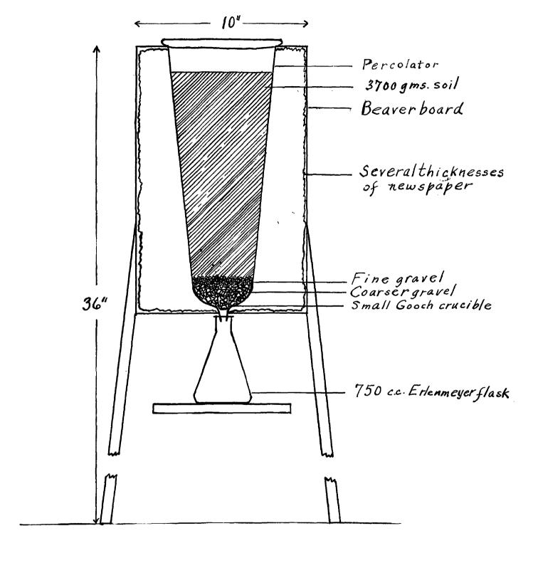
Fig. 1 Cross-section of Stand.
