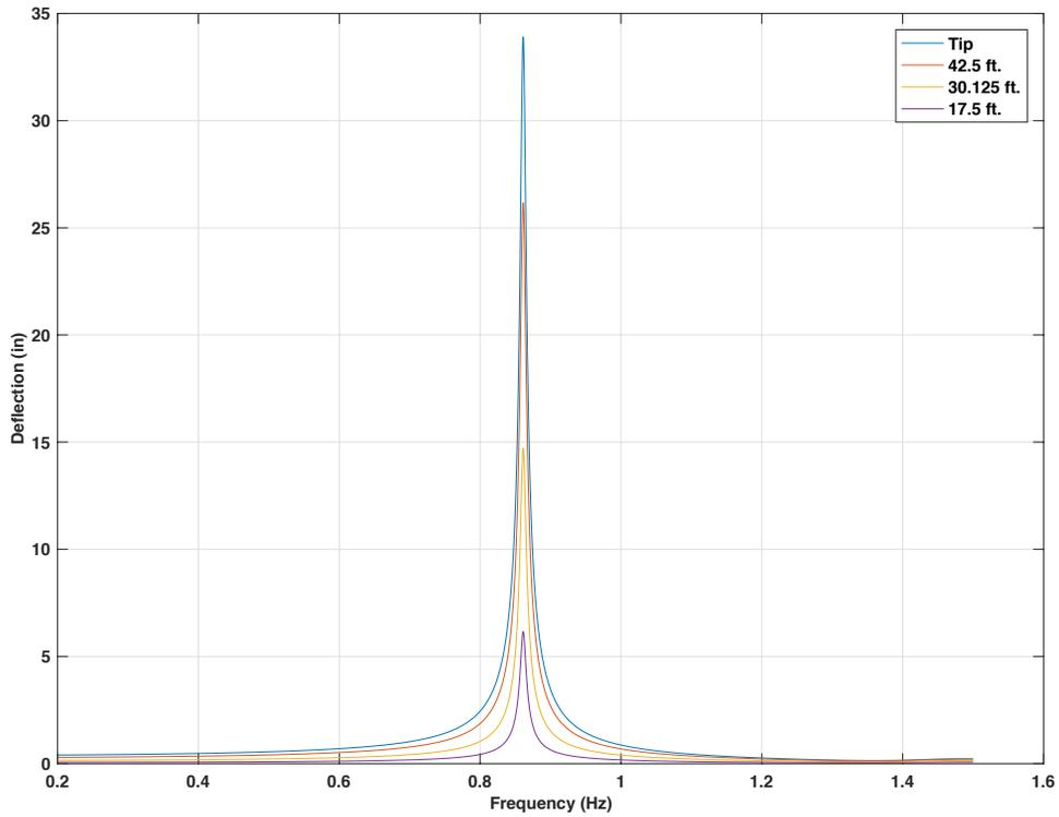
Figure 4-142 Frequency response for 50ft. mast arm with 15lb mass TMD, 5 lbf force on tip,  $f_d = 1.5 f_n$
