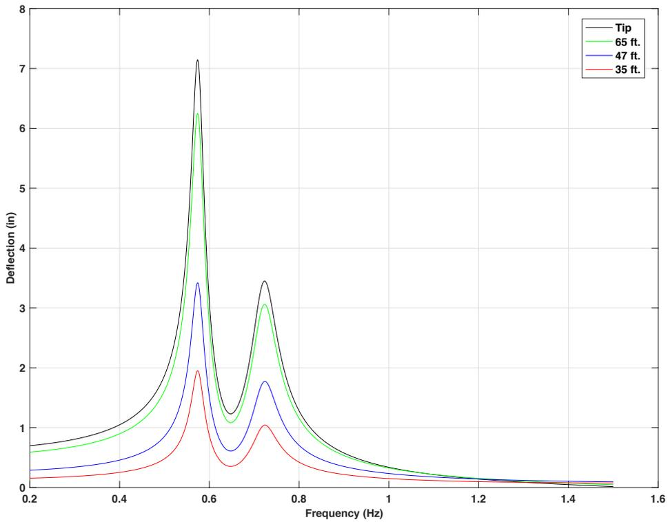
Figure 4-54 Frequency response for 70ft. mast arm with 15 lb. mass TMD at 5 ft from the tip  $f_d = 1.0f_n$ , 5 lbf force on tip of mast arm
