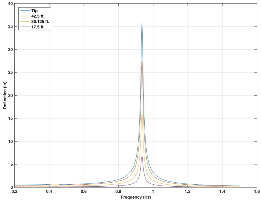
Figure 4-133 Frequency response for 50ft. mast arm with 15lb mass TMD, 5 lbf force on 3 signal heads location,  $f_d = 0.5 f_n$
