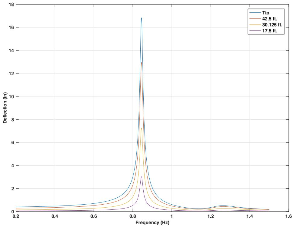
Figure 4-140 Frequency response for 50ft. mast arm with 15lb mass TMD, 5 lbf force on tip,  $f_d = 1.25 f_n$
