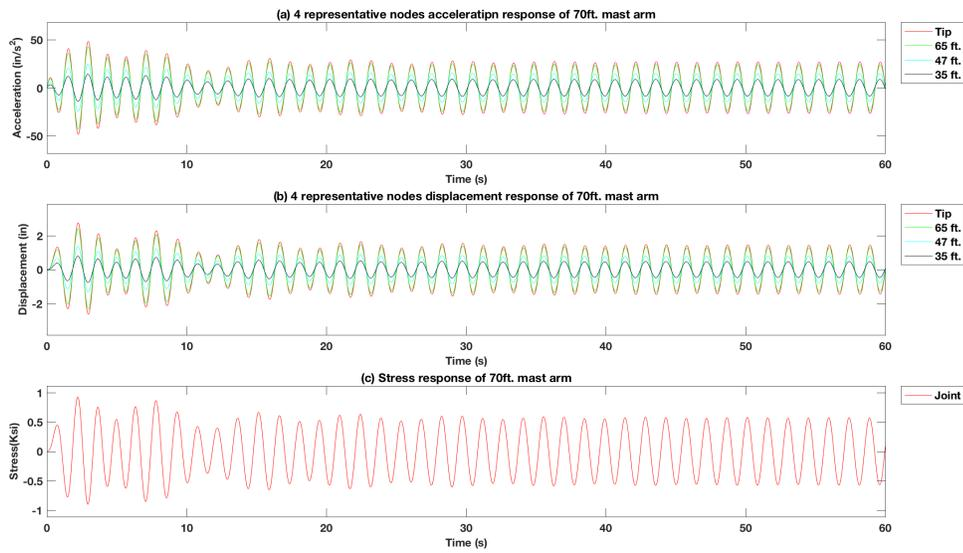
**Figure 4-18 Force vibration response of excitation force at signal heads' location of the 70 ft. mast arm signal pole structure model with 25 lb. mass TMD using the  $f_s = 1.1 f_n$**
