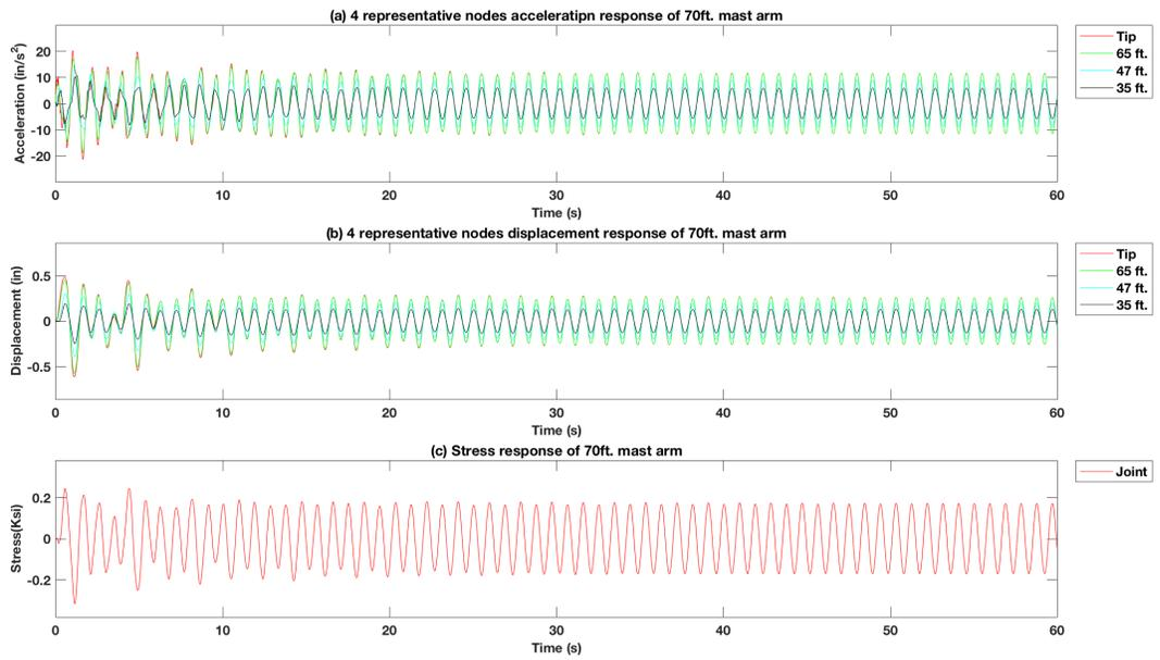
Figure 4-15 Force vibration response of excitation force at tip of the 70 ft. mast arm signal pole structure model with 25 lb. mass TMD using the  $f_x = 0.6f_n$
