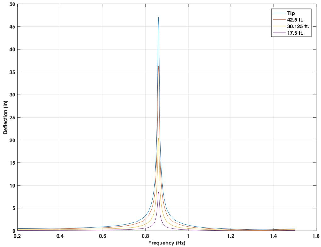
Figure 4-143 Frequency response for 50ft. mast arm with 15lb mass TMD, 5 lbf force on 3 signal heads location,  $f_d = 1.5 f_n$
