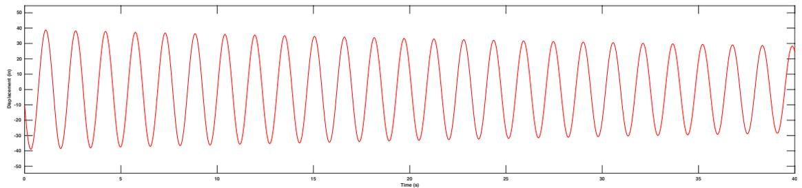
**Figure 3-7 Free vibration displacement response using ANSYS model with distributed mass and mass of signal heads**
