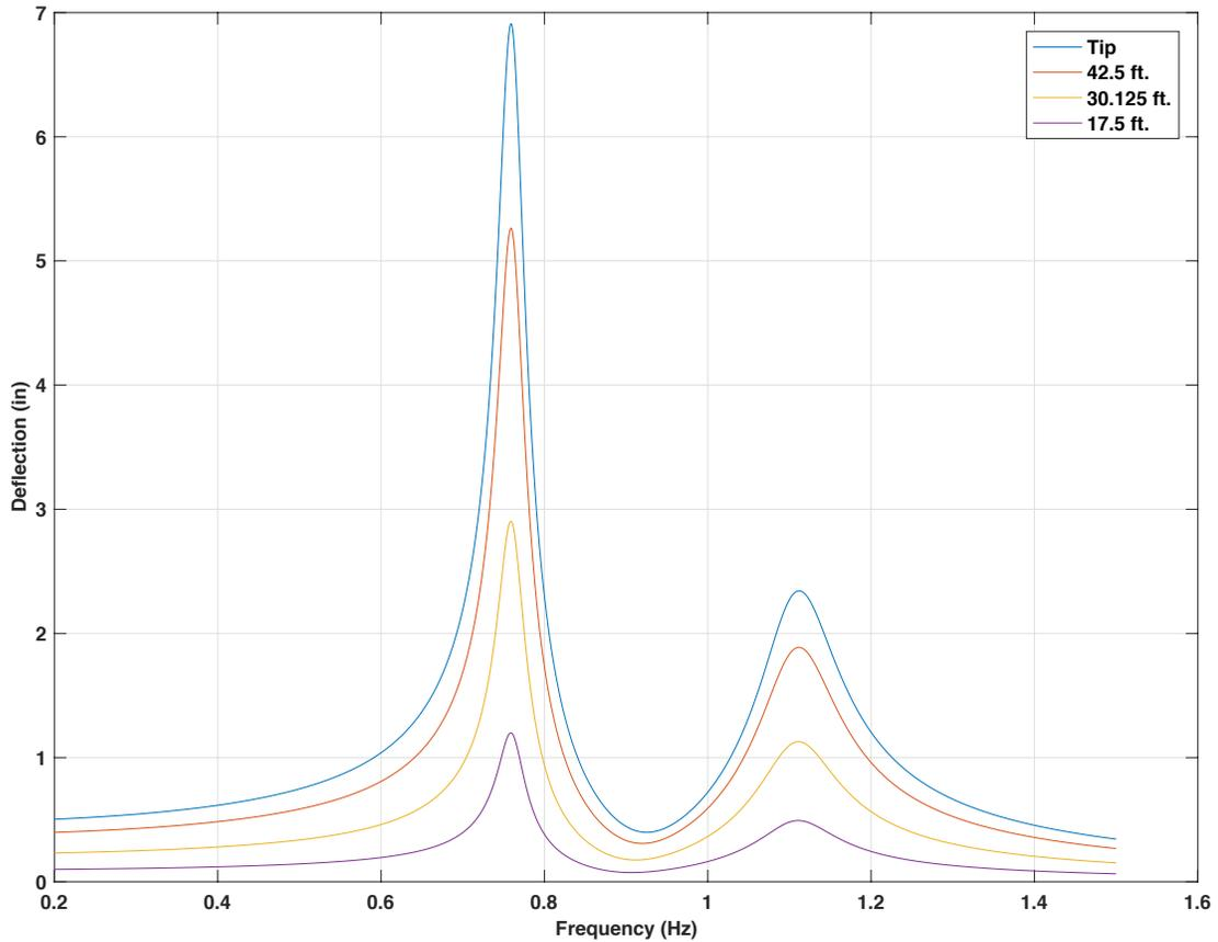
**Figure 4-121 Frequency response for 50ft. mast arm with 25lb mass TMD, force on signal heads' location**
