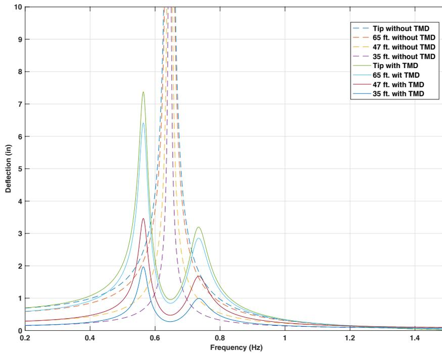
Figure 3-12 Harmonic Analysis for the finite element model using 15lb. mass TMD
