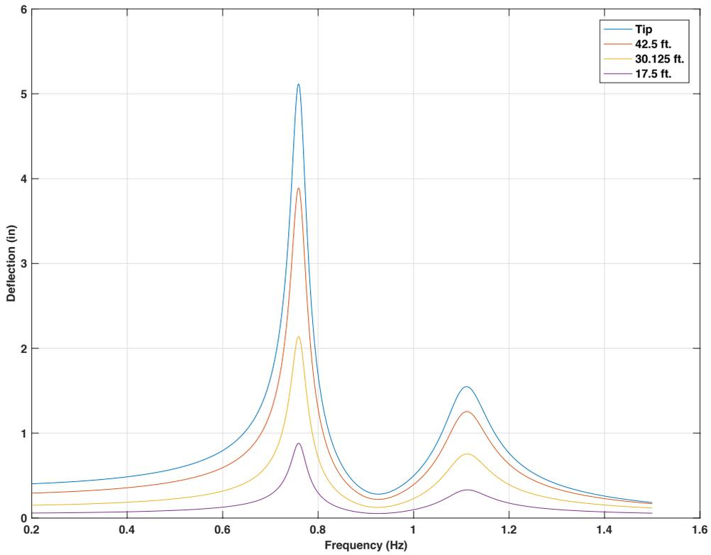
**Figure 4-120** Frequency response for 50ft. mast arm with 25lb mass TMD, force on the tip
