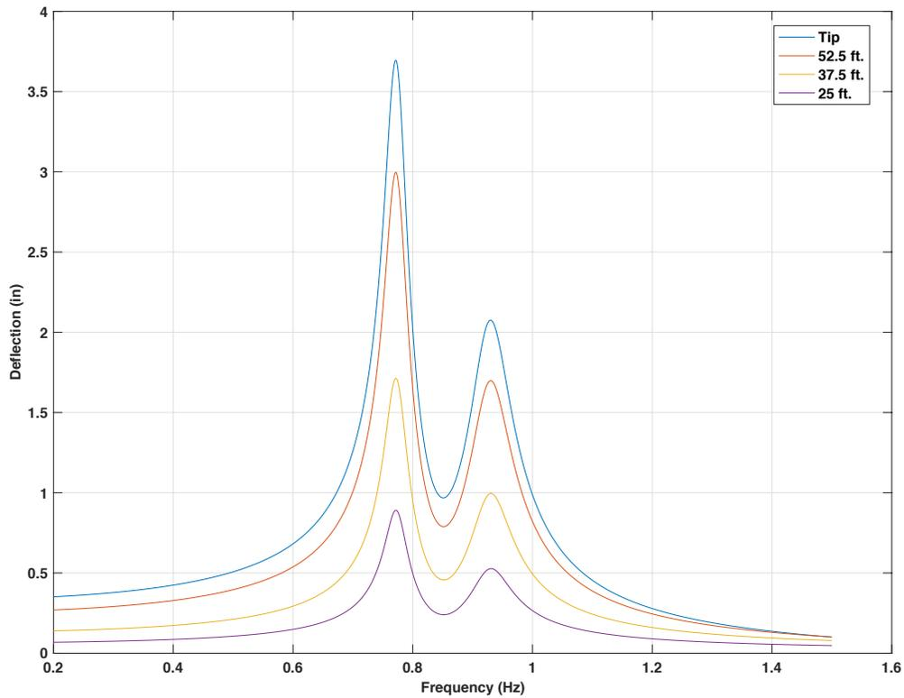
Figure 4-108 Frequency response for 60ft. mast arm with 15 lb. mass TMD at 2.5 ft from the tip
