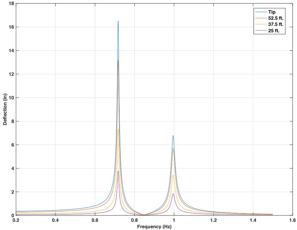
Figure 4-147 Frequency response for 50ft. mast arm with 25 lb. mass TMD using the  $\zeta = 1\%$ , 5 lbf force on tip of mast arm
