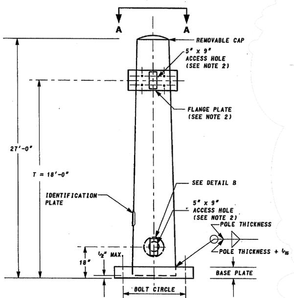
Figure 3-1 Standard Single Mast Pole (Signal Standard No. MD 818.06, 2007 Revised)
