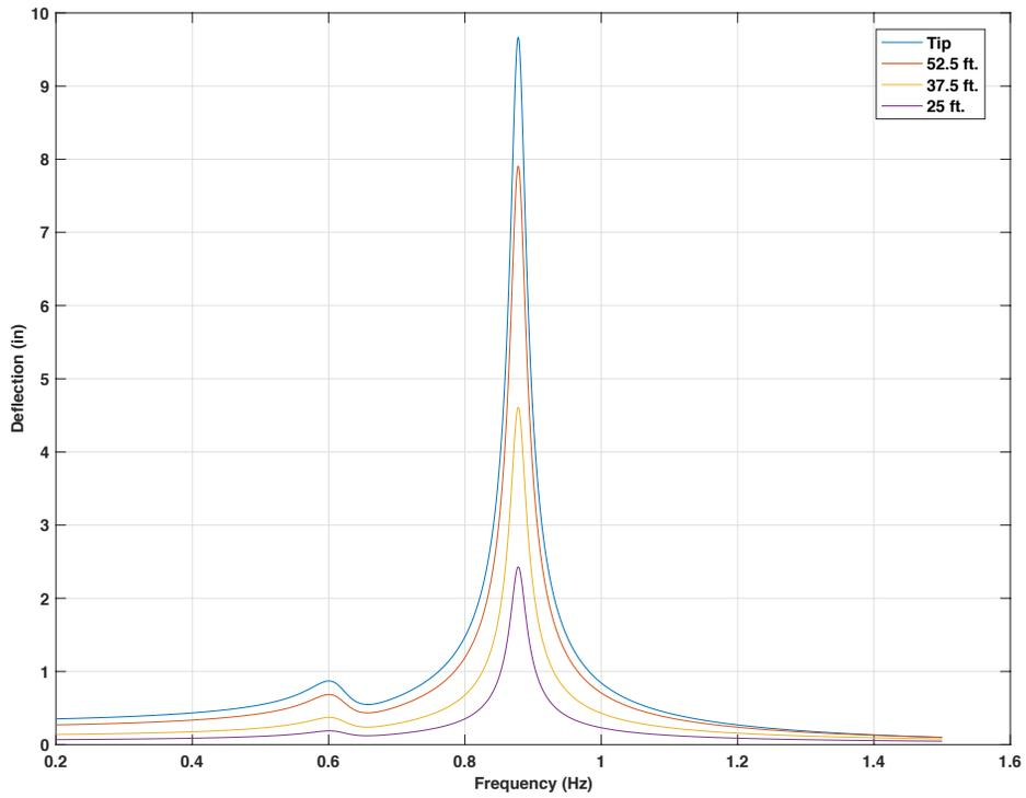
Figure 4-86 Frequency response for 60ft. mast arm with 15lb mass TMD, 5 lbf force on tip,  $f_d = 0.75 f_n$
