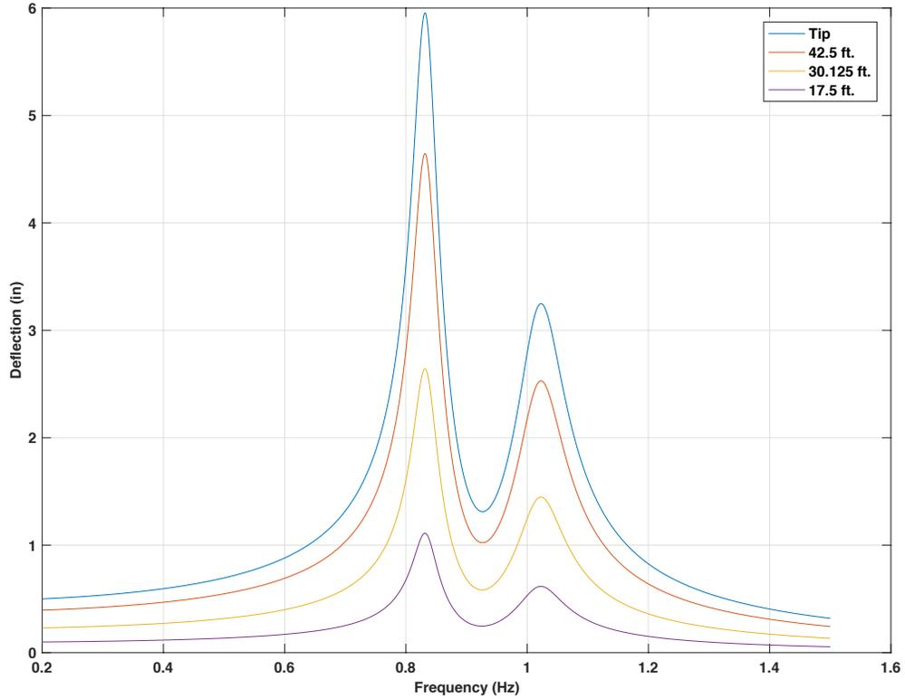
Figure 4-158 Frequency response for 50ft. mast arm with 15 lb. mass TMD at 10ft from the tip,
