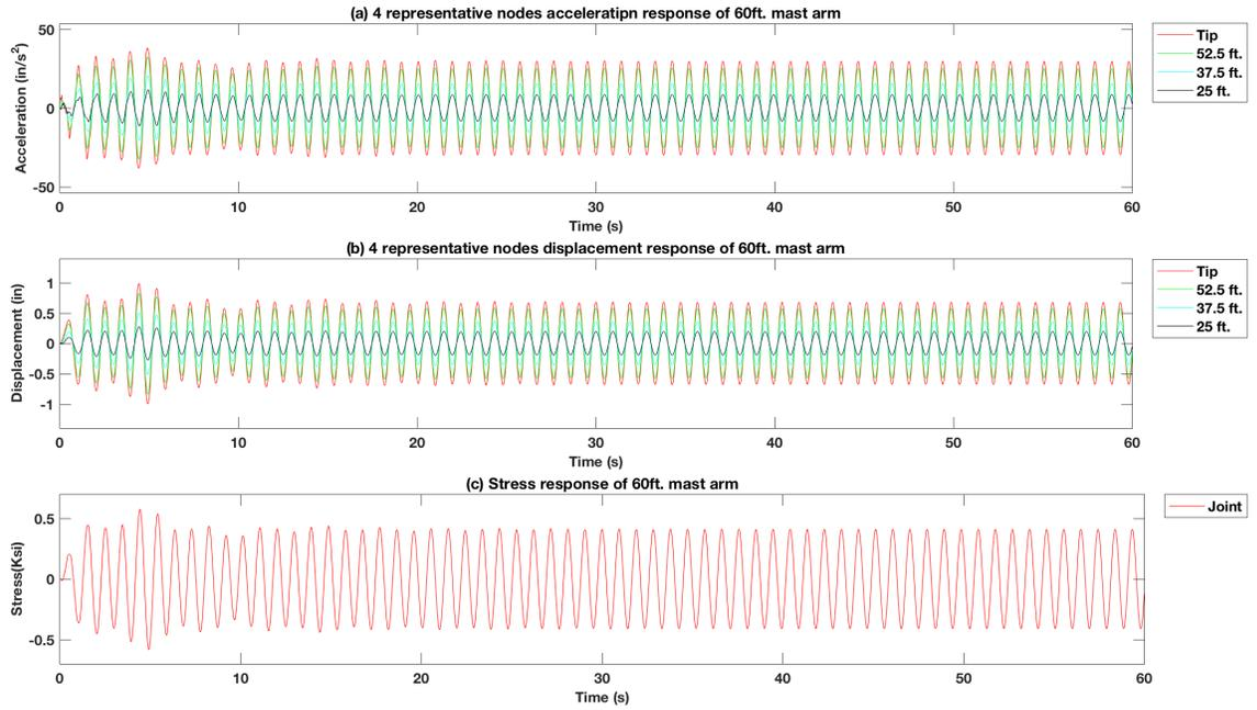
Figure 4-65 Force vibration response of excitation force at tip of the 60 ft. mast arm signal pole structure model with 15 lb. mass TMD using the  $f_x = 1.1 f_n$
