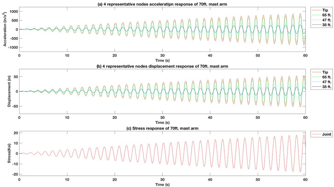
**Figure 4-3 Force vibration response of excitation force at tip in natural frequency of the 70 ft. mast arm signal pole structure model without TMD**
