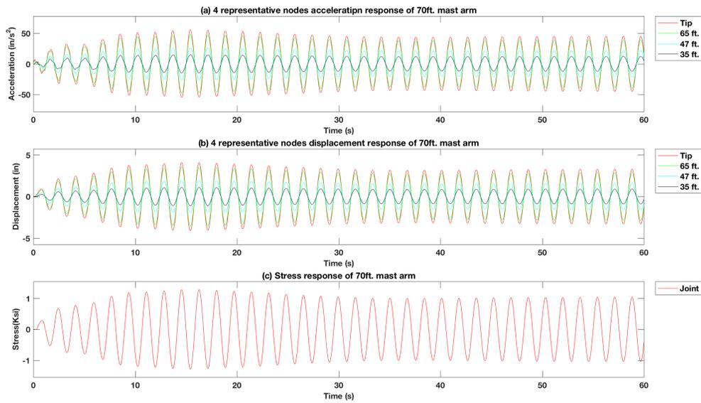
Figure 4-11 Force vibration response of excitation force at tip of the 70 ft. mast arm signal pole structure model with 15 lb. mass TMD using the  $f_x = 0.4f_n$
