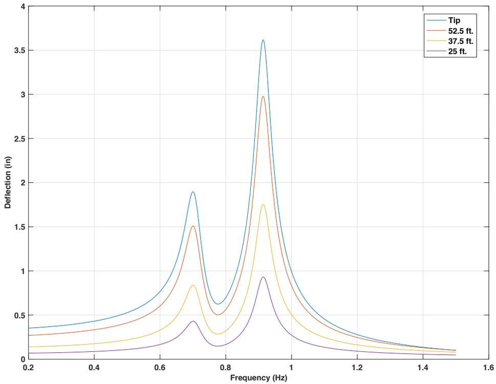
Figure 4-88 Frequency response for 60ft. mast arm with 15lb mass TMD, 5 lbf force on tip,  $f_d = 0.9 f_n$
