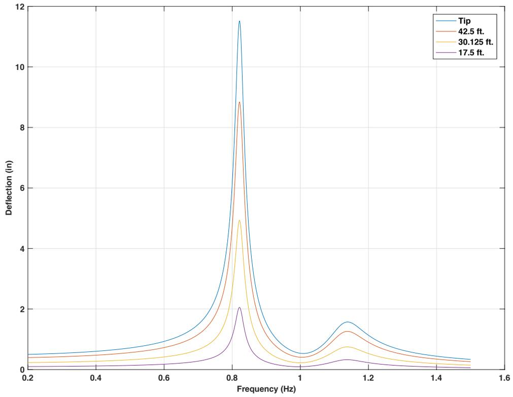
Figure 4-139 Frequency response for 50ft. mast arm with 15lb mass TMD, 5 lbf force on 3 signal heads location,  $f_d = 1.1 f_n$
