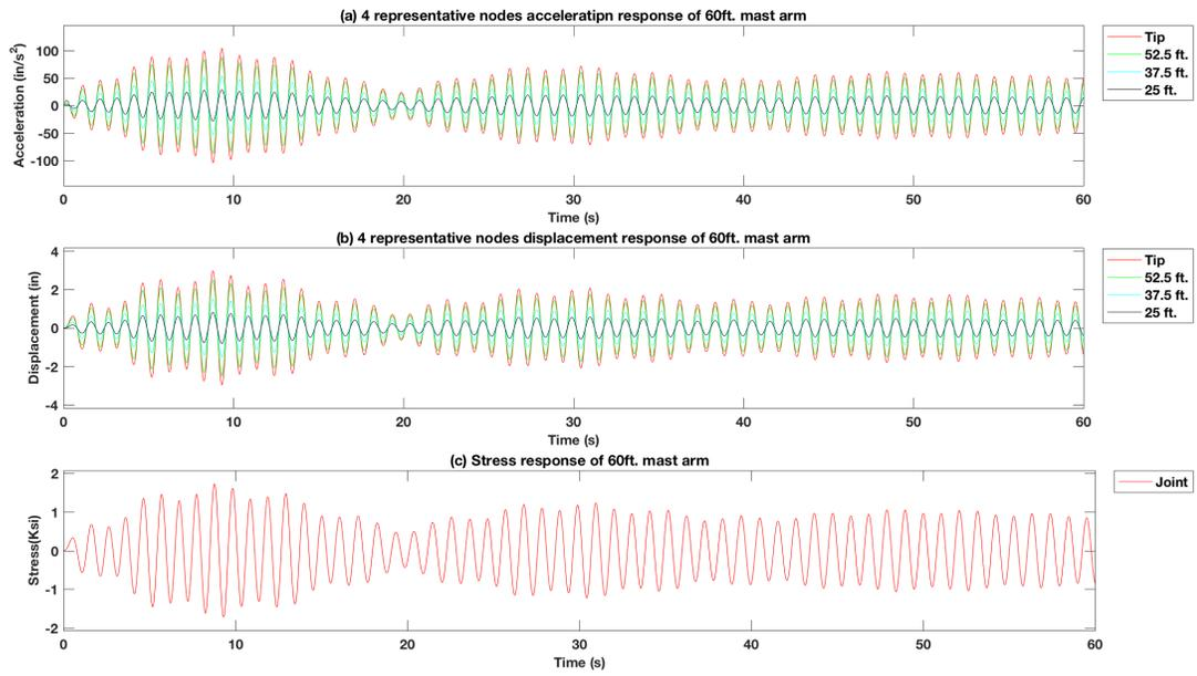
Figure 4-98 Force vibration response of excitation force at 3 signal heads position of the 60 ft. mast arm signal pole structure model with 25 lb. mass TMD using the  $\zeta = 1\%$ ,  $f_y = 0.95f_n$
