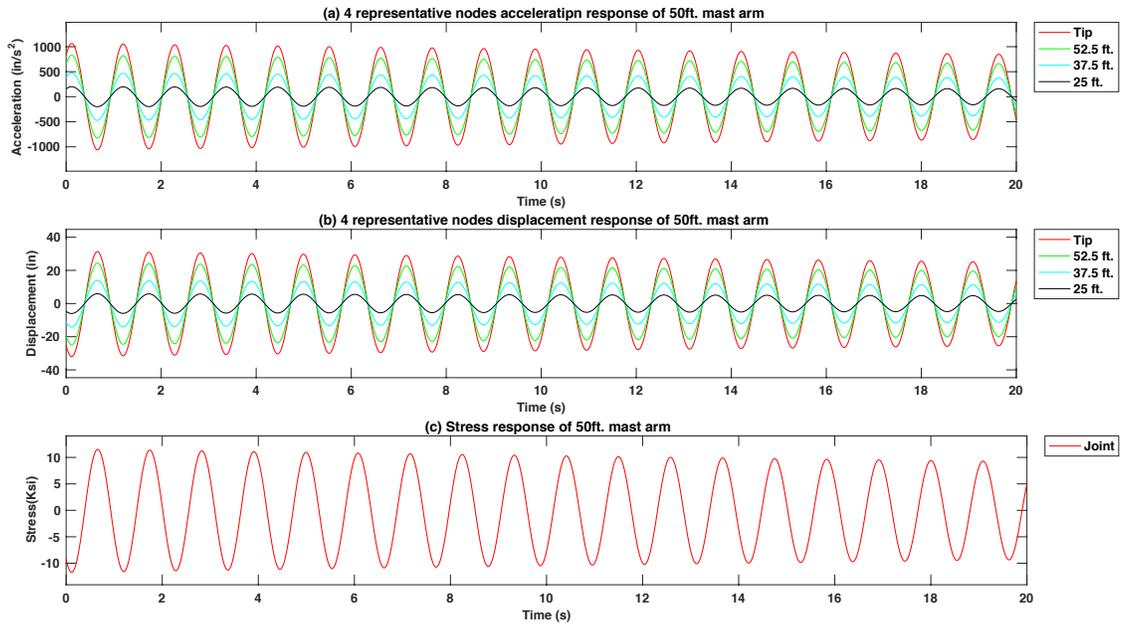
Figure 4-110 Free vibration response of the 50 ft. arm signal support structure model without TMD
