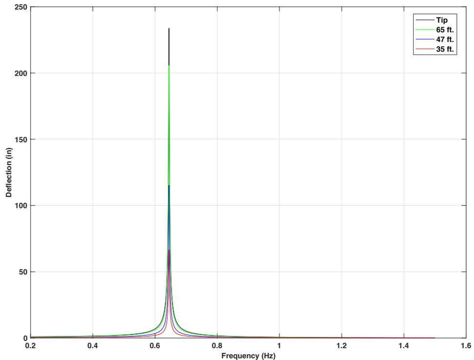
**Figure 4-7 Harmonic response for excitation force on the mast arm signal heads locations of the 70 ft. arm signal support structure model without TMD**
