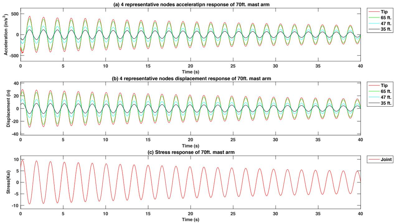
Figure 4-25 Free vibration response of excitation force at tip in the second mode frequency of the 70 ft. mast arm signal pole structure model with 15 lb. mass TMD using the  $f_d = 1.5 f_n$
