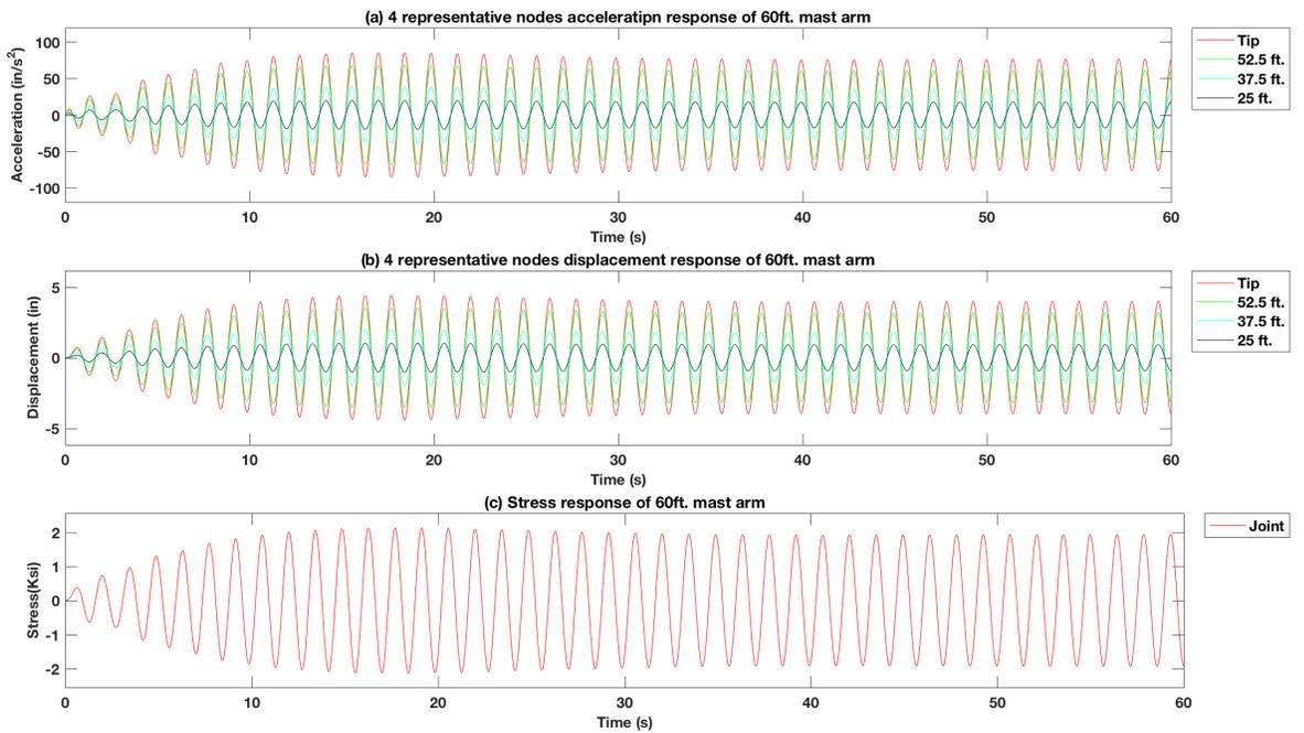
Figure 4-70 Force vibration response of excitation force at 3 signal head of the 60 ft. mast arm signal pole structure model with 25 lb. mass TMD using the  $f_x = 0.7 f_n$
