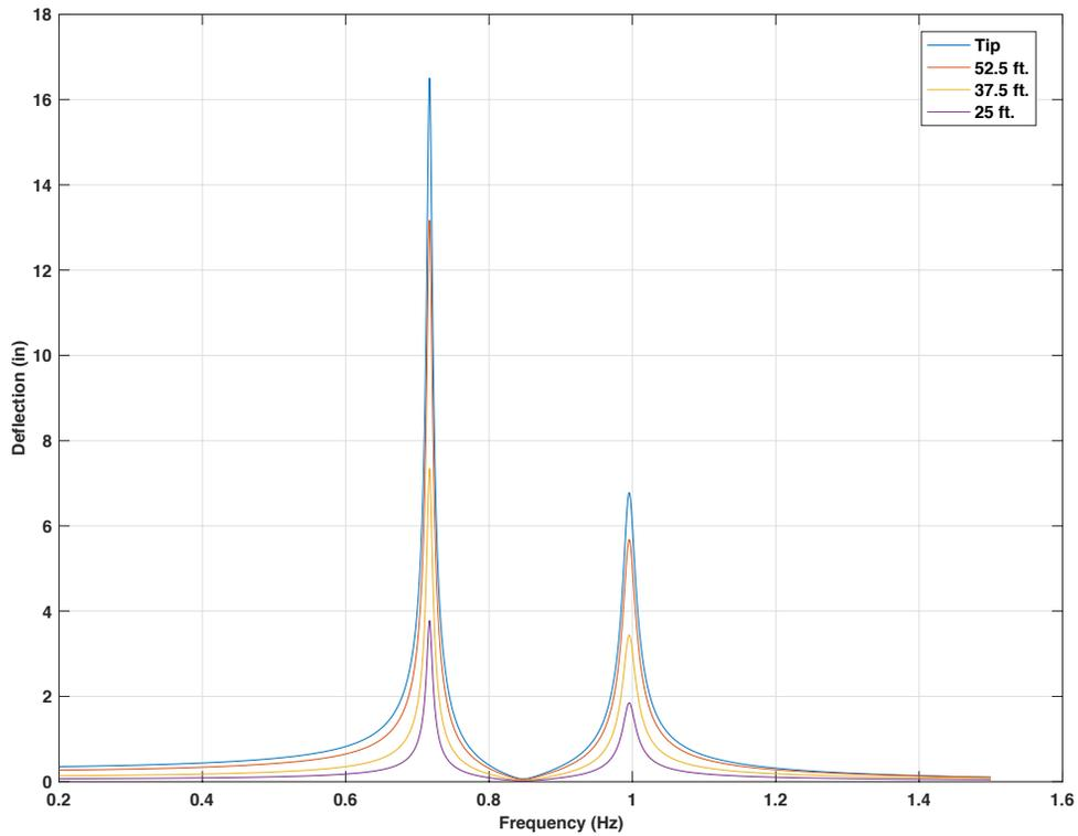
Figure 4-99 Frequency response for 60ft. mast arm with 25 lb. mass TMD using the  $\zeta = 1\%$ , 5 lbf force on tip of mast arm
