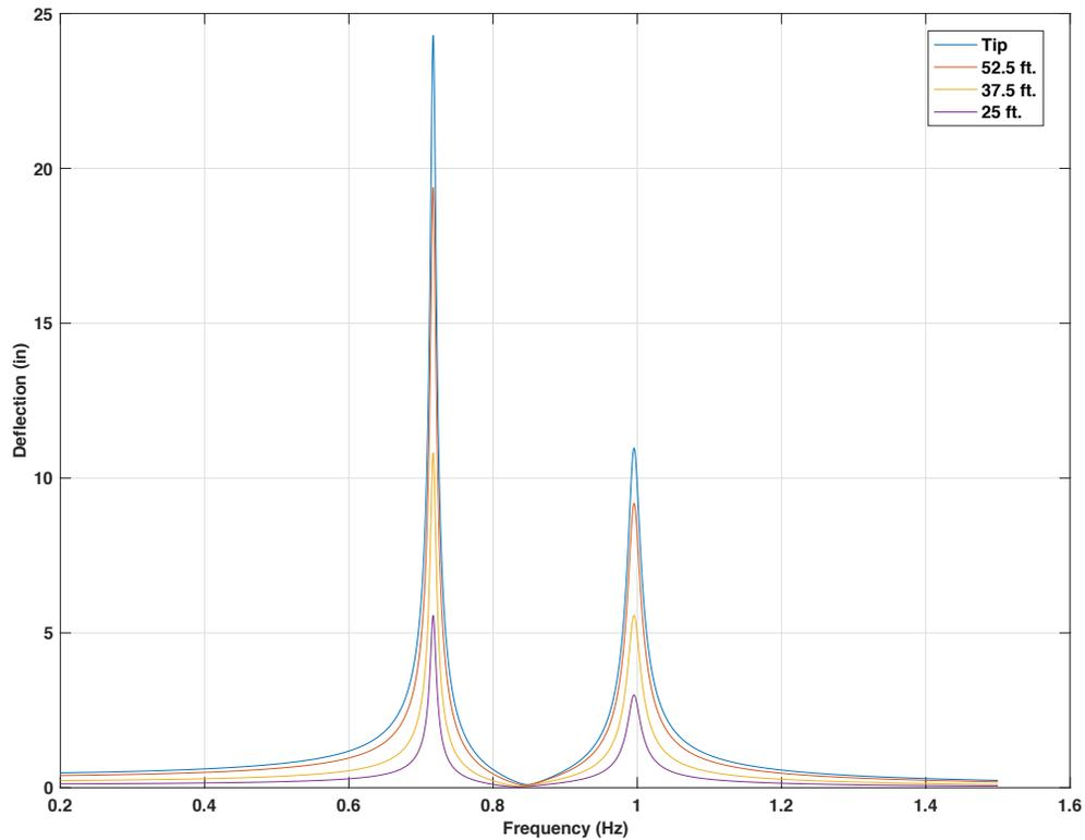
Figure 4-100 Frequency response for 60ft. mast arm with 25 lb. mass TMD using the  $\zeta = 1\%$ , 5 lbf force on 3 signal head location
