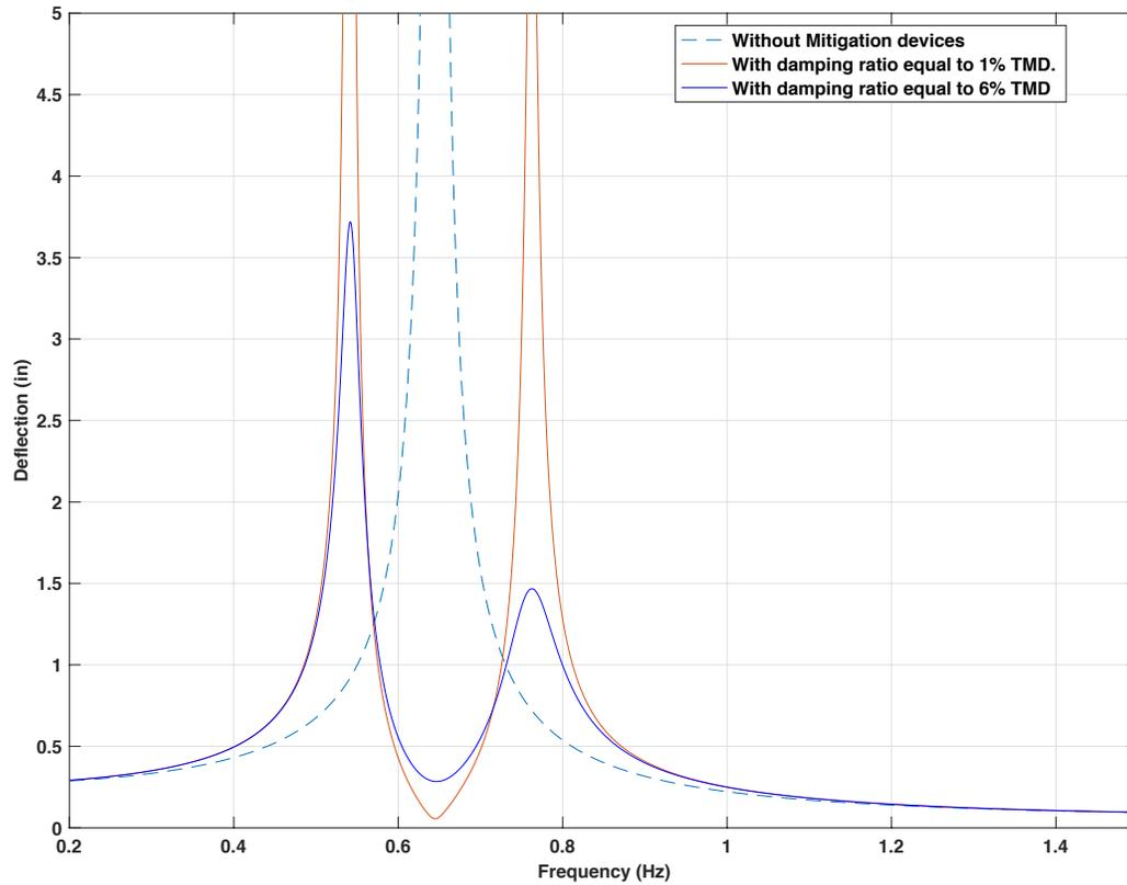
Figure 4-160 Comparison of frequency response curve of 70 feet mast arm
