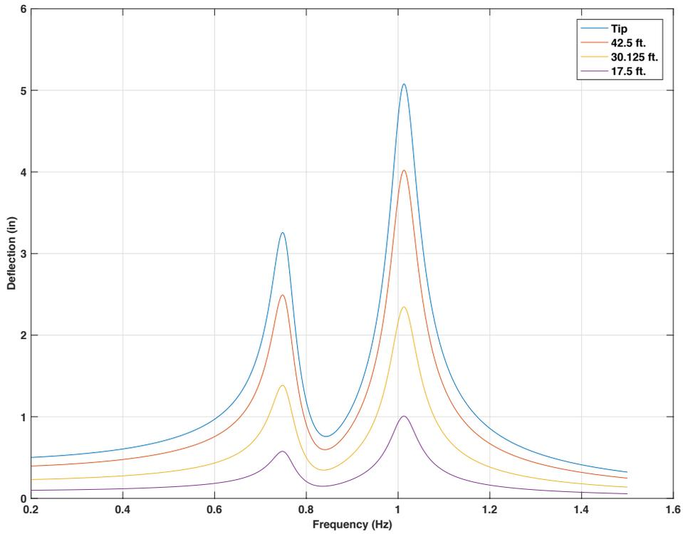
Figure 4-137 Frequency response for 50ft. mast arm with 15lb mass TMD, 5 lbf force on 3 signal heads location,  $f_d = 0.9 f_n$
