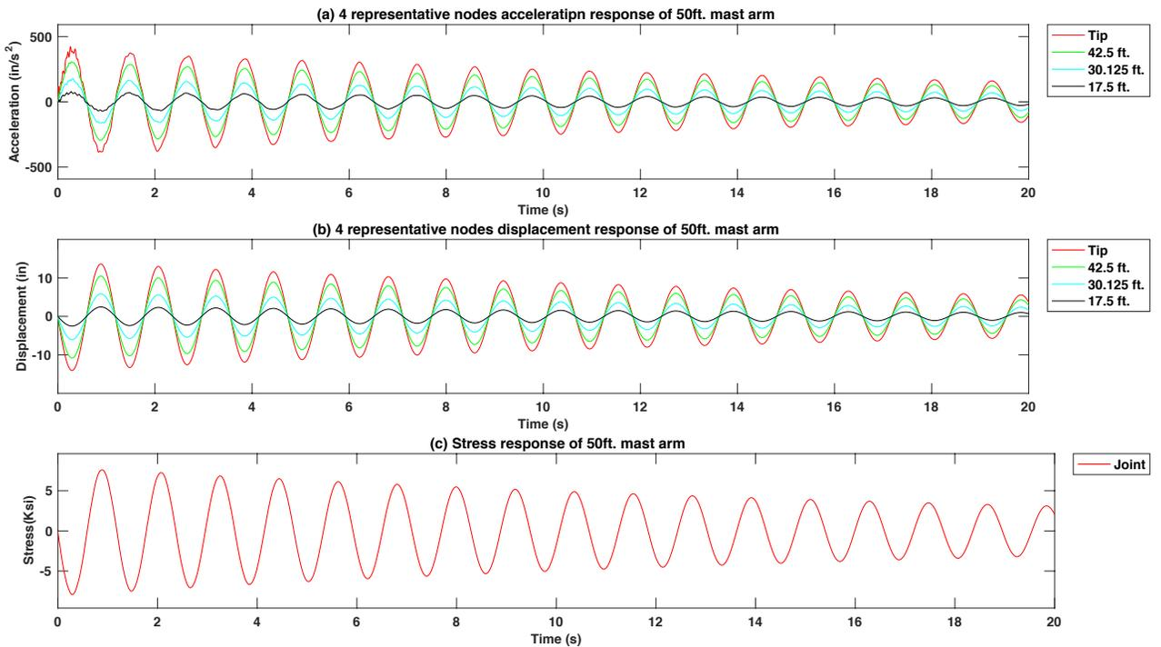
Figure 4-124 Free vibration response of excitation force at tip of the 50 ft. mast arm signal pole structure model with 15 lb. mass TMD using the  $f_d = 1.25 f_n$
