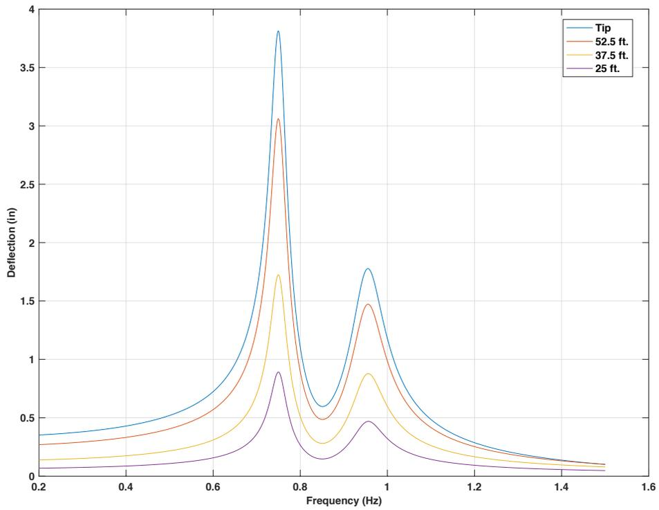
Figure 4-153 Frequency response for 50ft. mast arm with 15 lb. mass TMD at 1.5 ft from the tip, 5 lbf force on tip of mast arm,  $f_d = 1.0f_n$
