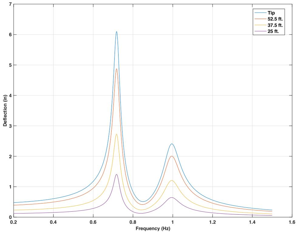
**Figure 4-72 Frequency response for 60ft. mast arm with 25lb mass TMD, force on signal heads' location**
