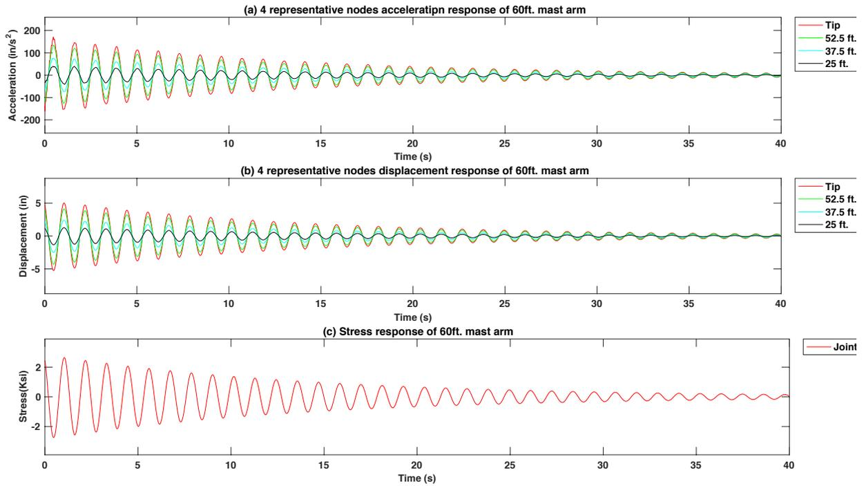
Figure 4-74 Free vibration response of excitation force at tip in natural frequency of the 60 ft. mast arm signal pole structure model with 15 lb. mass TMD using the  $f_d = 0.75 f_n$
