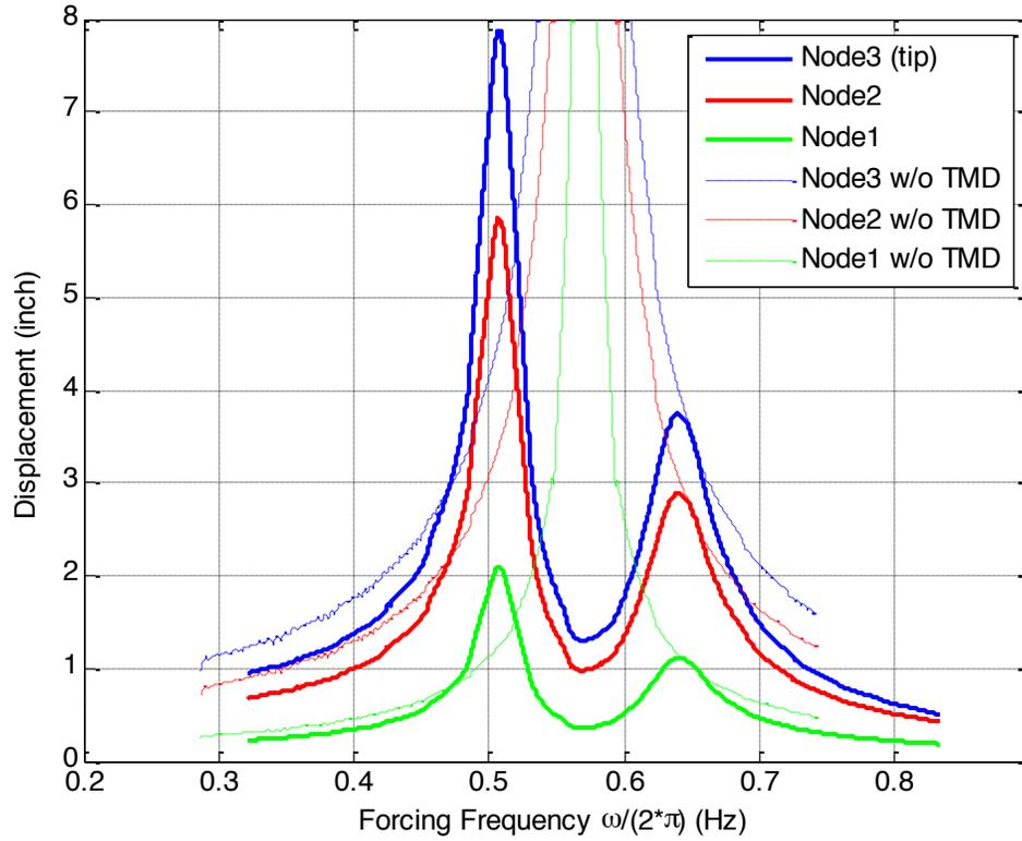
Figure 3-11 Harmonic Analysis for the Analytical model using 15lb. mass TMD
