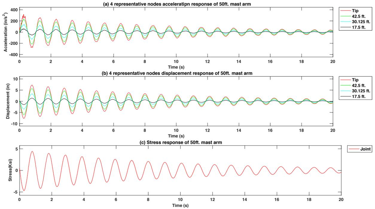
Figure 4-123 Free vibration response of excitation force at tip in natural frequency of the 50 ft. mast arm signal pole structure model with 15 lb. mass TMD using the  $f_d = 0.75 f_n$
