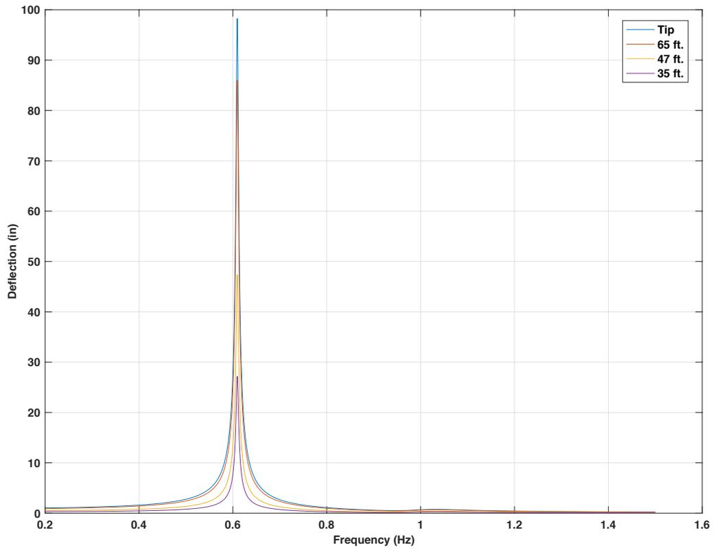
Figure 4-42 Frequency response for 70ft. mast arm with 15lb mass TMD, 5 lbf force on 3 signal heads location,  $f_d = 1.5 f_n$
