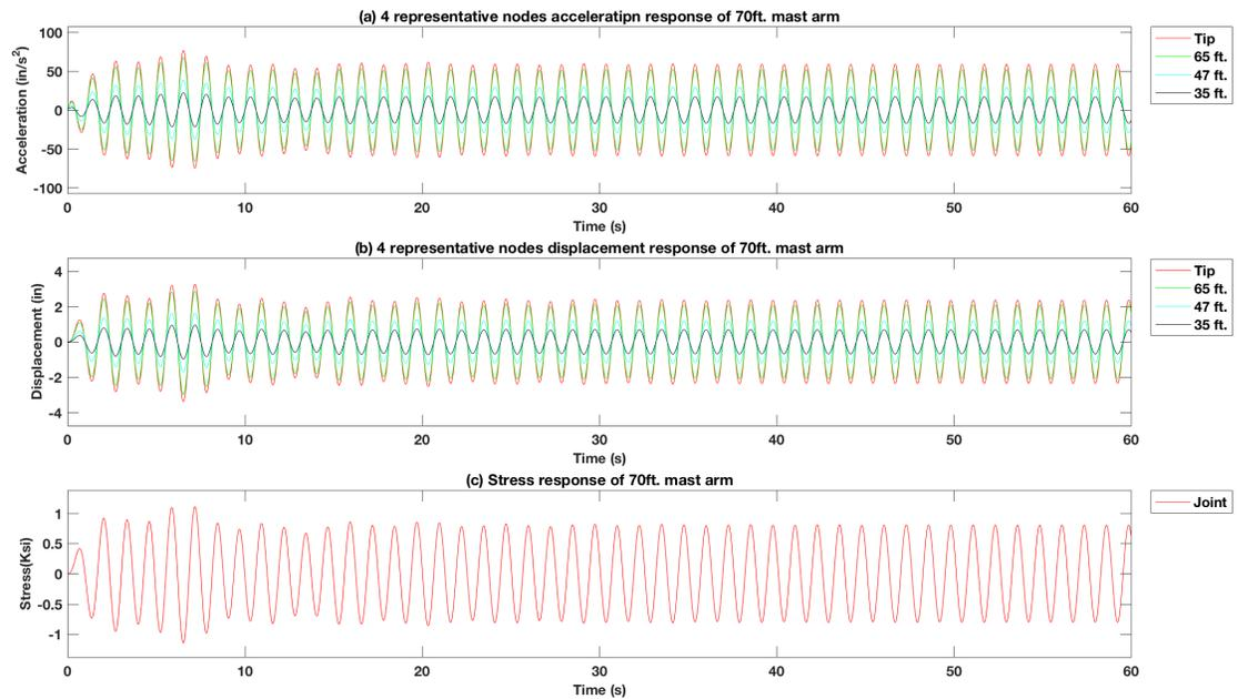
Figure 4-50 Force vibration response of excitation force at 3 signal heads position on the 70 ft. mast arm signal pole structure model TMD at 5 ft from the tip  $f_x = 1.1f_n$
