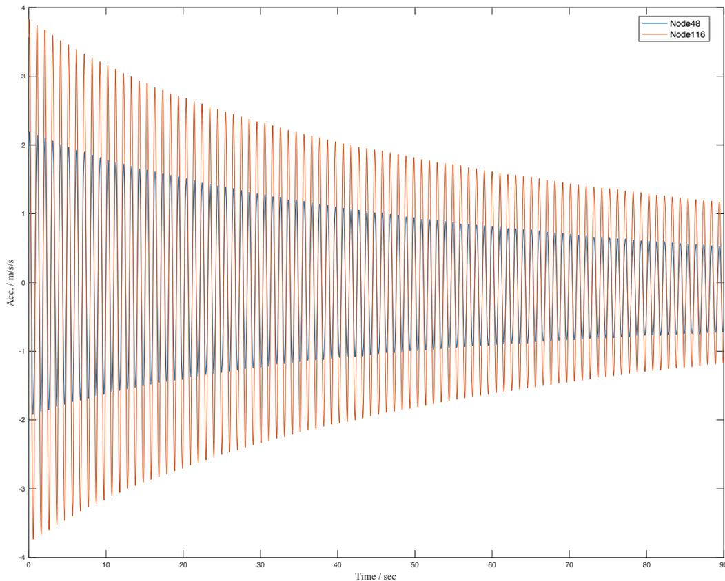
**Figure 5-3 response curve for free vibration of 50 ft mast arm**
