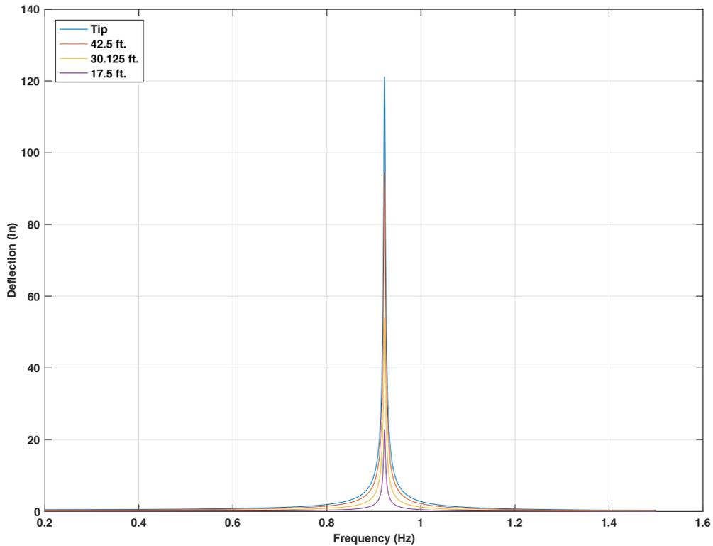
**Figure 4-114 Harmonic response for excitation force on the mast arm signal heads locations of the 50 ft. arm signal support structure model without TMD**
