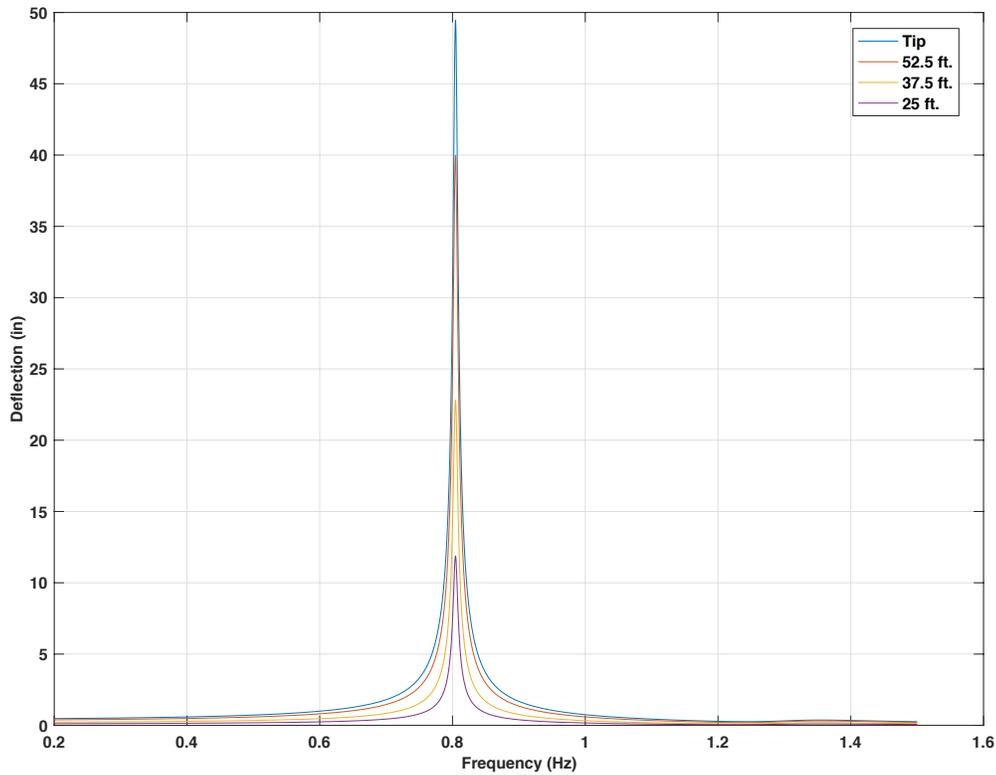
Figure 4-95 Frequency response for 60ft. mast arm with 15lb mass TMD, 5 lbf force on 3 signal heads location,  $f_d = 1.5 f_n$
