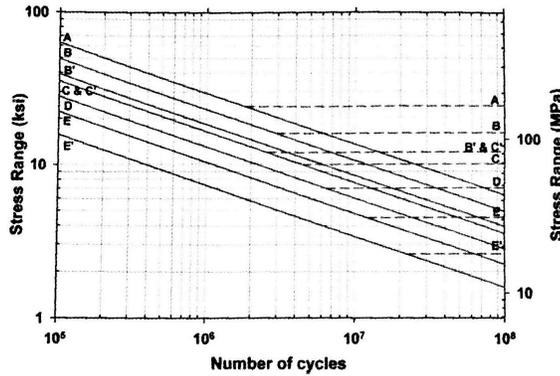
Figure 2-1 Stress Range Vs. Number of cycles (AASHTO Specification Figure C11.9.3-1)
