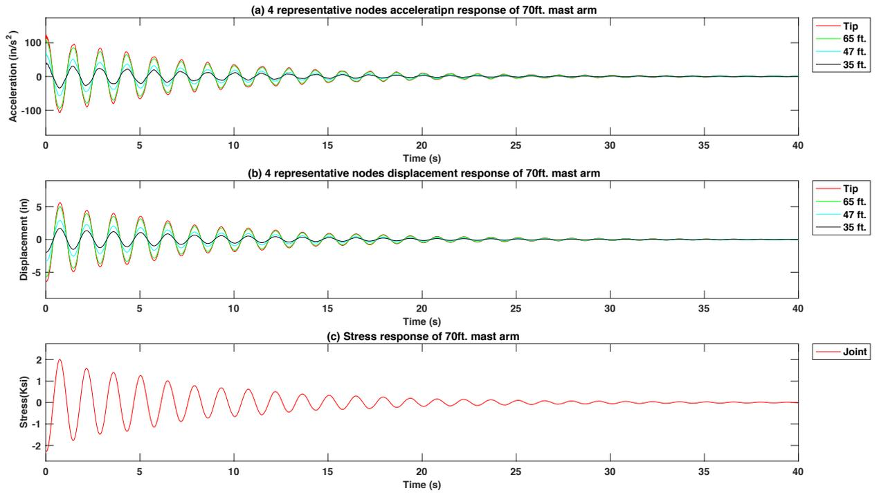
**Figure 4-23 Free vibration response of excitation force at tip in natural frequency of the 70 ft. mast arm signal pole structure model with 15 lb. mass TMD using the  $f_d = 0.9 f_n$**
