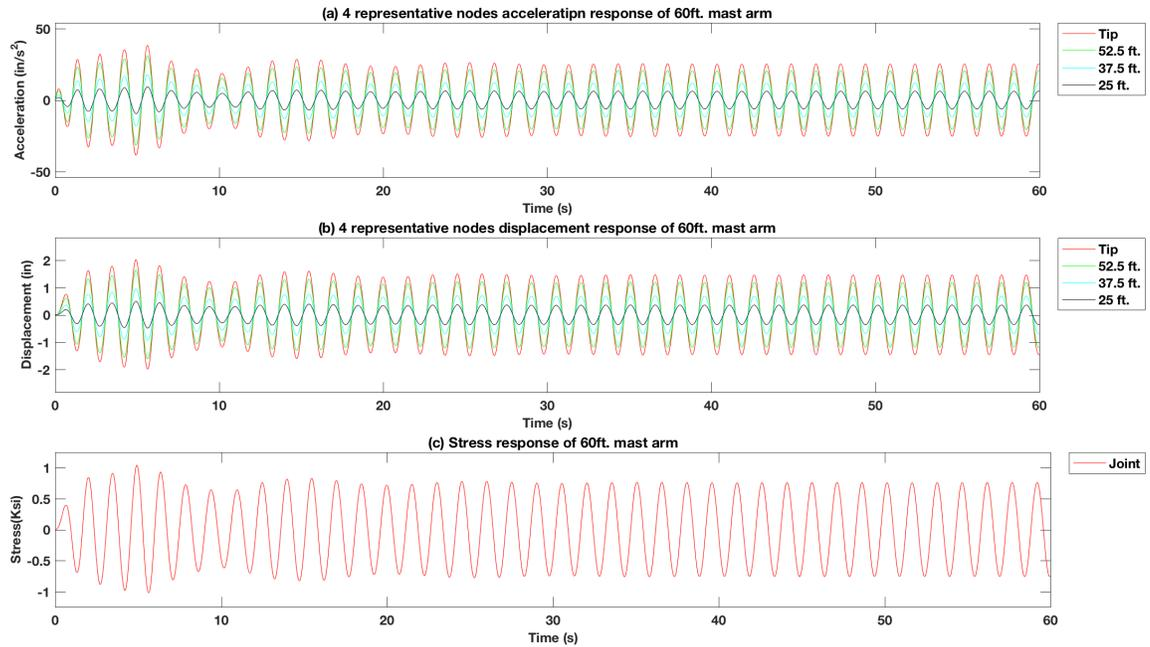
Figure 4-102 Force vibration response of excitation force at 3 signal heads position of the 60 ft. mast arm signal pole structure model TMD at 5 ft from the tip  $f_x = 0.7f_n$
