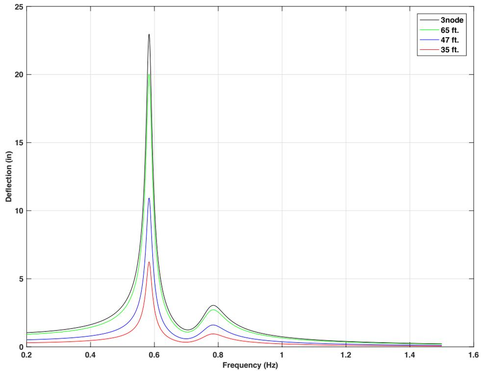
Figure 4-38 Frequency response for 70ft. mast arm with 15lb mass TMD, 5 lbf force on 3 signal heads location,  $f_d = 1.1 f_n$  (notation 3node means tip deflection under this situation)
