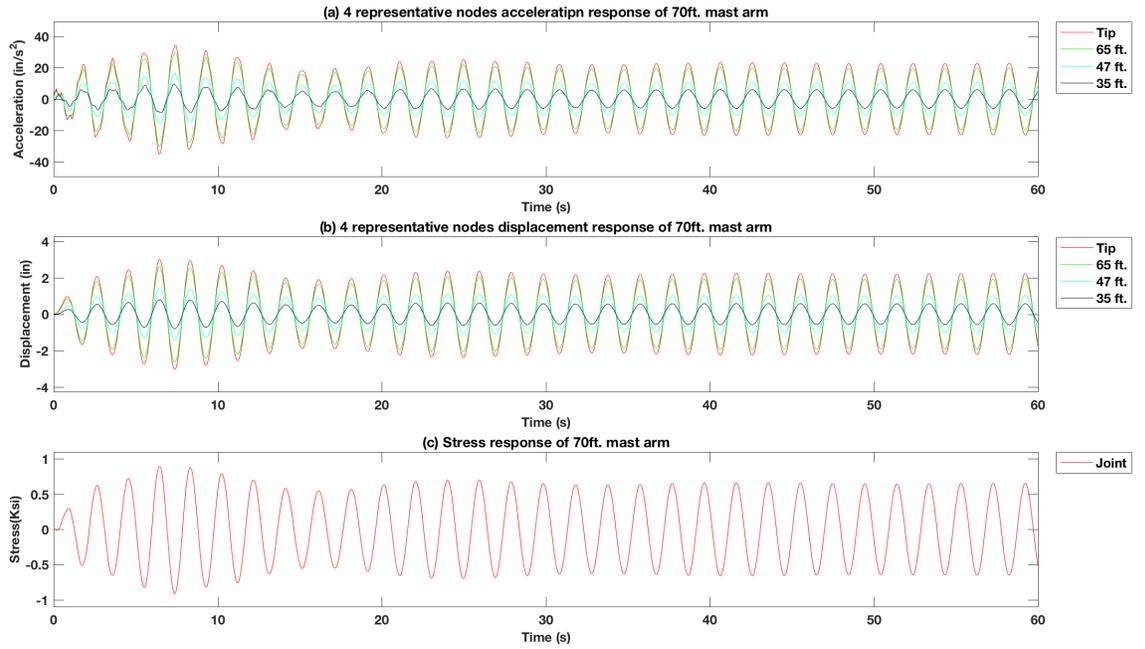
Figure 4-49 Force vibration response of excitation force at tip on the 70 ft. mast arm signal pole structure model TMD at 2.5 ft from the tip  $f_x = 0.7f_n$
