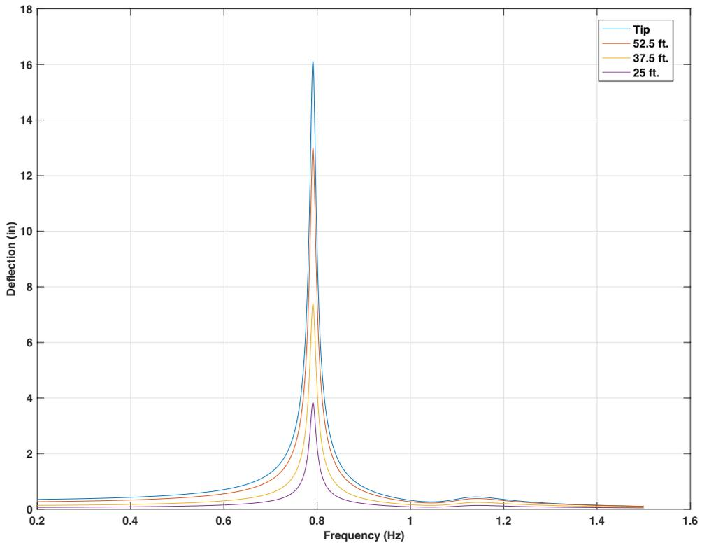
Figure 4-92 Frequency response for 60ft. mast arm with 15lb mass TMD, 5 lbf force on tip,  $f_d = 1.25 f_n$
