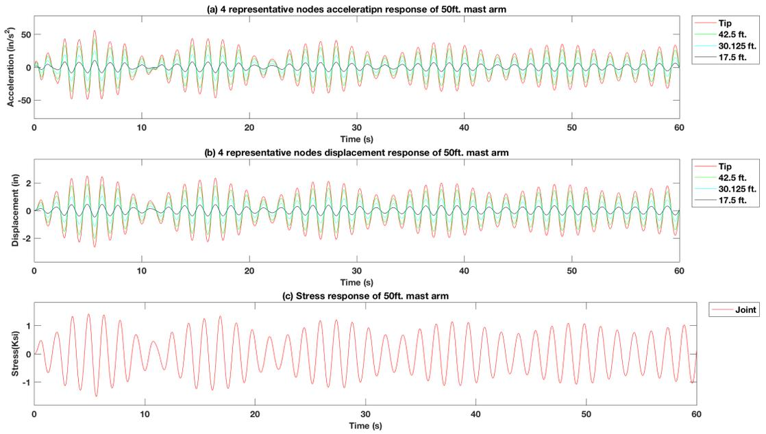
Figure 4-146 Force vibration response of excitation force at 3 signal heads position of the 50 ft. mast arm signal pole structure model with 25 lb. mass TMD using the  $\zeta = 1\%$ ,  $f_x = 0.6f_n$
