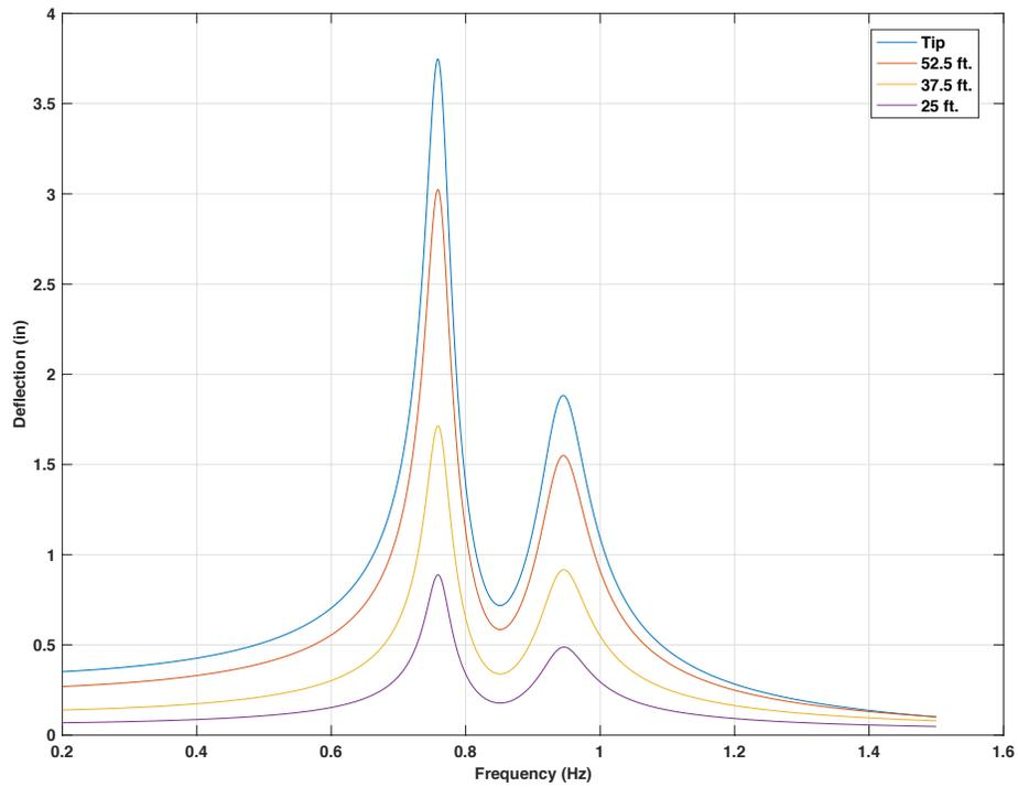
Figure 4-106 Frequency response for 60ft. mast arm with 15 lb. mass TMD at 5 ft from the tip  $f_d = 1.0f_n$ , 5 lbf force on tip of mast arm
