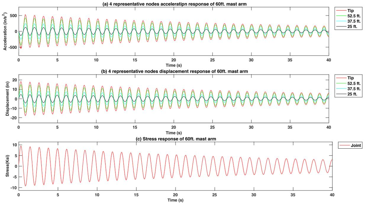
Figure 4-73 Free vibration response of excitation force at tip of the 60 ft. mast arm signal pole structure model with 15 lb. mass TMD using the  $f_d = 0.5 f_n$
