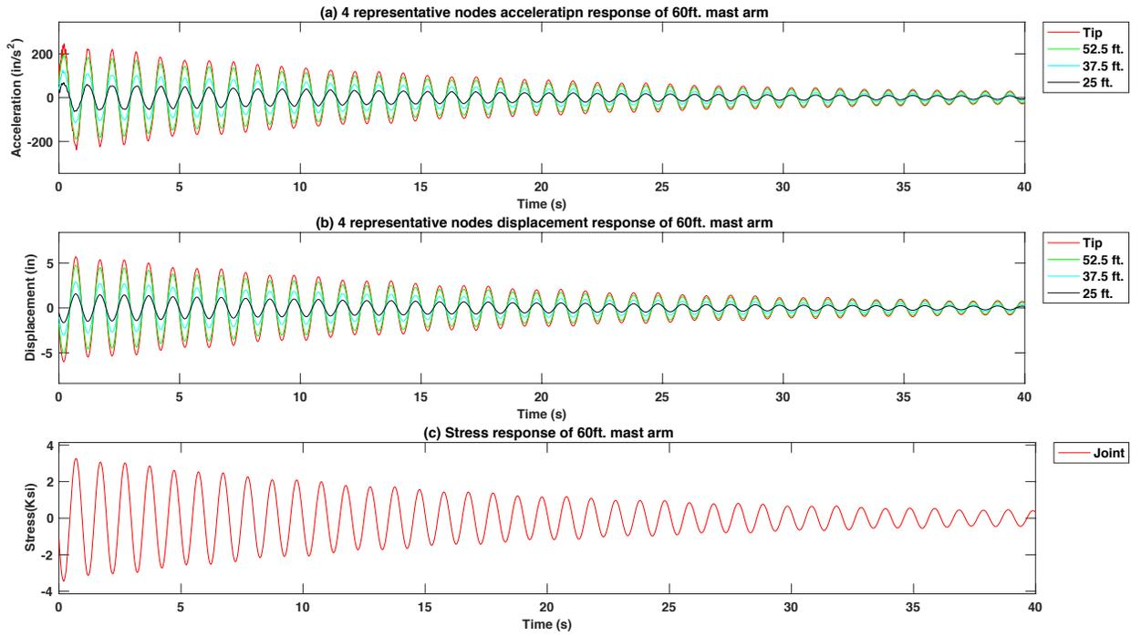
Figure 4-96 Free vibration response of excitation force at tip of the 60 ft. mast arm signal pole structure model with 25 lb. mass TMD using the  $\zeta = 1\%$ .
