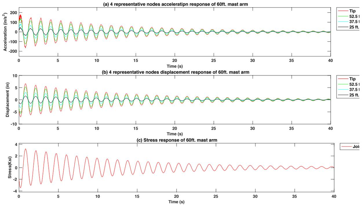
Figure 4-75 Free vibration response of excitation force at tip of the 60 ft. mast arm signal pole structure model with 15 lb. mass TMD using the  $f_d = 1.1 f_n$
