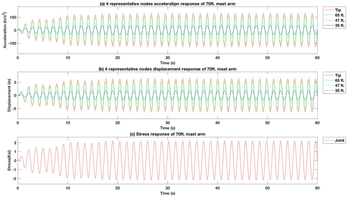
Figure 4-51 Force vibration response of excitation force at 3 signal heads position on 70 ft. mast arm signal pole structure model TMD at 10 ft from the tip  $f_d = 1.0 f_n$
