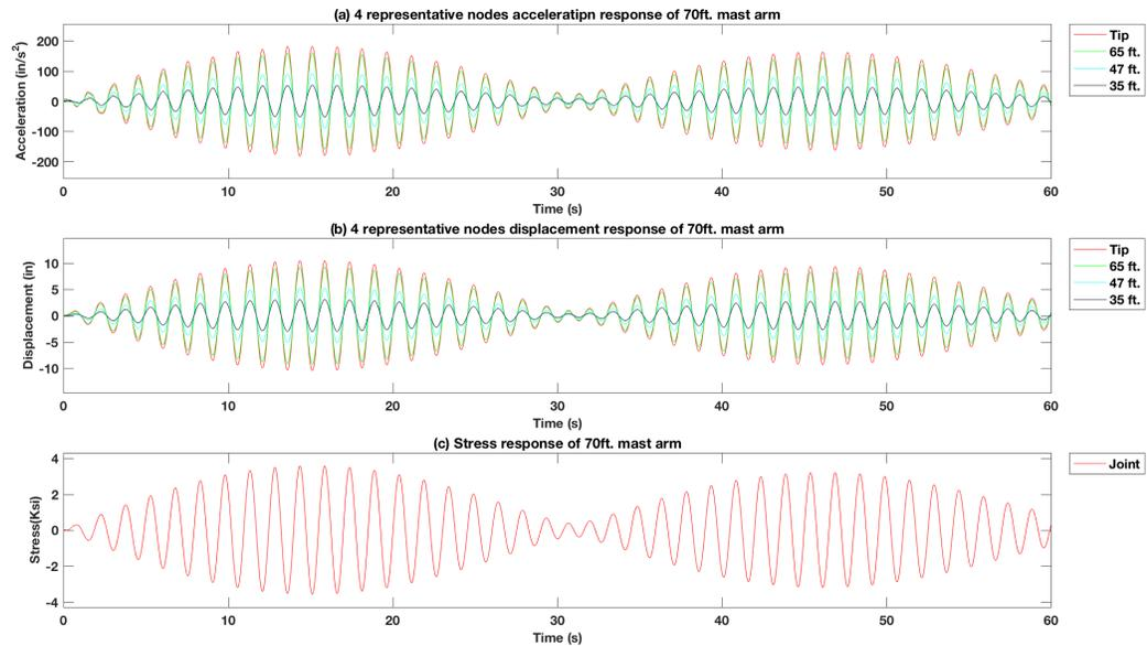
**Figure 4-4 Force vibration response of excitation force at tip in  $f_2 = 1.05 \times \text{Natural frequency}$  of the 70 ft. arm signal support structure model without TMD**
