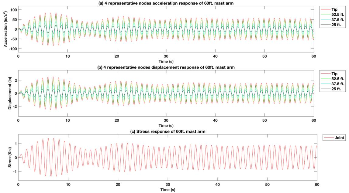
**Figure 4-79 Force vibration response of excitation force at tip of the 60 ft. mast arm signal pole structure model with 15 lb. mass TMD using the  $f_d = 0.75 f_n$ ,  $f_y = 1.1 f_n$**
