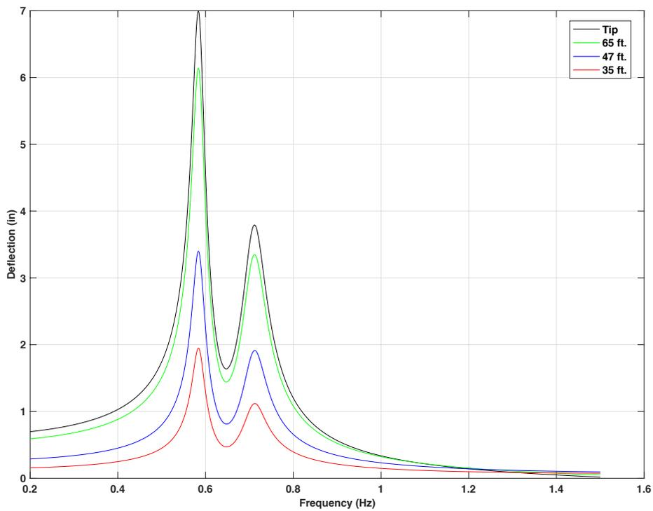
Figure 4-56 Frequency response for 70ft. mast arm with 15 lb. mass TMD at 2.5 ft from the tip
