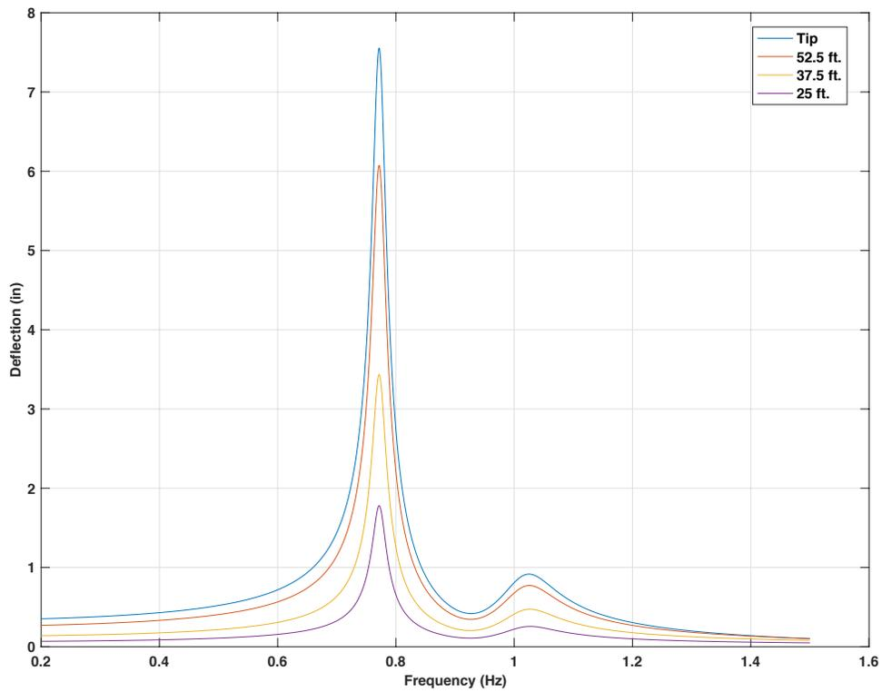
Figure 4-90 Frequency response for 60ft. mast arm with 15lb mass TMD, 5 lbf force on tip,  $f_d = 1.1 f_n$
