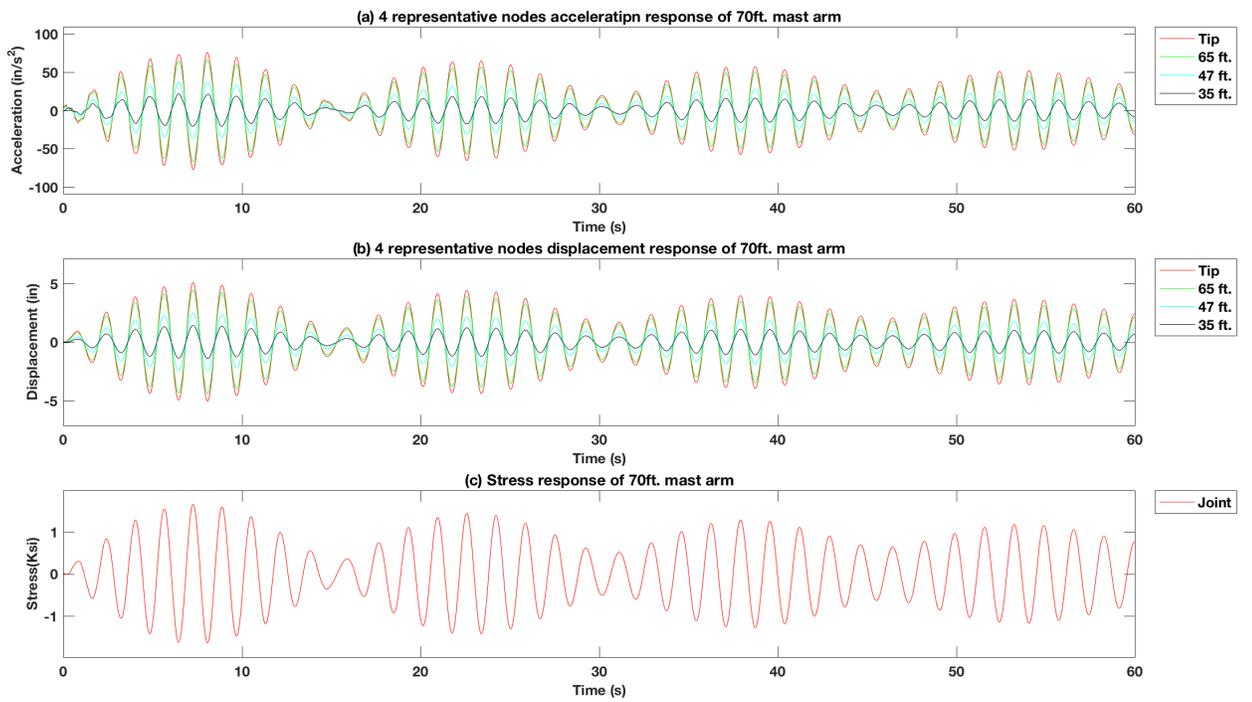
Figure 4-28 Force vibration response of excitation force at tip of the 70 ft. mast arm signal pole structure model with 15 lb. mass TMD using the  $f_d = 0.5 f_n$ ,  $f_x = 1.1 f_n$
