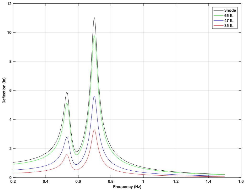
Figure 4-36 Frequency response for 70ft. mast arm with 15lb mass TMD, 5 lbf force on 3 signal heads location,  $f_d = 0.9 f_n$  (notation 3node means tip deflection under this situation)
