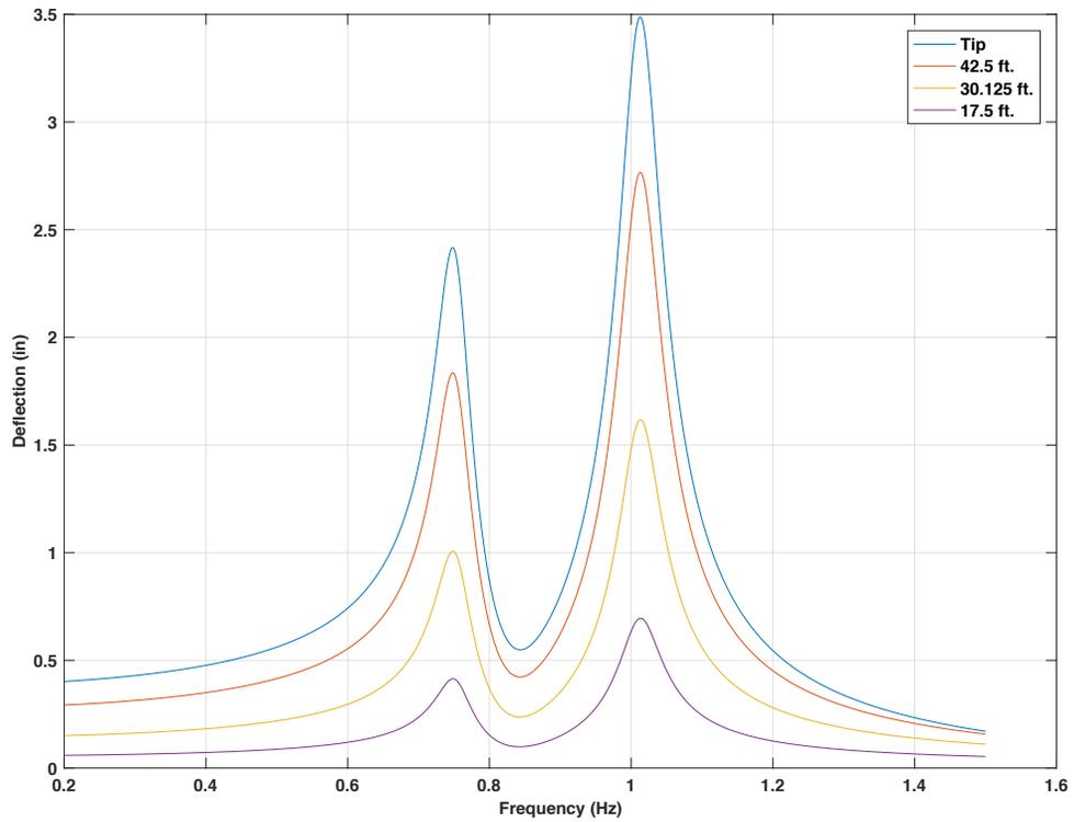
Figure 4-136 Frequency response for 50ft. mast arm with 15lb mass TMD, 5 lbf force on tip,  $f_d = 0.9 f_n$
