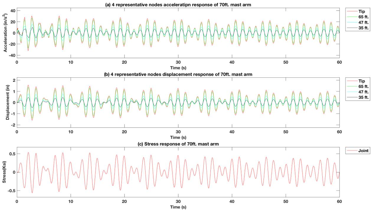
Figure 4-29 Force vibration response of excitation force at tip of the 70 ft. mast arm signal pole structure model with 15 lb. mass TMD using the  $f_d = 1.5 f_n$ ,  $f_y = 1.3 f_n$
