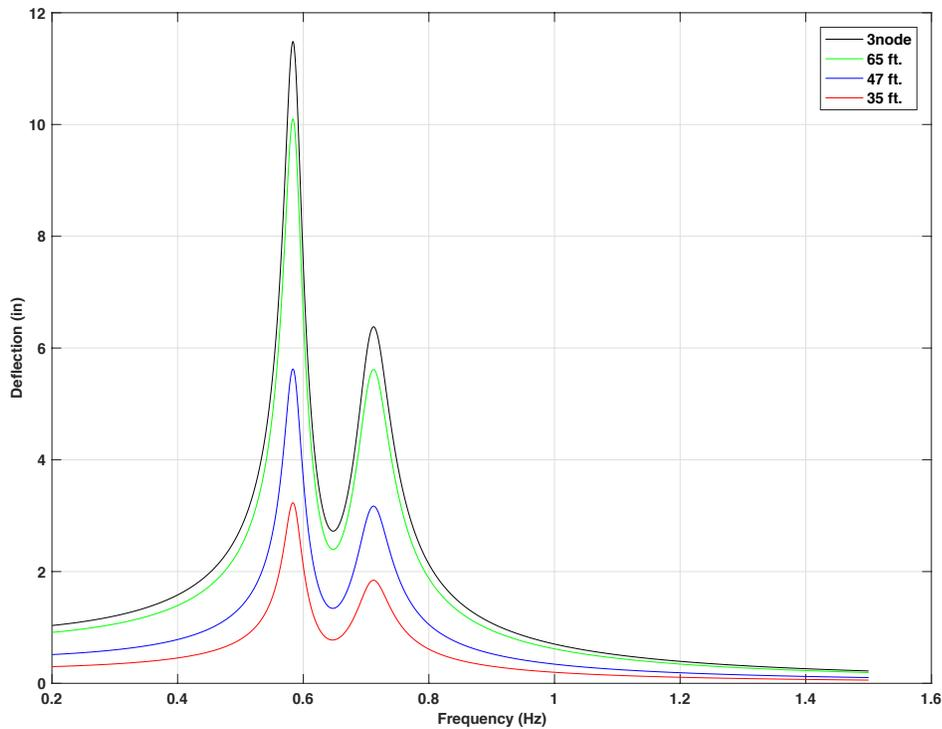
**Figure 4-57 Frequency response for 70ft. mast arm with 15 lb. mass TMD at 2.5 ft from the tip,  $f_d = 1.0f_n$ , 5 lbf force on 3 signal head location**
