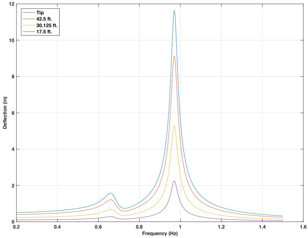
Figure 4-135 Frequency response for 50ft. mast arm with 15lb mass TMD, 5 lbf force on 3 signal heads location,  $f_d = 0.75 f_n$
