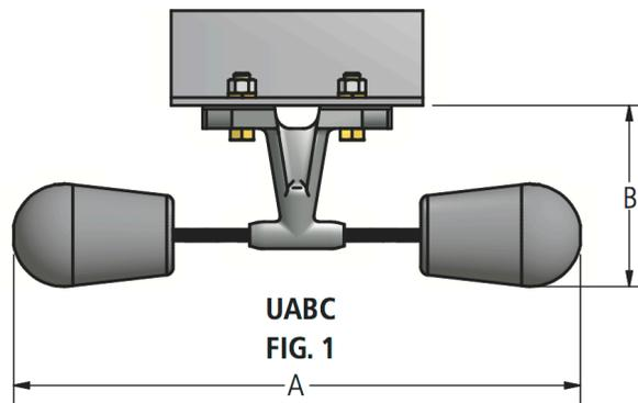
**Figure 3-9 Alcoa damper. (From AFL Substation Bus Dampers catalog)**
