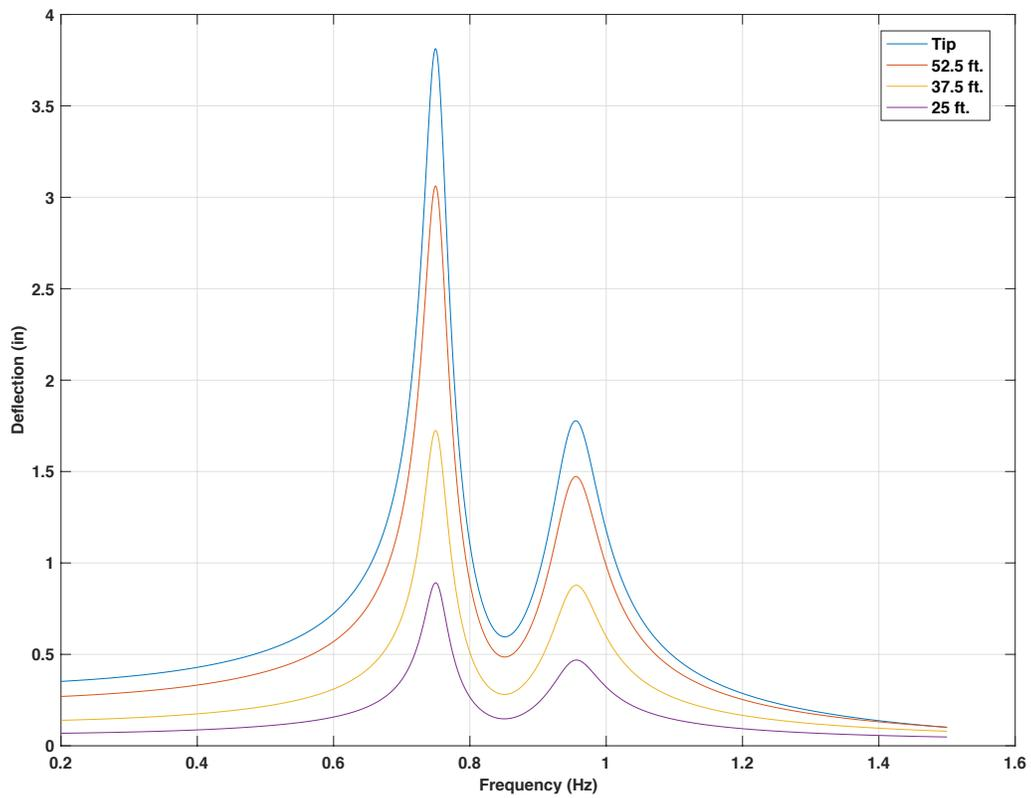
Figure 4-104 Frequency response for 60ft. mast arm with 15 lb. mass TMD at 1.5 ft from the tip, 5 lbf force on tip of mast arm,  $f_d = 1.0f_n$
