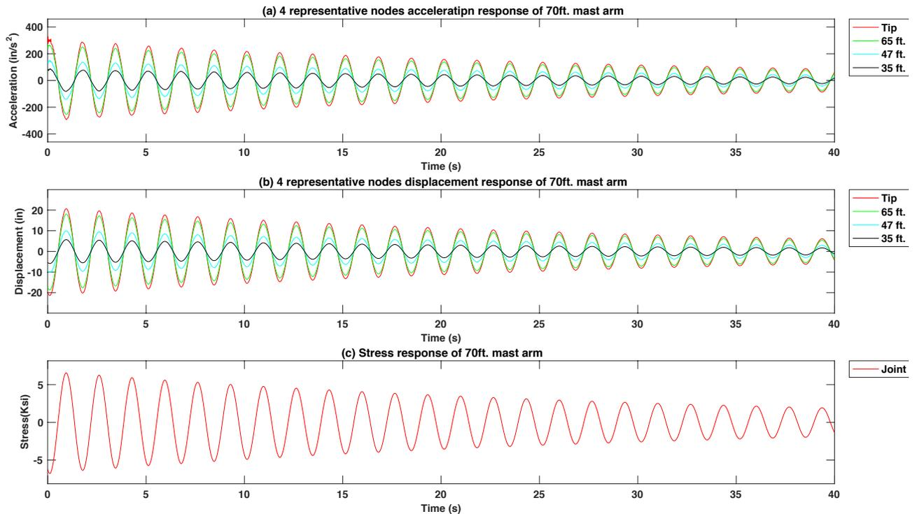
**Figure 4-24 Free vibration response of excitation force at tip in the second mode frequency of the 70 ft. mast arm signal pole structure model with 15 lb. mass TMD using the  $f_d = 1.25 f_n$**
