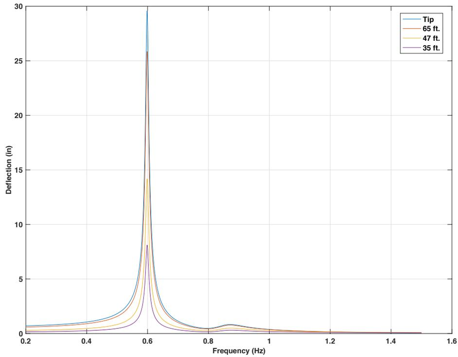
Figure 4-39 Frequency response for 70ft. mast arm with 15lb mass TMD, 5 lbf force on tip,  $f_d = 1.25 f_n$
