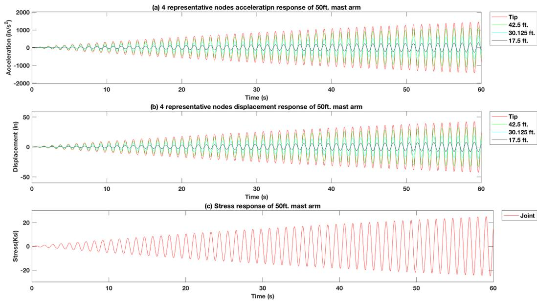
Figure 4-111 Force vibration response of excitation force at tip in  $f_x = 1.0 f_n$  of the 50 ft. mast arm signal pole structure model without TMD
