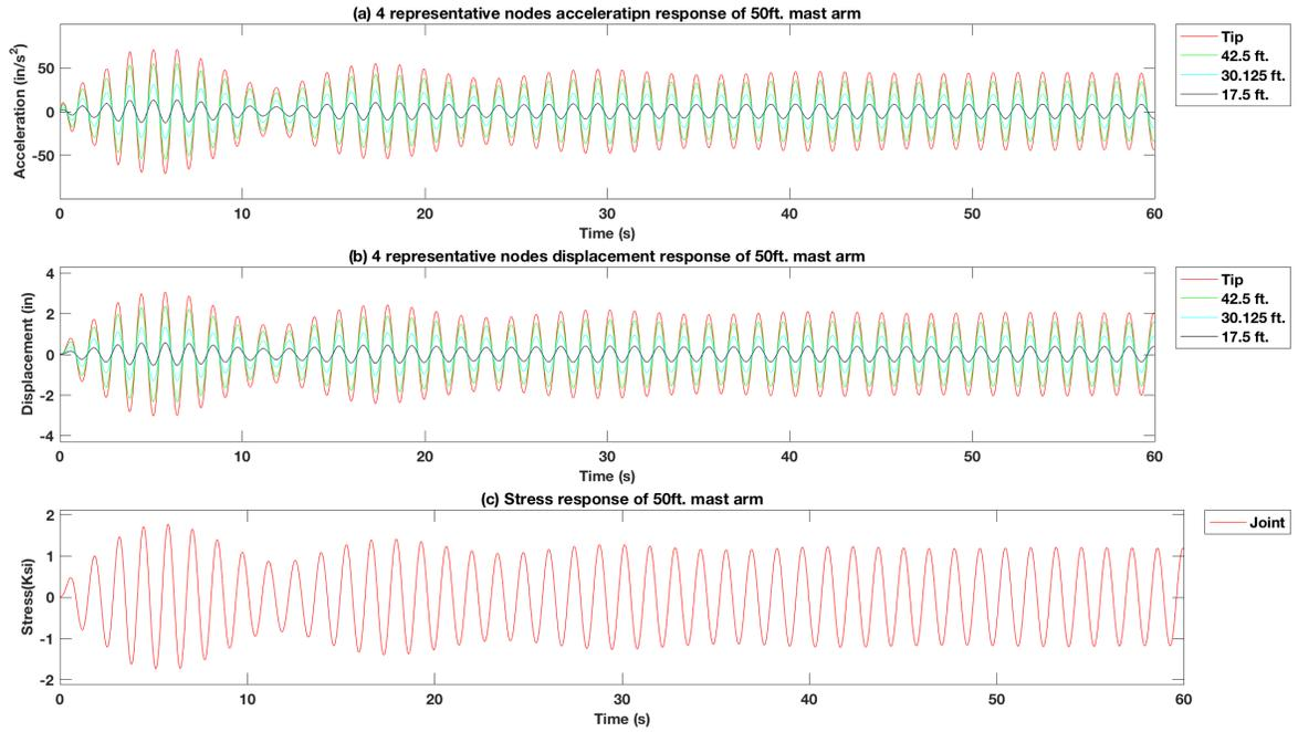
Figure 4-131 Force vibration response of excitation force at tip of the 50 ft. mast arm signal pole structure model with 15 lb. mass TMD using the  $f_d = 1.1 f_n$ ,  $f_x = 0.9 f_n$
