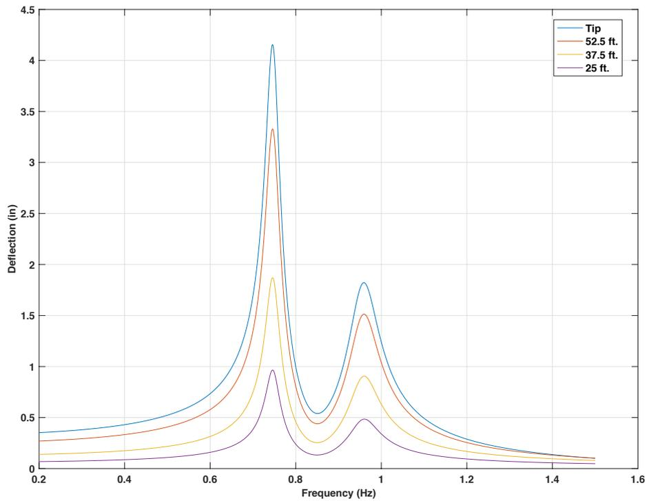
Figure 4-67 Frequency response for 60ft. mast arm with 15lb mass TMD, force on the tip
