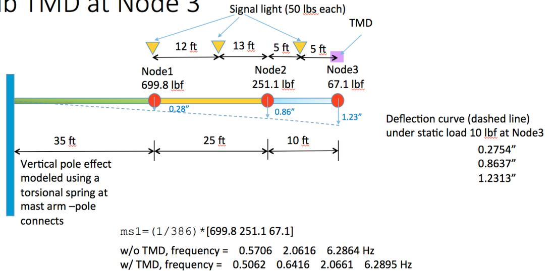
**Figure 3-10 Model and static summary of MATLAB model for the TMD with the mast arm**
