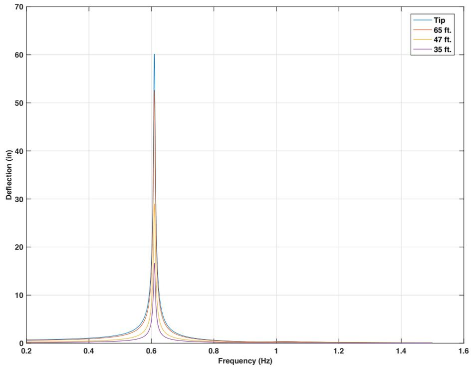
Figure 4-41 Frequency response for 70ft. mast arm with 15lb mass TMD, 5 lbf force on tip,  $f_d = 1.5 f_n$
