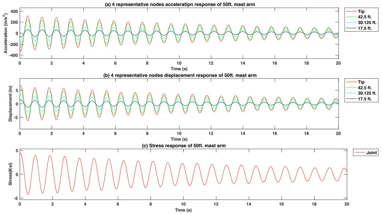
Figure 4-144 Free vibration response of excitation force at tip of the 50 ft. mast arm signal pole structure model with 25 lb. mass TMD using the  $\zeta = 1\%$
