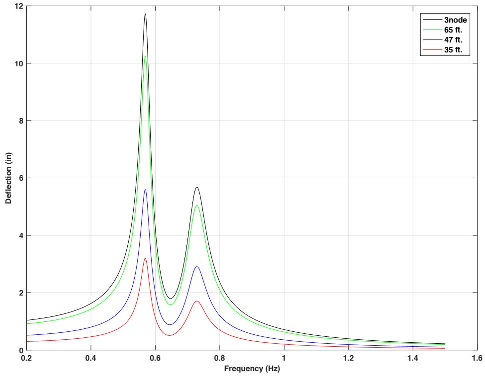
Figure 4-53 Frequency response for 70ft. mast arm with 15 lb. mass TMD at 2.5 ft from the tip,  $f_d = 1.0f_n$ , 5 lbf force on 3 signal head location (notation 3node means tip deflection under this situation)
