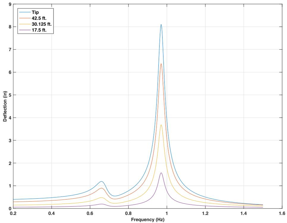
Figure 4-134 Frequency response for 50ft. mast arm with 15lb mass TMD, 5 lbf force on tip,
