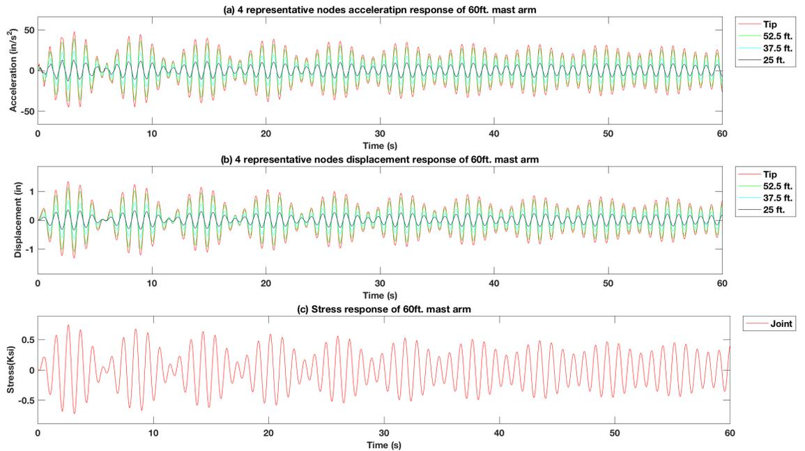
**Figure 4-80 Force vibration response of excitation force at tip of the 60 ft. mast arm signal pole structure model with 15 lb. mass TMD using the  $f_d = 0.5 f_n$ ,  $f_y = 1.2 f_n$**
