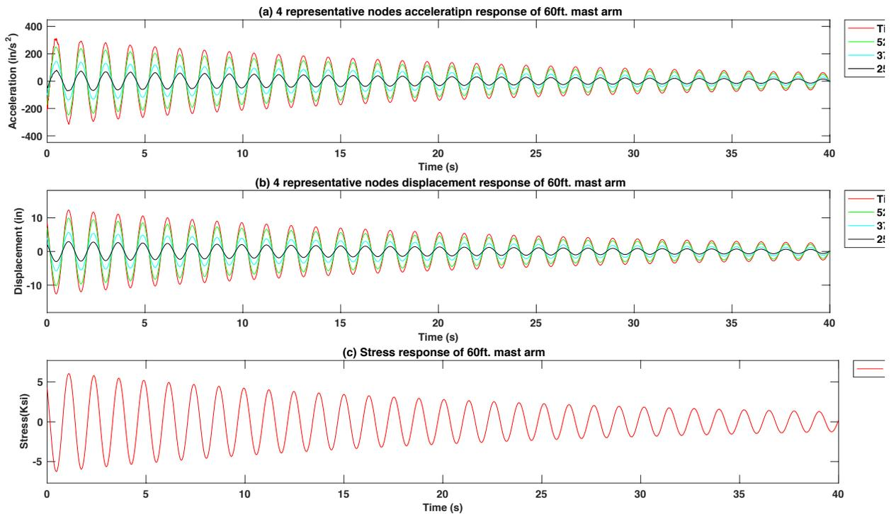
Figure 4-76 Free vibration response of excitation force at tip of the 60 ft. mast arm signal pole structure model with 15 lb. mass TMD using the  $f_d = 1.25 f_n$
