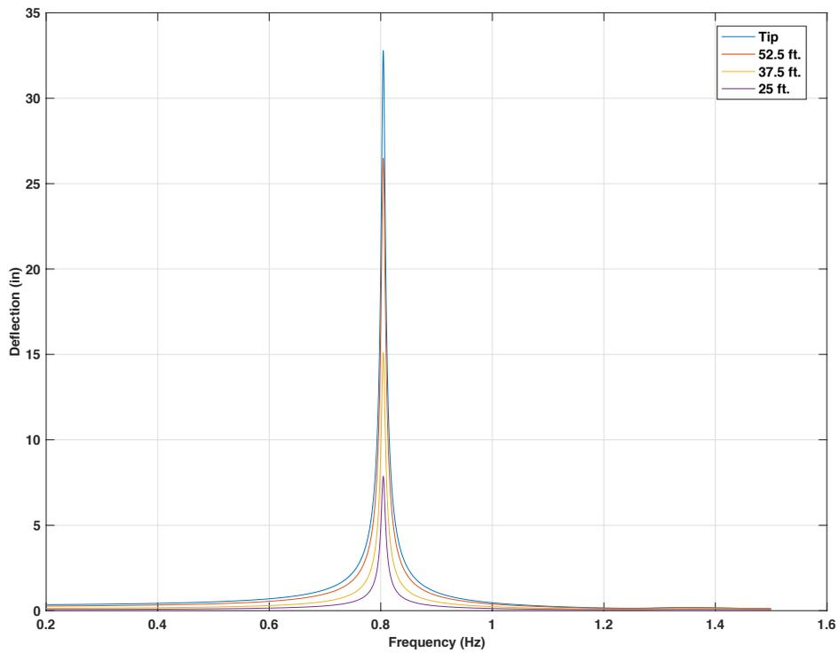
Figure 4-94 Frequency response for 60ft. mast arm with 15lb mass TMD, 5 lbf force on tip,  $f_d = 1.5 f_n$
