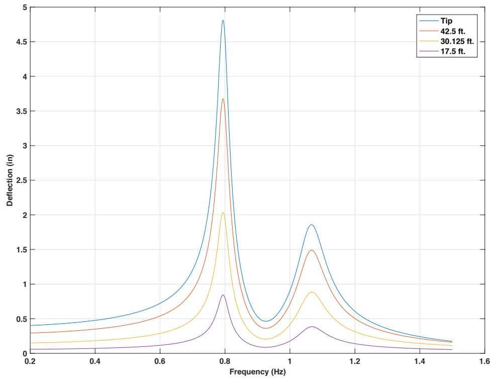
Figure 4-118 Frequency response for 50ft. mast arm with 15lb mass TMD, force on the tip
