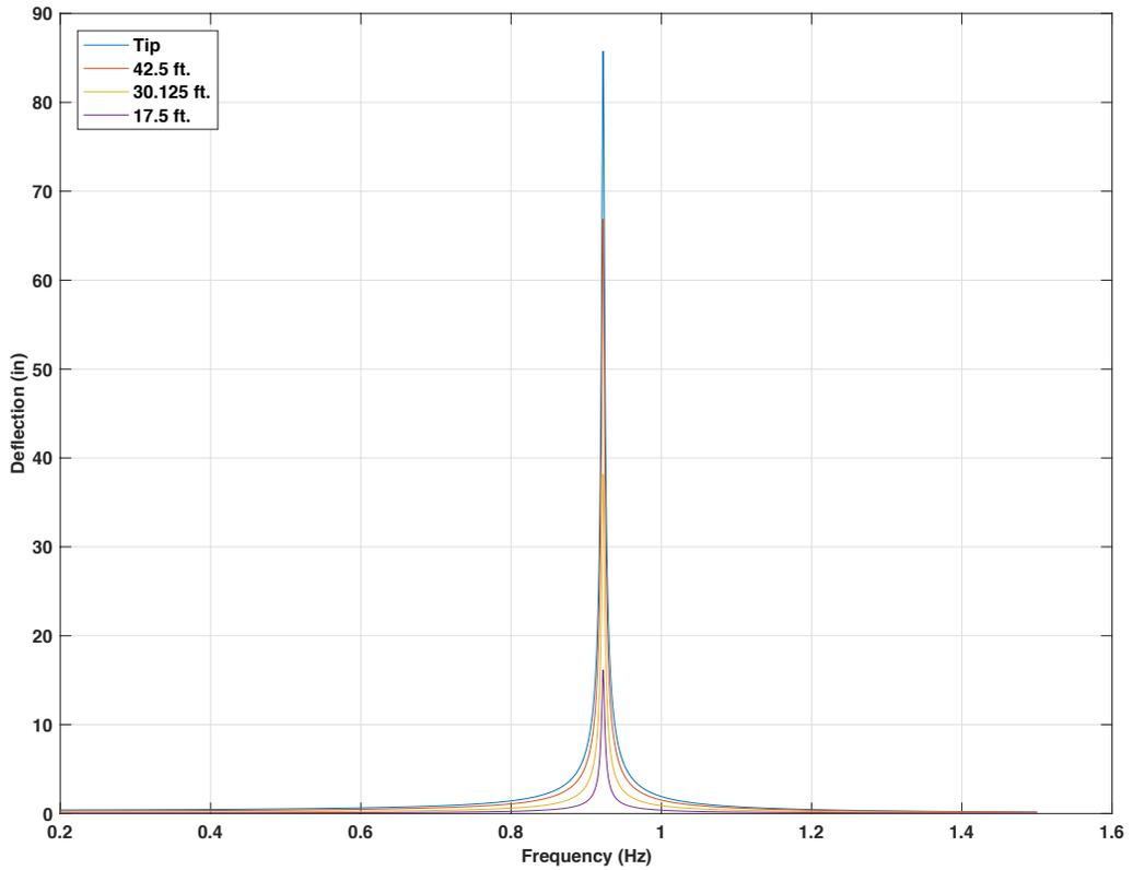
Figure 4-113 Harmonic response for excitation force on the mast arm tip of the 50 ft. arm signal support structure model without TMD
