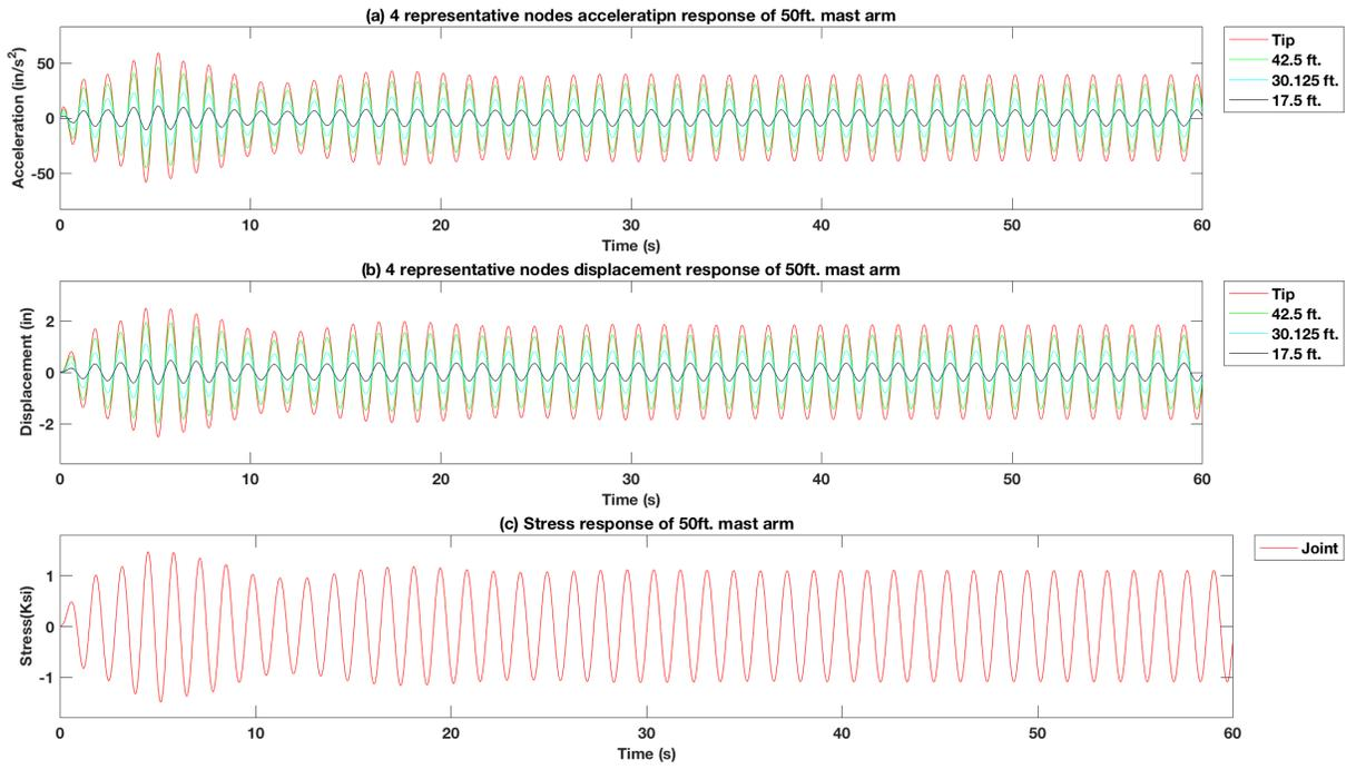
Figure 4-151 Force vibration response of excitation force at 3 signal heads position of the 50 ft. mast arm signal pole structure model TMD at 5 ft from the tip  $f_y = 0.7f_n$
