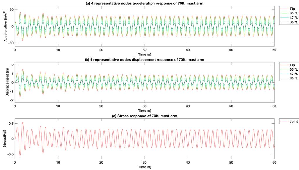
**Figure 4-17 Force vibration response of excitation force at signal heads' location of the 70 ft. mast arm signal pole structure model with 15 lb. mass TMD using the  $f_s = 1.3 f_n$**
