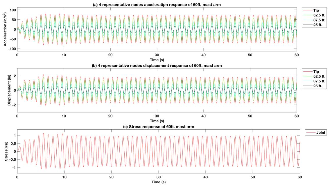
Figure 4-66 Force vibration response of excitation force at 3 signal heads location of the 60 ft. mast arm signal pole structure model with 15 lb. mass TMD using the  $f_x = 1.05 f_n$
