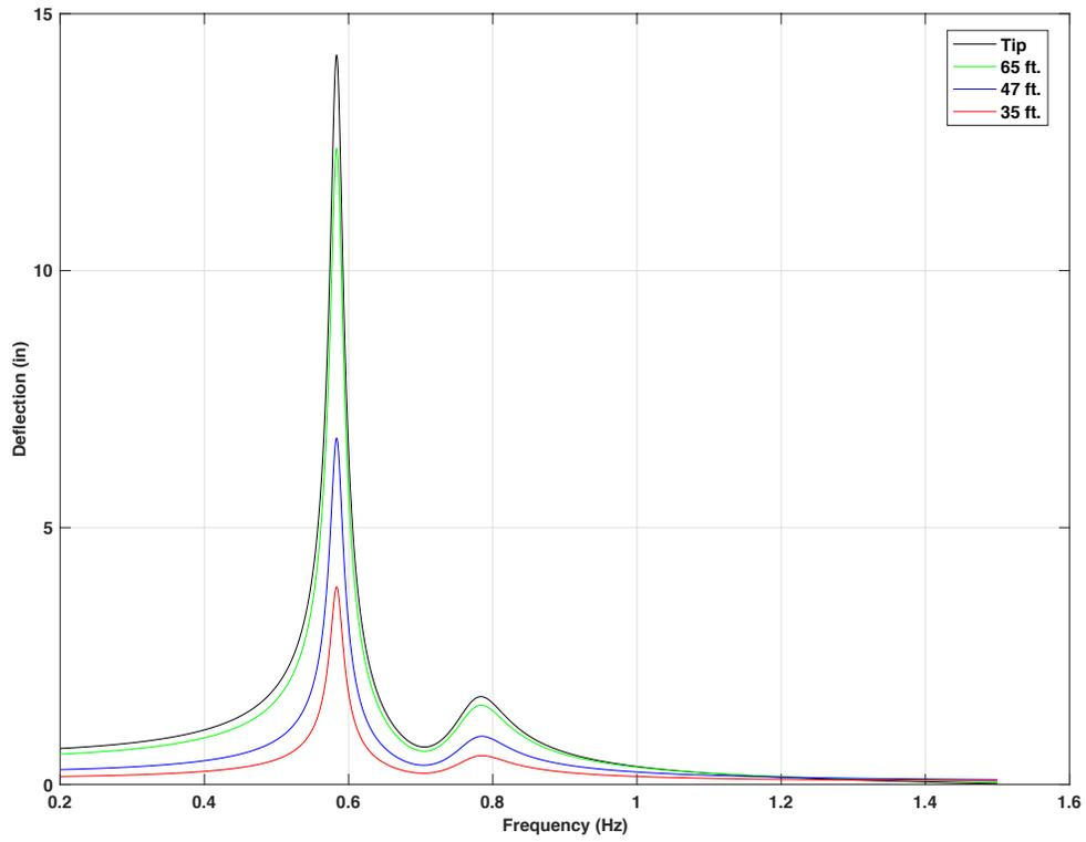
Figure 4-37 Frequency response for 70ft. mast arm with 15lb mass TMD, 5 lbf force on tip,  $f_d = 1.1 f_n$
