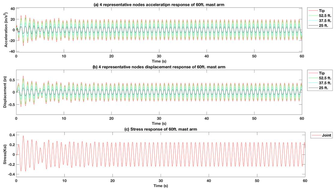
Figure 4-101 Force vibration response of excitation force at tip in the second mode frequency of the 60 ft. mast arm signal pole structure model TMD at 1.5 ft from the tip  $f_x = 1.2f_n$
