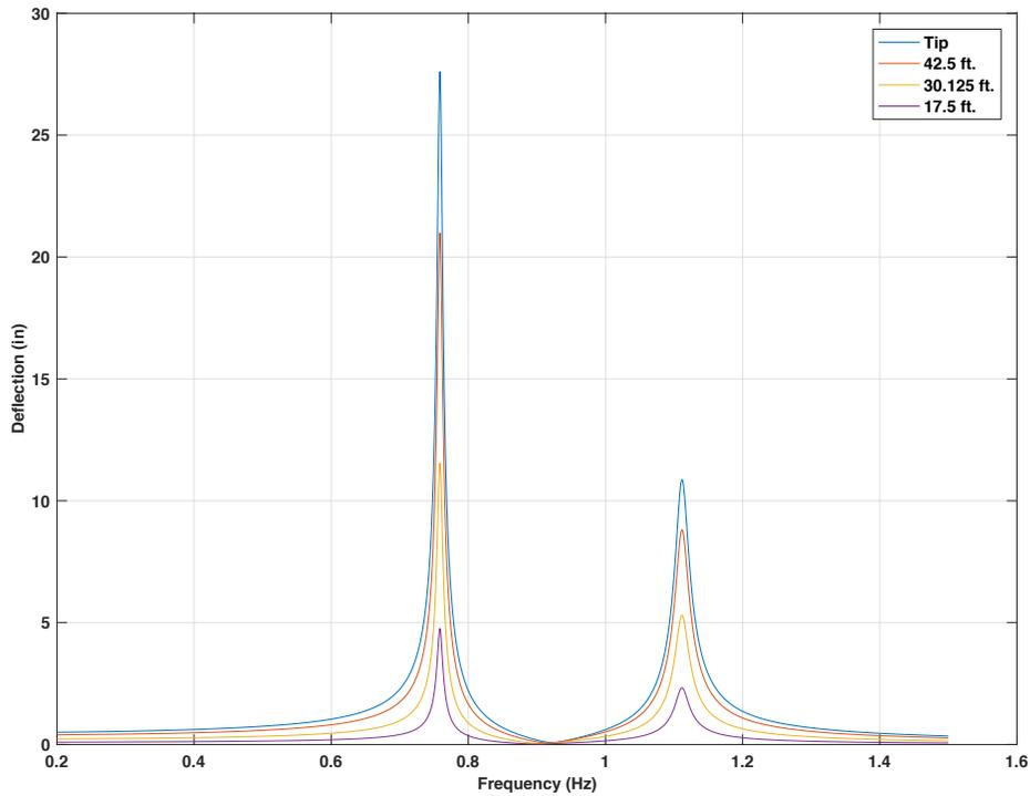
**Figure 4-148 Frequency response for 50ft. mast arm with 25 lb. mass TMD using the  $\zeta = 1\%$ , 5 lbf force on 3 signal head location**
