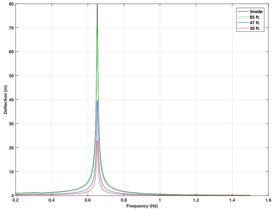
Figure 4-32 Frequency response for 70ft. mast arm with 15lb mass TMD, 5 lbf force on 3 signal heads location,  $f_d = 0.5 f_n$  (notation 3node means tip deflection under this situation)
