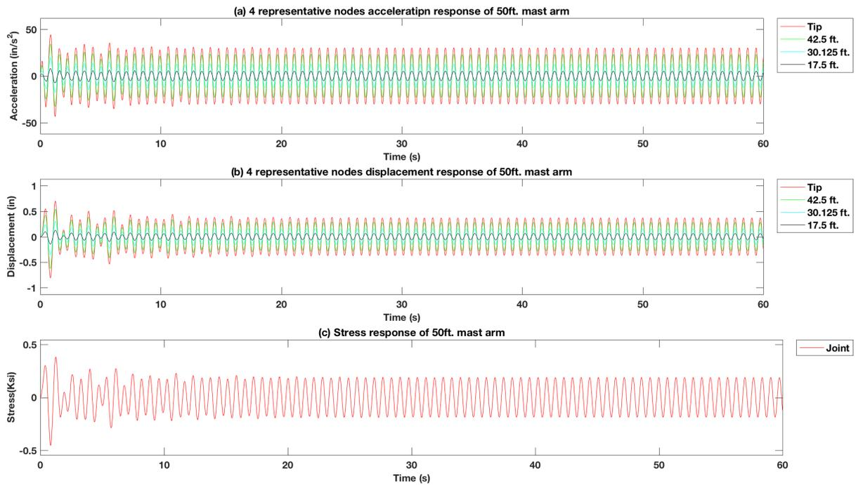
Figure 4-152 Force vibration response of excitation force at 3 signal heads position of the 50 ft. mast arm signal pole structure model TMD at 10 ft from the tip  $f_y = 1.4f_n$
