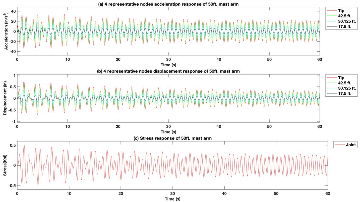
Figure 4-128 Force vibration response of excitation force at tip of the 50 ft. mast arm signal pole structure model with 15 lb. mass TMD using the  $f_d = 0.5 f_n$ ,  $f_x = 1.4 f_n$
