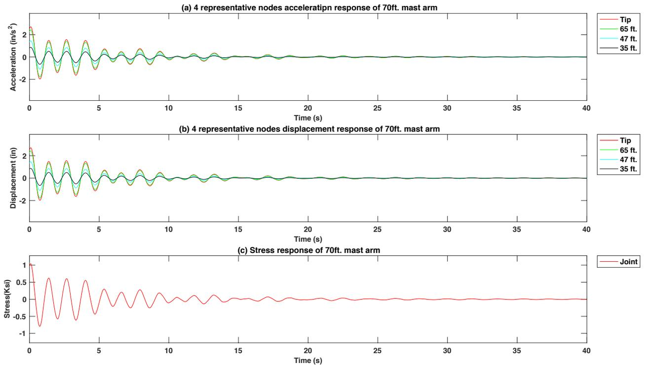
**Figure 4-9 Free vibration response of the 70 ft. arm signal support structure model with 25 lb. TMD in the same frequency of the structure**
