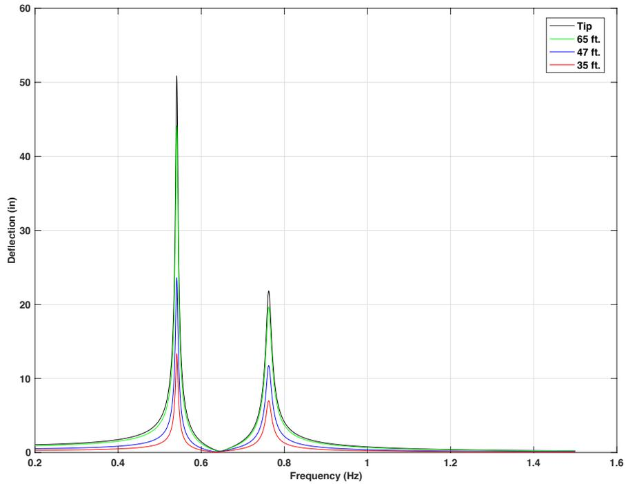
Figure 4-47 Frequency response for 70ft. mast arm with 25 lb. mass TMD using the  $\zeta = 1\%$ , 5 lbf force on 3 signal head location
