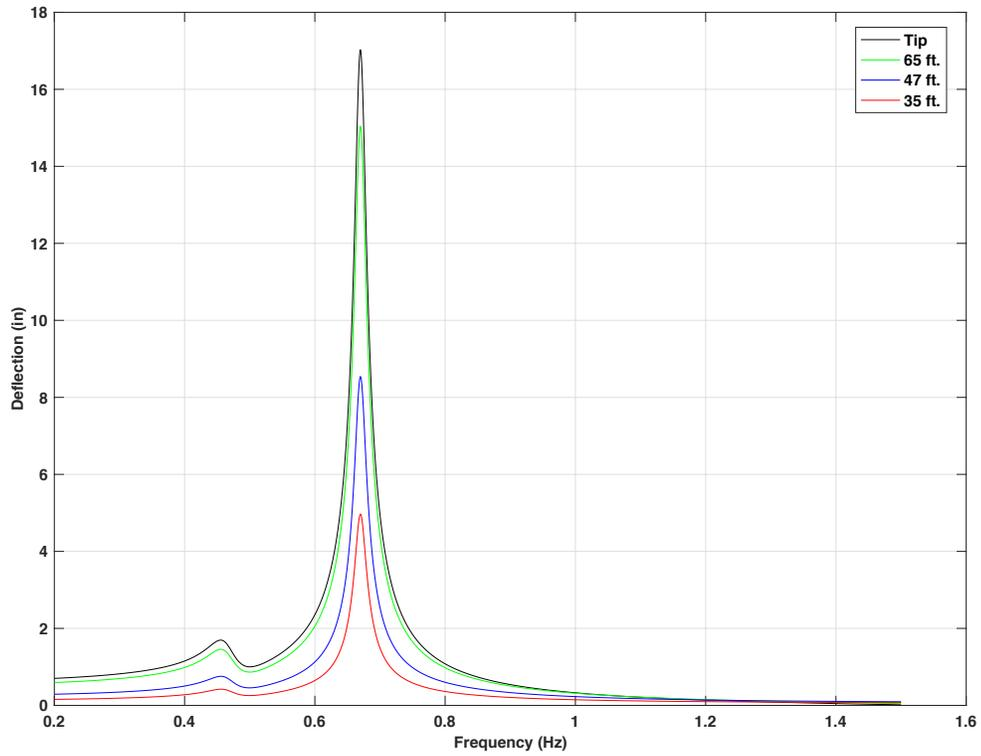
Figure 4-33 Frequency response for 70ft. mast arm with 15lb mass TMD, 5 lbf force on tip,  $f_d = 0.75 f_n$
