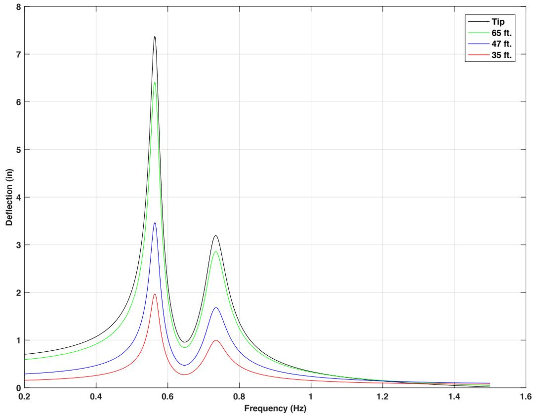
**Figure 4-13 Frequency response for 70ft. mast arm with 15lb mass TMD, force on the tip**
