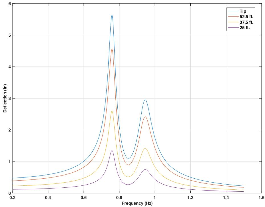
Figure 4-107 Frequency response for 60ft. mast arm with 15 lb. mass TMD at 5 ft from the tip,
