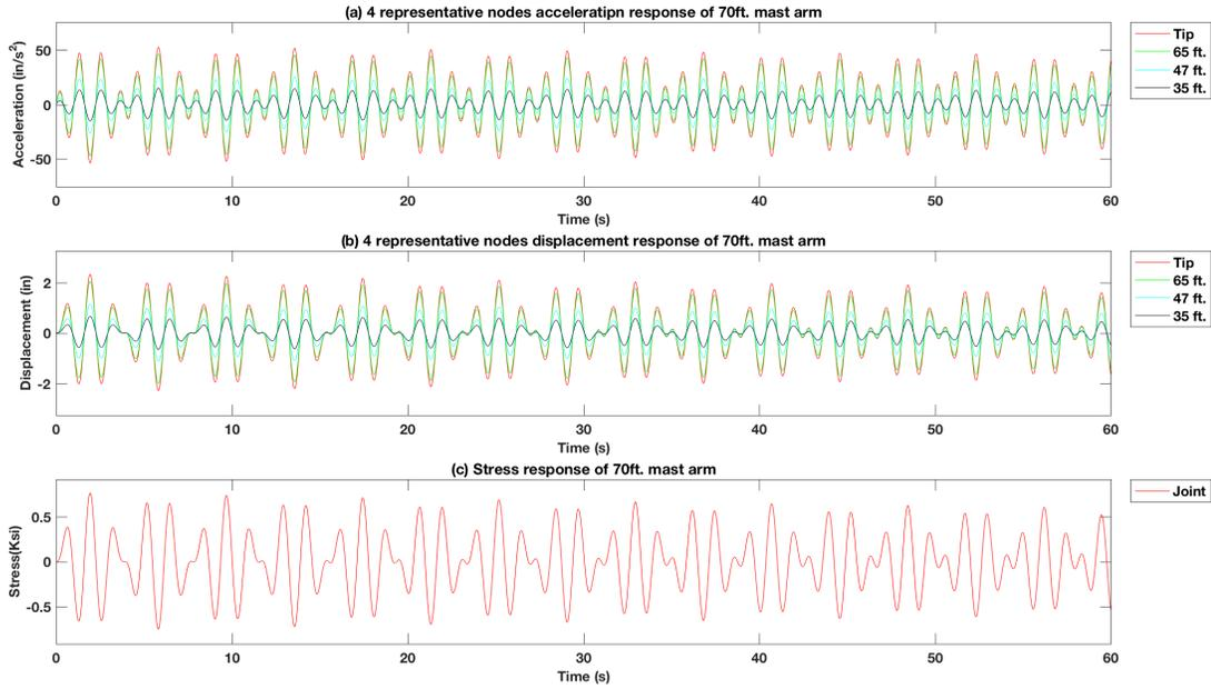
**Figure 4-6 Force vibration response of excitation force at mast arm signal heads locations in  $f_x = 1.5 \times \text{Natural frequency}$  of the 70 ft. arm signal support structure model without TMD**
