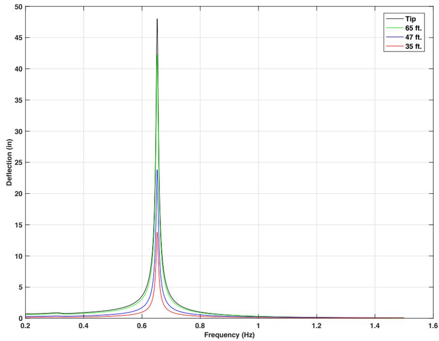
Figure 4-31 Frequency response for 70ft. mast arm with 15lb mass TMD, 5 lbf force on tip,  $f_d = 0.5 f_n$
