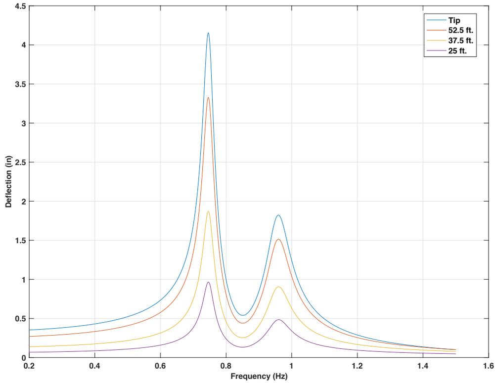
**Figure 4-71 Frequency response for 60ft. mast arm with 25lb mass TMD, force on the tip**
