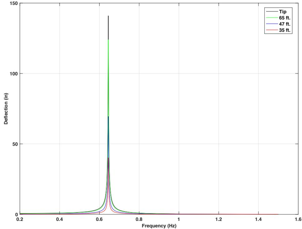
**Figure 4-5 Harmonic response for excitation force on the mast arm tip of the 70 ft. arm signal support structure model without TMD**
