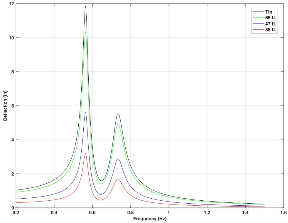
**Figure 4-19 Frequency response for 70ft. mast arm with 15lb mass TMD, force on signal heads' location**
