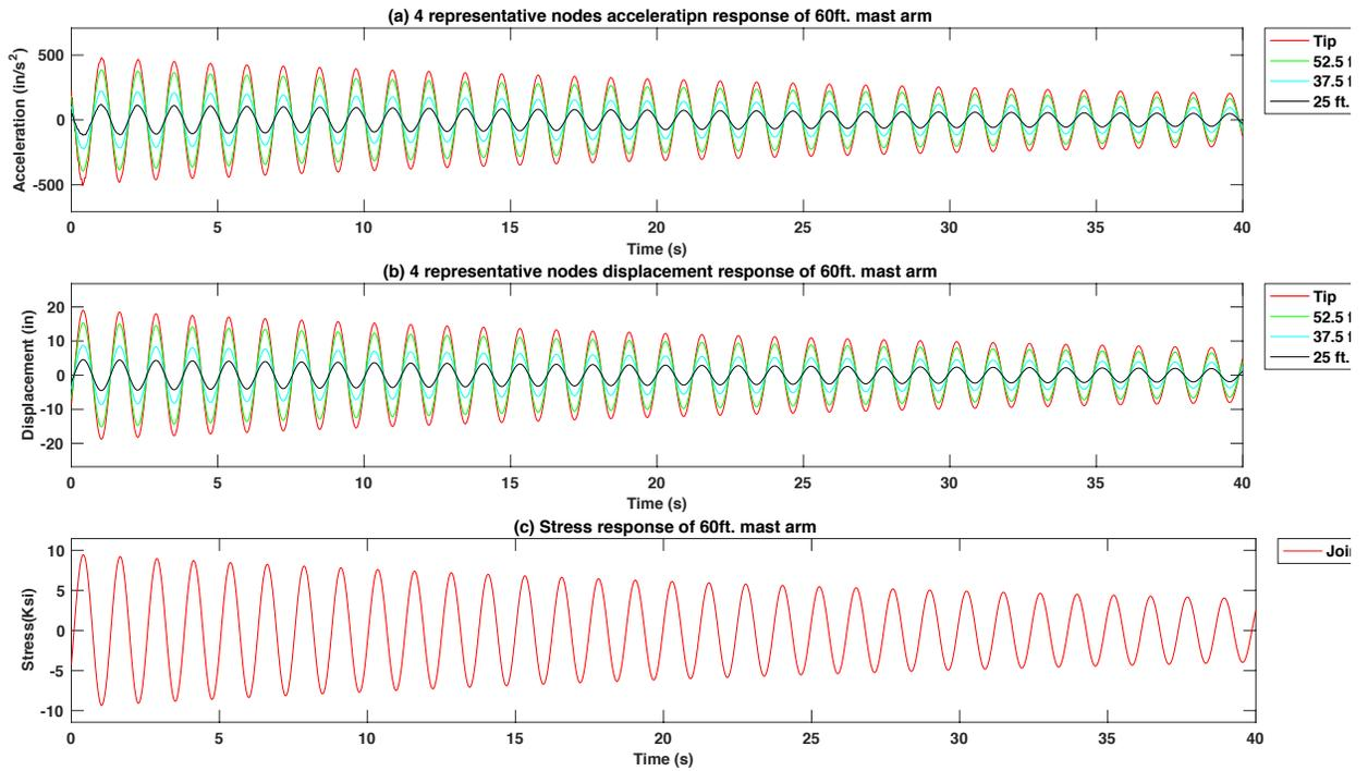
Figure 4-77 Free vibration response of excitation force at tip of the 60 ft. mast arm signal pole structure model with 15 lb. mass TMD using the  $f_d = 1.5 f_n$
