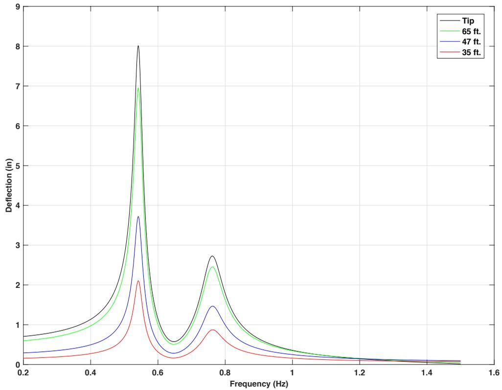
Figure 4-16 Frequency response for 70ft. mast arm with 25lb mass TMD, force on the tip
