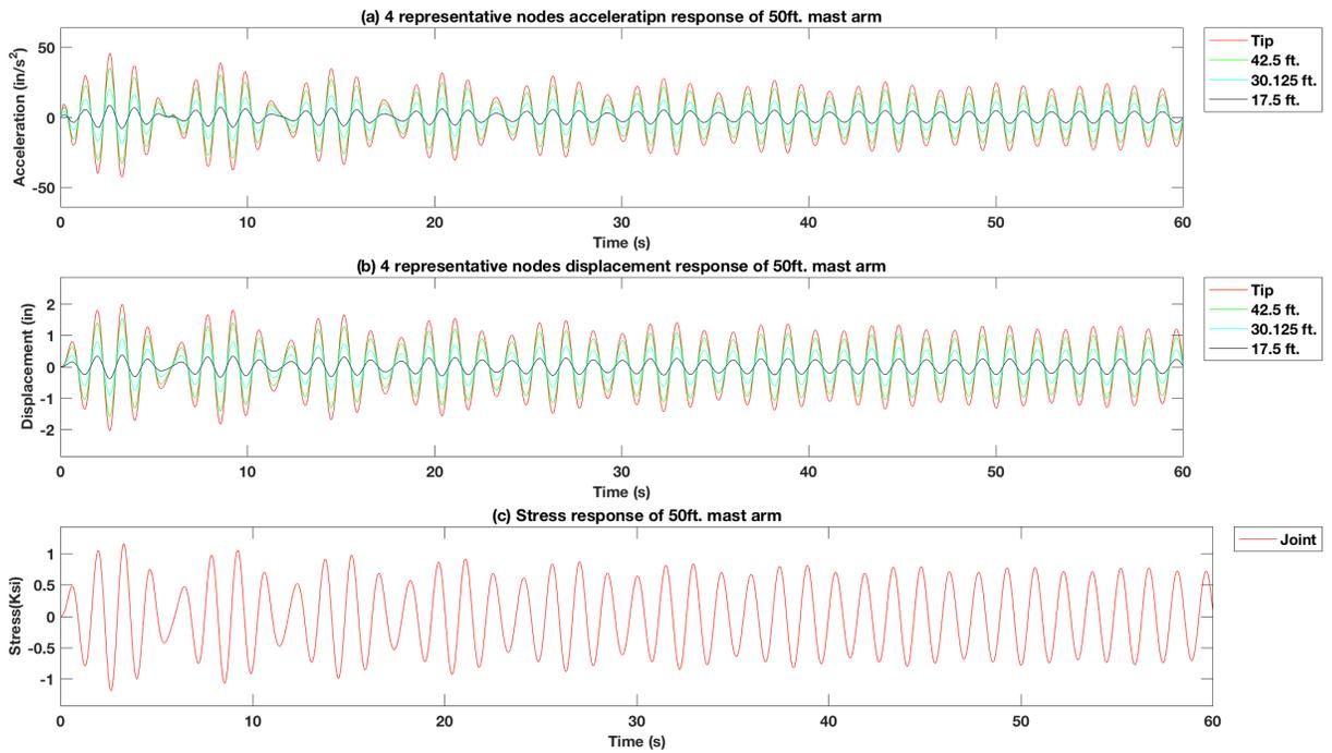
**Figure 4-130 Force vibration response of excitation force at 3 signal heads location of the 50 ft. mast arm signal pole structure model with 15 lb. mass TMD using the  $f_d = 1.25 f_n$ ,  $f_y = 0.8 f_n$**
