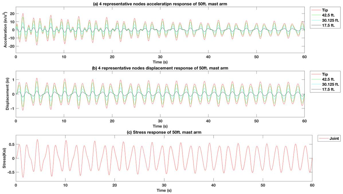
**Figure 4-129 Force vibration response of excitation force at 3 signal heads location of the 50 ft. mast arm signal pole structure model with 15 lb. mass TMD using the  $f_d = 1.5 f_n$ ,  $f_y = 0.6 f_n$**
