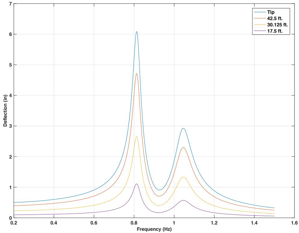
Figure 4-156 Frequency response for 50ft. mast arm with 15 lb. mass TMD at 5 ft from the tip,
