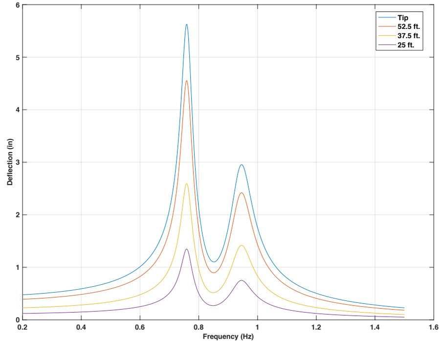
Figure 4-105 Frequency response for 60ft. mast arm with 15 lb. mass TMD at 2.5 ft from the tip, 5 lbf force on 3 signal head location,  $f_d = 1.0f_n$
