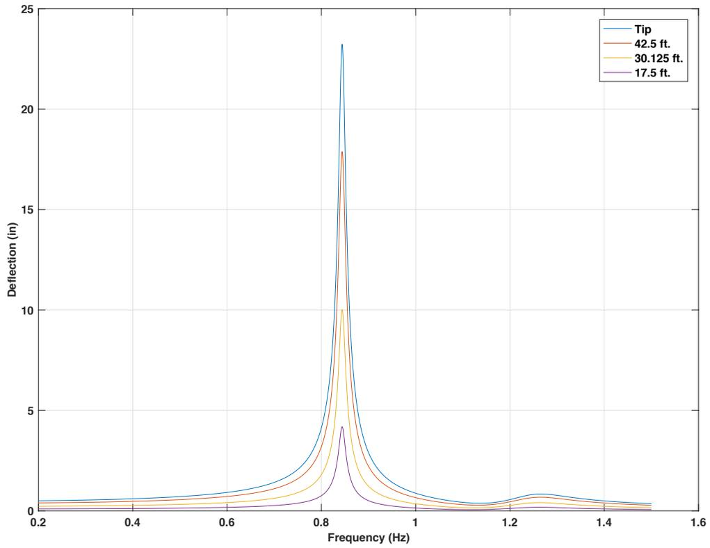
Figure 4-141 Frequency response for 50ft. mast arm with 15lb mass TMD, 5 lbf force on 3 signal heads location,  $f_d = 1.25 f_n$
