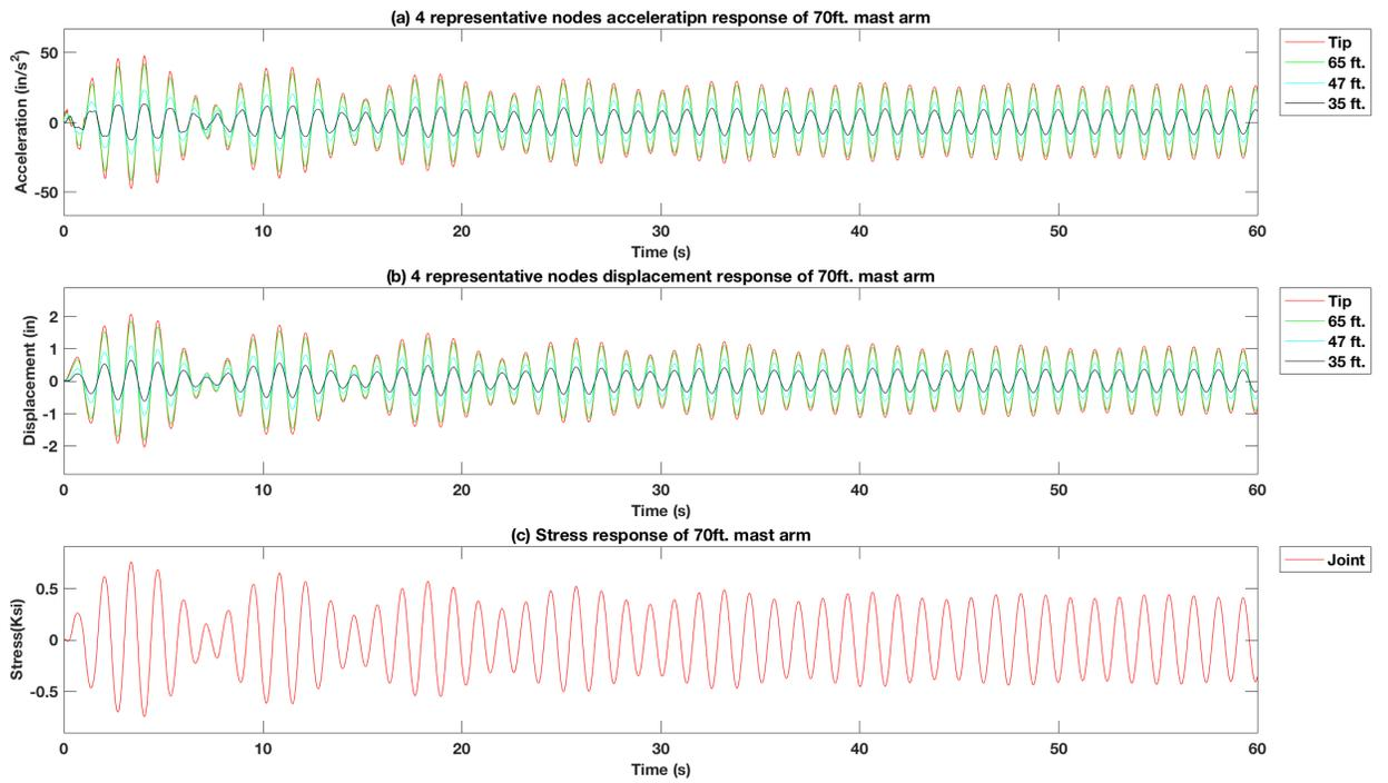
Figure 4-27 Force vibration response of excitation force at tip of the 70 ft. mast arm signal pole structure model with 15 lb. mass TMD using the  $f_d = 0.75 f_n$ ,  $f_x = 1.2 f_n$
