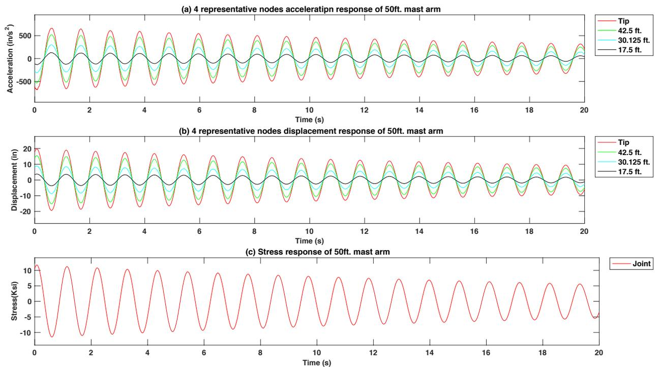
**Figure 4-122 Free vibration response of excitation force at tip of the 50 ft. mast arm signal pole structure model with 15 lb. mass TMD using the  $f_d = 0.5 f_n$**
