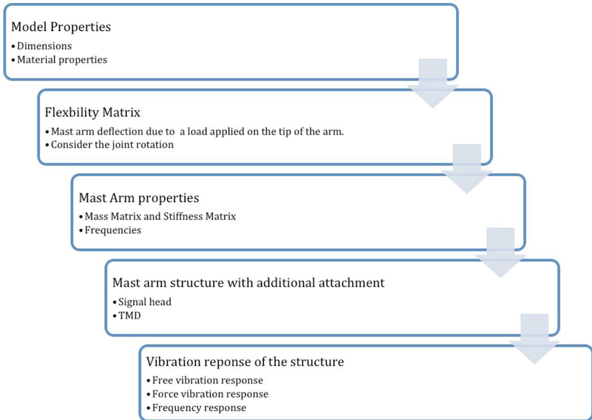
**Figure 3-4 Flowchart of the procedures of Analysis**
