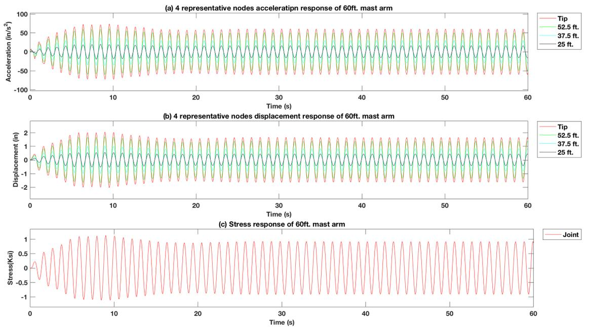
Figure 4-78 Force vibration response of excitation force at tip of the 60 ft. mast arm signal pole structure model with 15 lb. mass TMD using the  $f_d = 0.9 f_n, f_s = 1.05 f_n$
