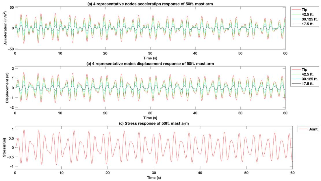
Figure 4-112 Force vibration response of excitation force at 3 signal head locations in  $f_v = 0.7 f_n$  of the 50 ft. arm signal support structure model without TMD
