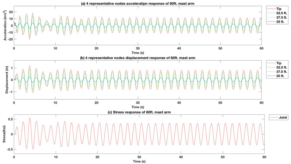
Figure 4-69 Force vibration response of excitation force at tip of the 60 ft. mast arm signal pole structure model with 25 lb. mass TMD using the  $f_x = 0.6 f_n$
