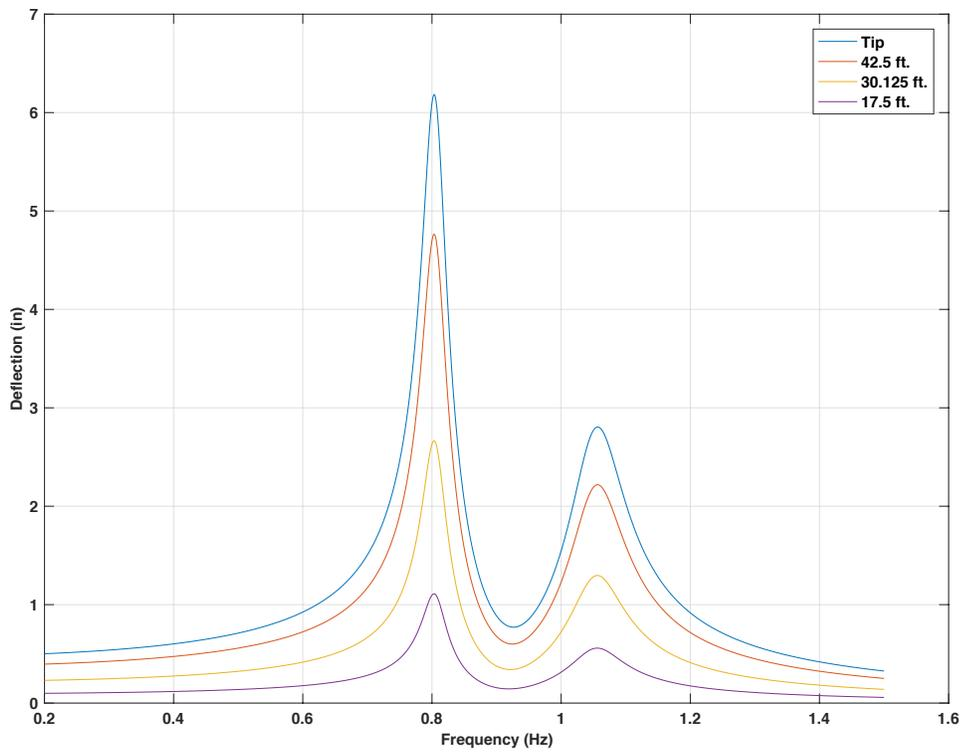
Figure 4-154 Frequency response for 50ft. mast arm with 15 lb. mass TMD at 1.5 ft from the tip, 5 lbf force on 3 signal head location,  $f_d = 1.0f_n$
