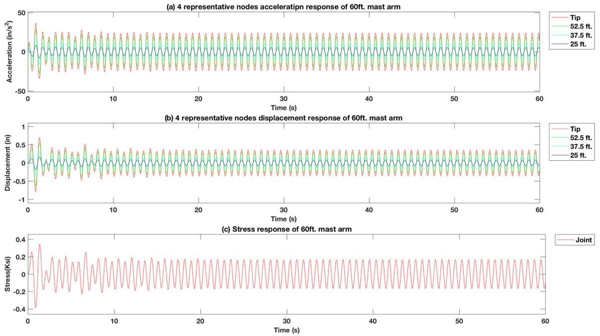
Figure 4-103 Force vibration response of excitation force at 3 signal heads position of the 60 ft. mast arm signal pole structure model TMD at 10 ft from the tip  $f_y = 1.4f_n$
