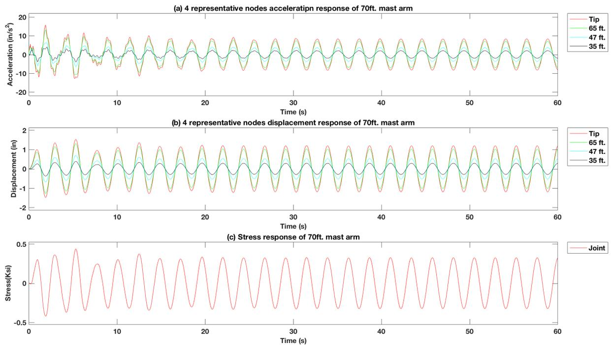
Figure 4-26 Force vibration response of excitation force at tip of the 70 ft. mast arm signal pole structure model with 15 lb. mass TMD using the  $f_d = 0.9 f_n$ ,  $f_y = 0.6 f_n$
