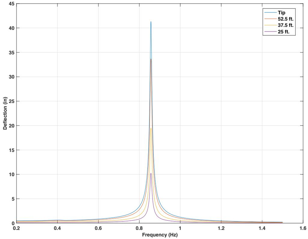
Figure 4-85 Frequency response for 60ft. mast arm with 15lb mass TMD, 5 lbf force on 3 signal heads location,  $f_d = 0.5 f_n$
