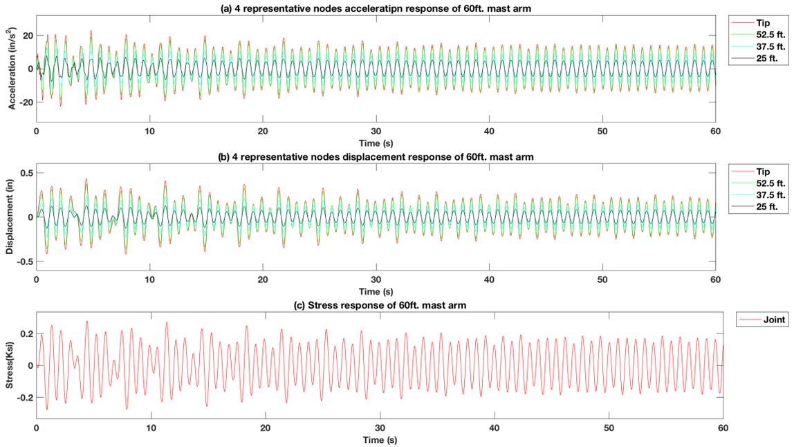
Figure 4-97 Force vibration response of excitation force at tip of the 60 ft. mast arm signal pole structure model with 25 lb. mass TMD using the  $\zeta = 1\%$ ,  $f_x = 1.3f_n$ .
