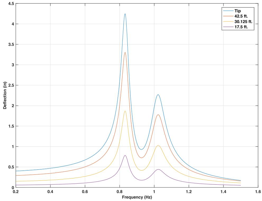
Figure 4-157 Frequency response for 50ft. mast arm with 15 lb. mass TMD at 10 ft from the tip
