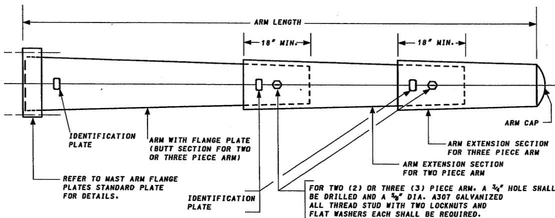
Figure 3-2 Standard Mast Arms (Signal Standard No. MD 818.13, 2007 Revised)
