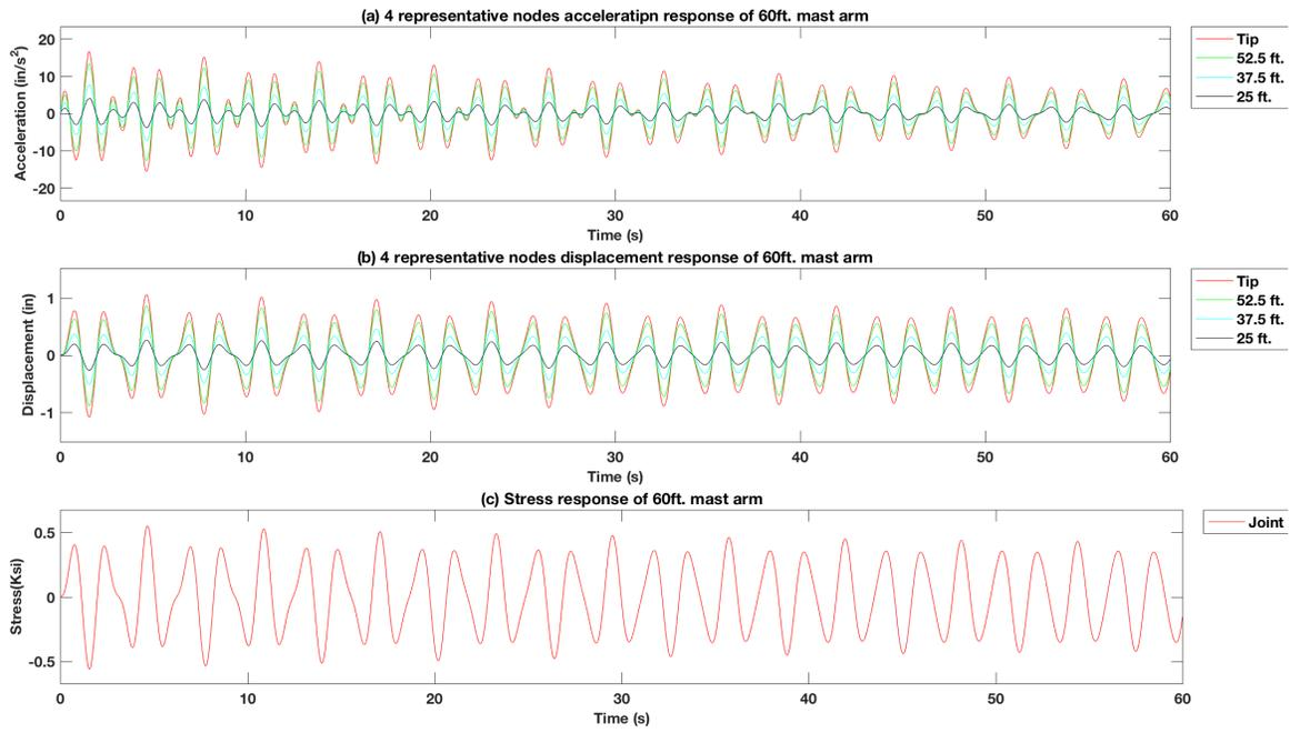
**Figure 4-81 Force vibration response of excitation force at 3 signal heads location of the 60 ft. mast arm signal pole structure model with 15 lb. mass TMD using the  $f_d = 1.5 f_n$ ,  $f_y = 0.6 f_n$**
