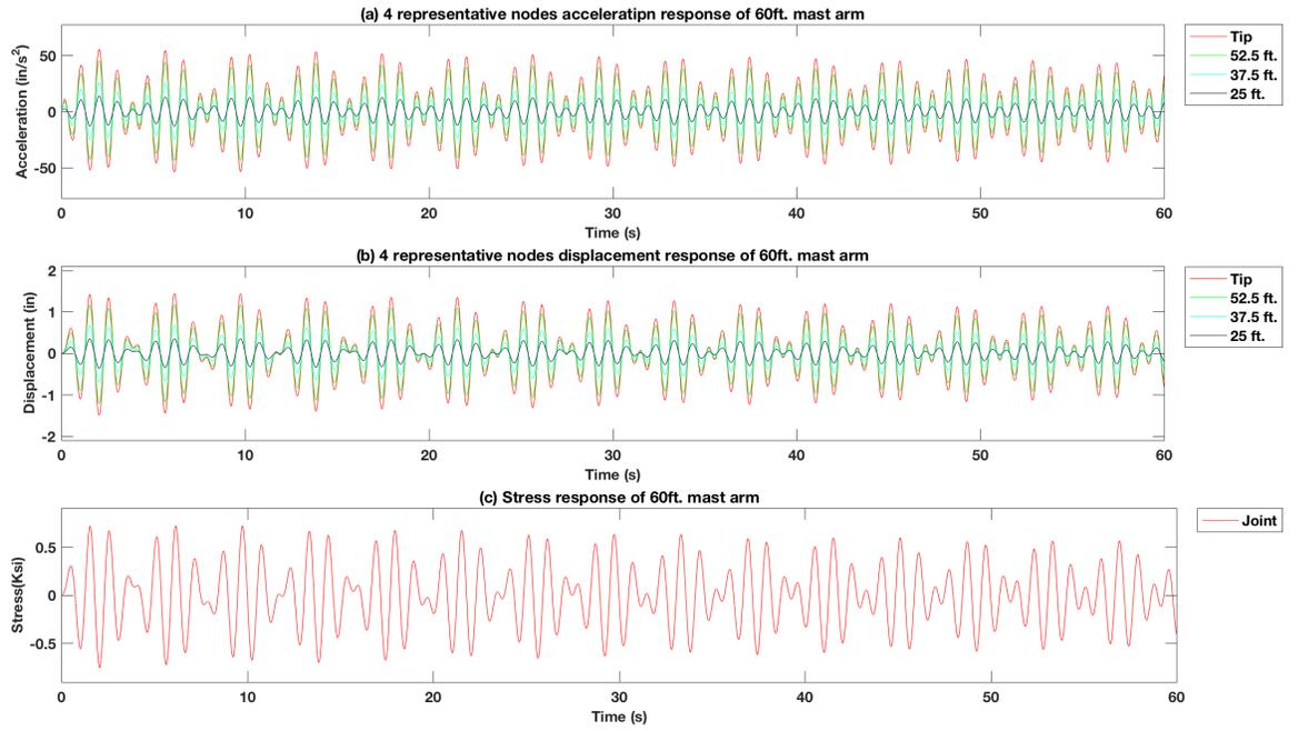
**Figure 4-60 Force vibration response of excitation force at tip in  $f_y = 1.3 \times f$  of the 60 ft. arm signal support structure model without TMD**
