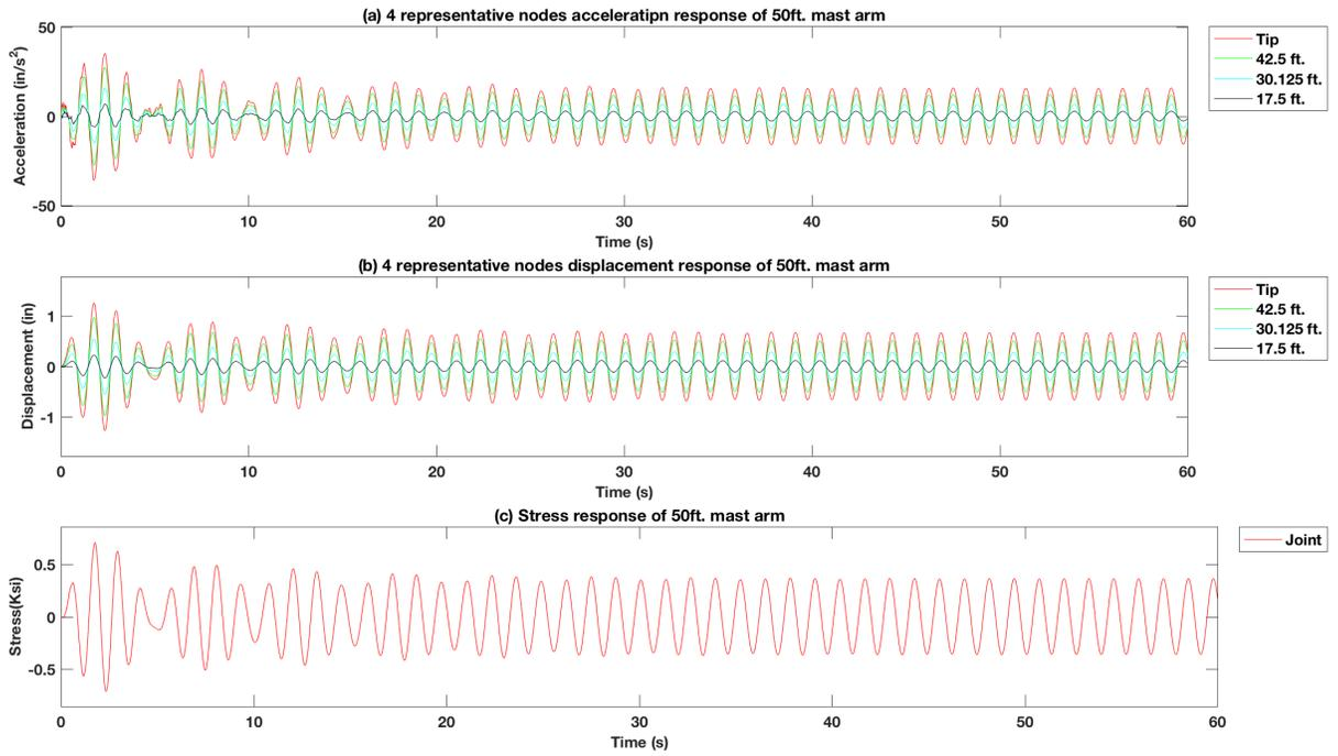
Figure 4-127 Force vibration response of excitation force at tip of the 50 ft. mast arm signal pole structure model with 15 lb. mass TMD using the  $f_d = 0.75 f_n$ ,  $f_x = 0.4 f_n$
