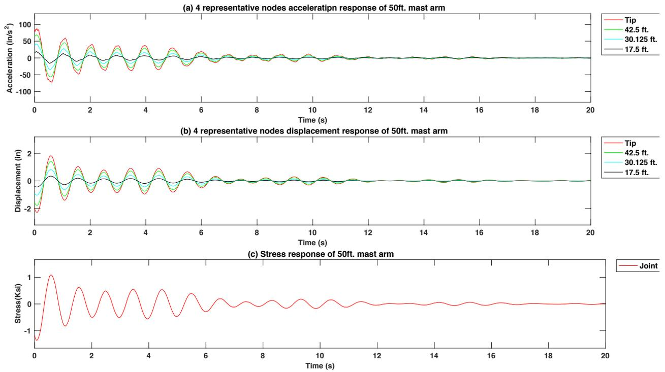
Figure 4-149 Free vibration response of excitation force at tip in the second mode frequency of the 50 ft. mast arm signal pole structure model with 15 lb. mass TMD at 10 ft from the tip
