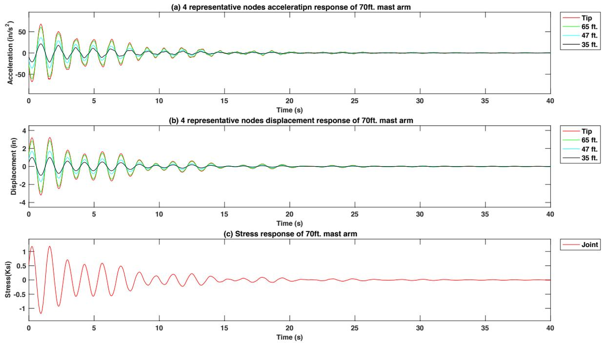
**Figure 4-8 Free vibration response of the 70 ft. arm signal support structure model with 15 lb. TMD in the same frequency of the structure**
