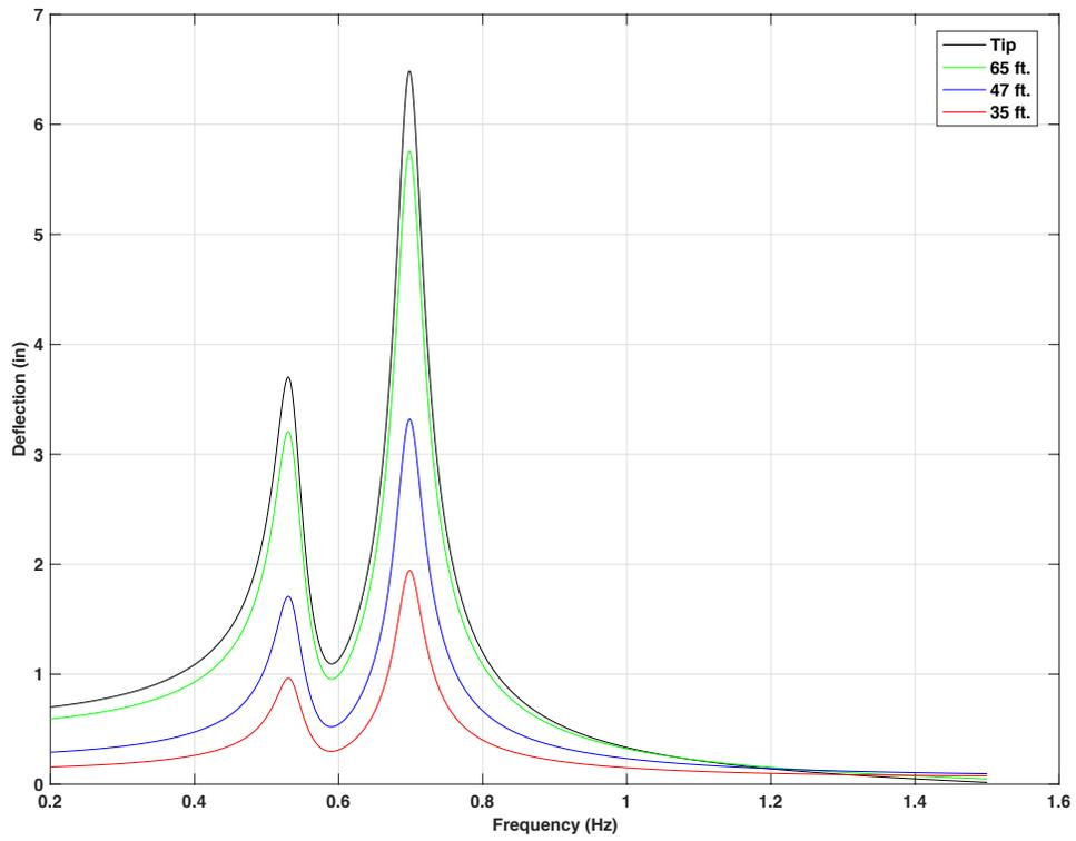
Figure 4-35 Frequency response for 70ft. mast arm with 15lb mass TMD, 5 lbf force on tip,  $f_d = 0.9 f_n$
