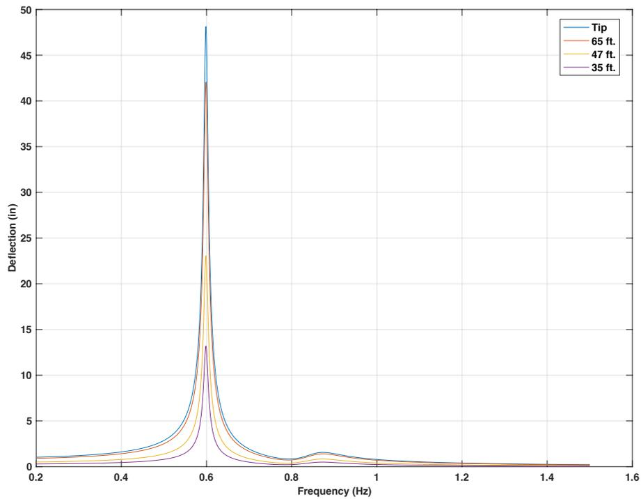
Figure 4-40 Frequency response for 70ft. mast arm with 15lb mass TMD, 5 lbf force on 3 signal heads location,  $f_d = 1.25 f_n$
