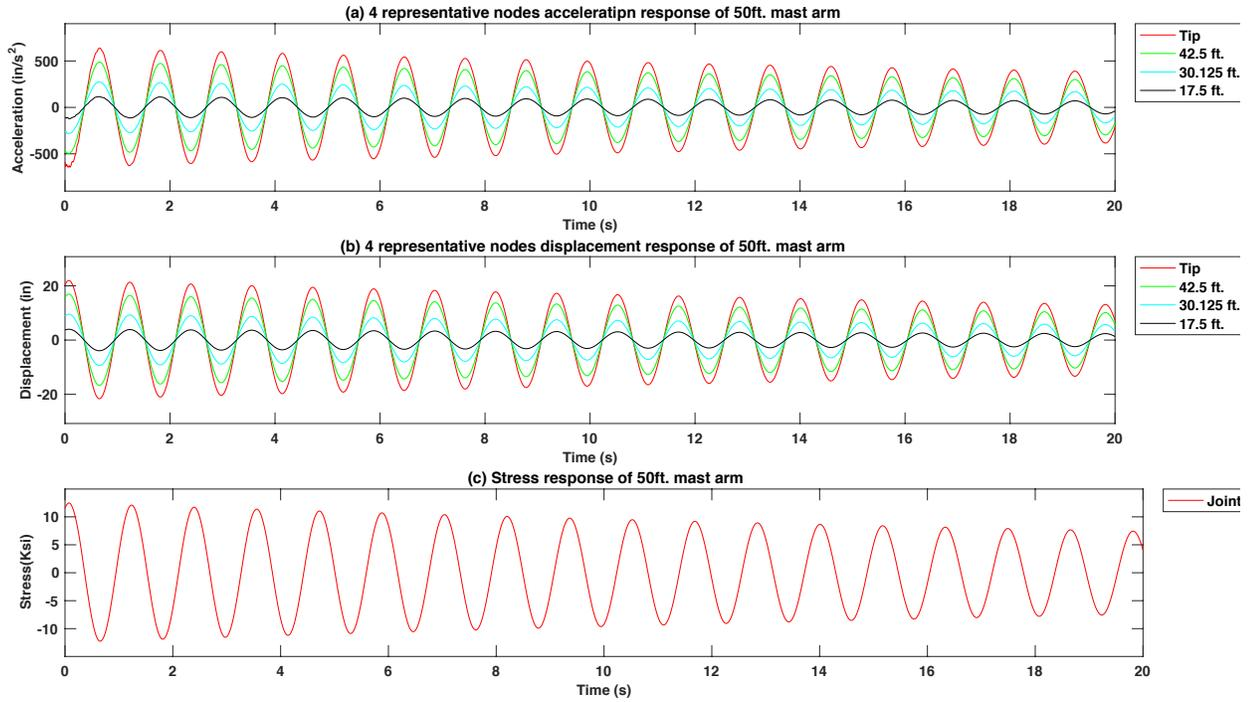
Figure 4-125 Free vibration response of excitation force at tip of the 50 ft. mast arm signal pole structure model with 15 lb. mass TMD using the  $f_d = 1.5 f_n$
