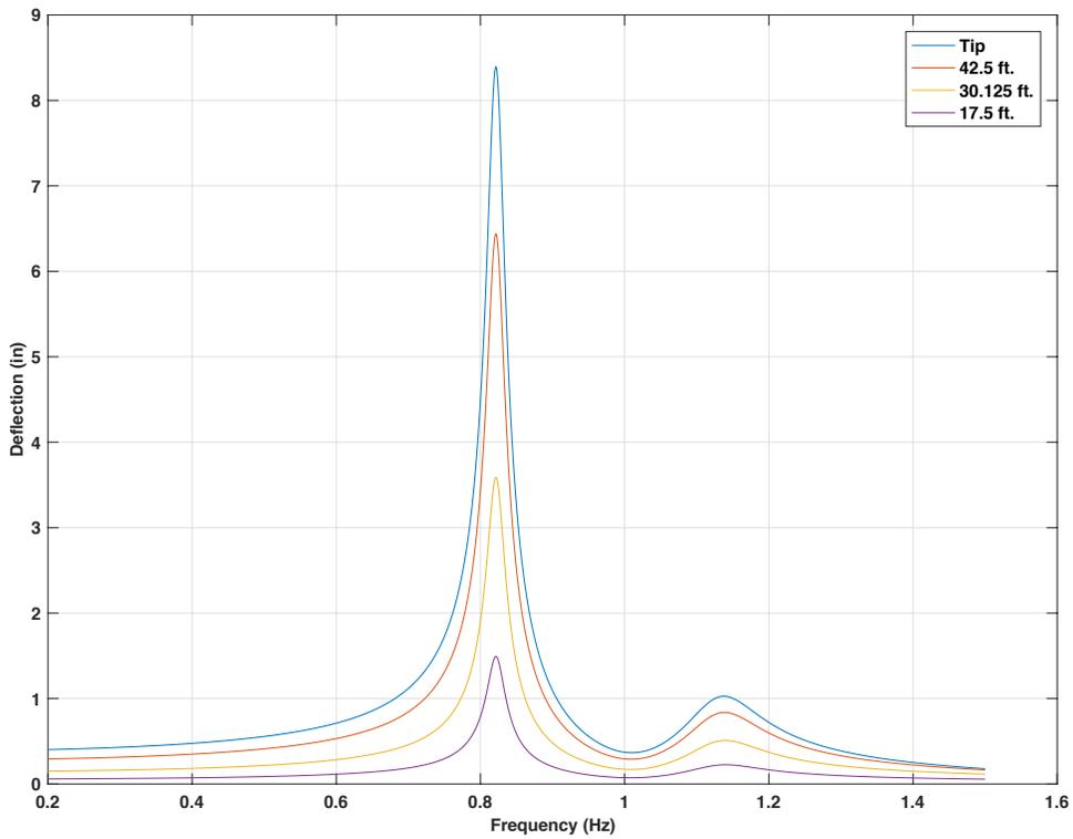
Figure 4-138 Frequency response for 50ft. mast arm with 15lb mass TMD, 5 lbf force on tip,  $f_d = 1.1 f_n$
