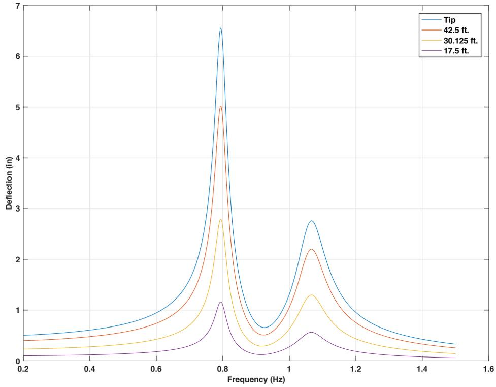
**Figure 4-119** Frequency response for 50ft. mast arm with 15lb mass TMD, force on signal heads' location
