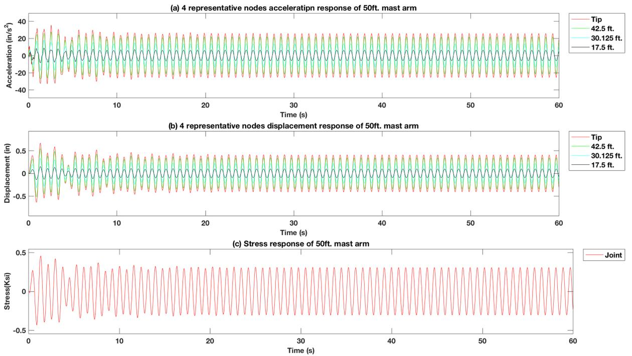
Figure 4-150 Force vibration response of excitation force at tip in the second mode frequency of the 50ft. mast arm signal pole structure model TMD at 2.5 ft from the tip  $f_x = 1.2f_n$
