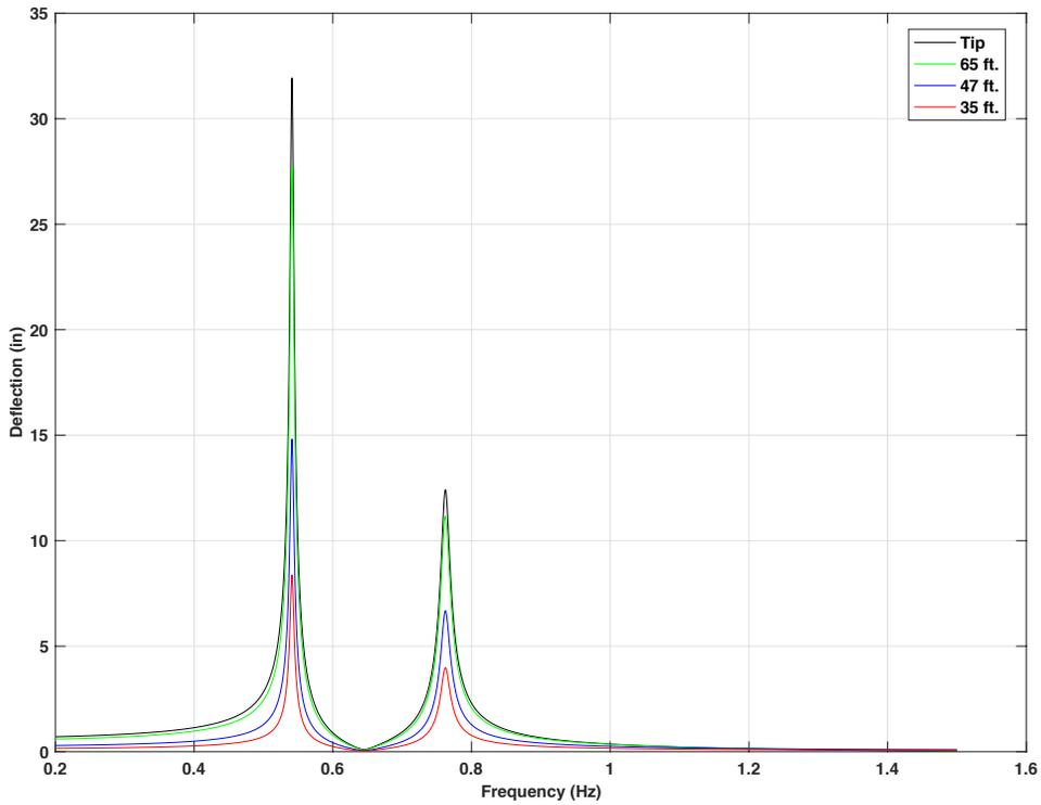
Figure 4-46 Frequency response for 70ft. mast arm with 25 lb. mass TMD using the  $\zeta = 1\%$ , 5 lbf force on tip of mast arm,  $f_d = 1.0f_n$
