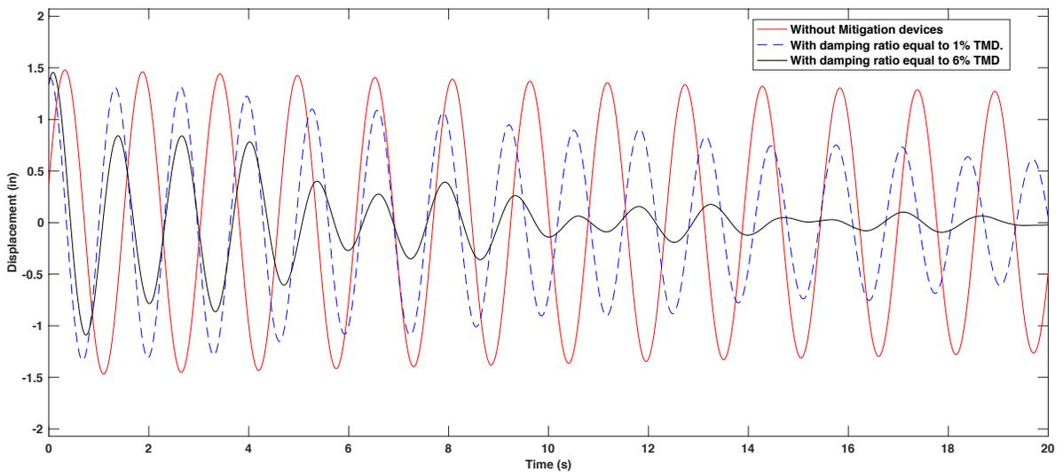
**Figure 4-159 Comparison of free vibration response curve of 70 feet mast arm**
