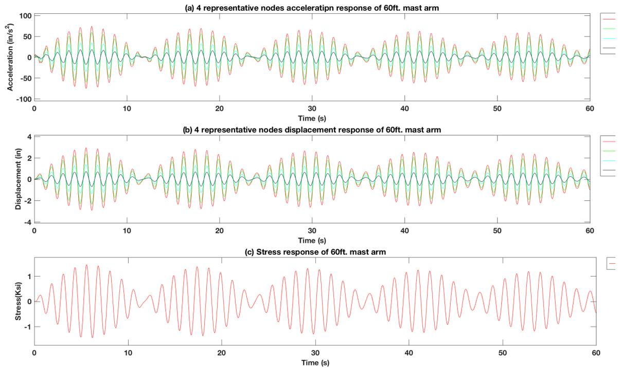
Figure 4-59 Force vibration response of excitation force at tip in  $f_x = 0.9 \times f$  of the 60 ft. mast arm signal pole structure model without TMD
