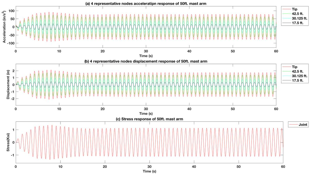
Figure 4-126 Force vibration response of excitation force at tip of the 50 ft. mast arm signal pole structure model with 15 lb. mass TMD using the  $f_d = 0.9 f_n, f_s = 1.05 f_n$
