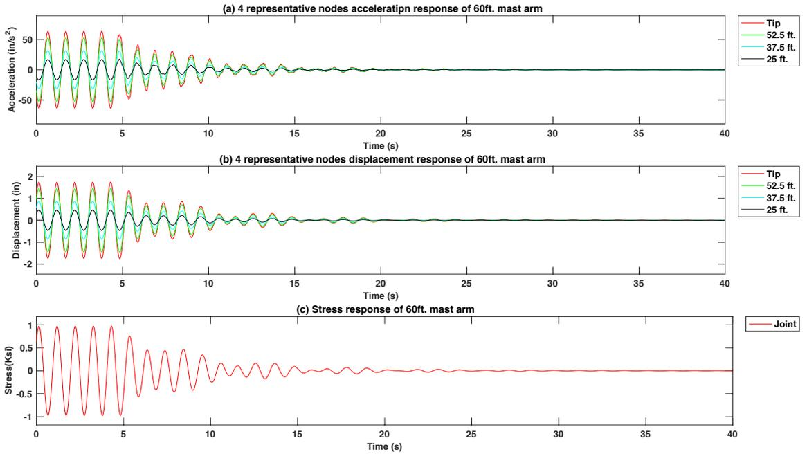
**Figure 4-63 Free vibration response of the 60 ft. arm signal support structure model with 15lb. TMD in the same frequency of the structure**
