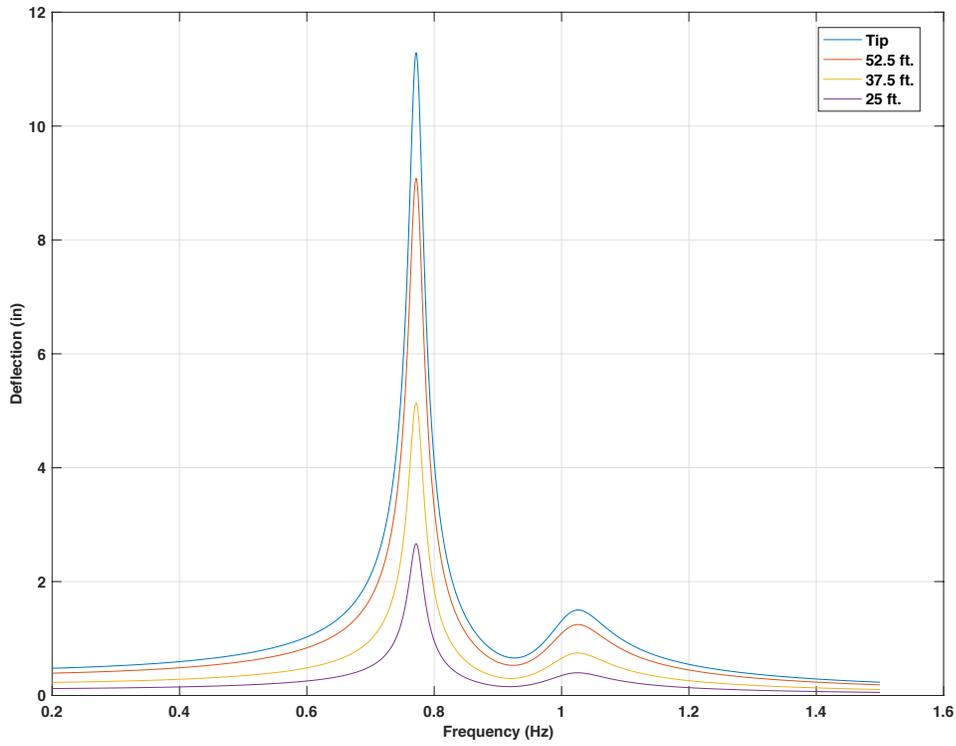
Figure 4-91 Frequency response for 60ft. mast arm with 15lb mass TMD, 5 lbf force on 3 signal heads location,  $f_d = 1.1 f_n$
