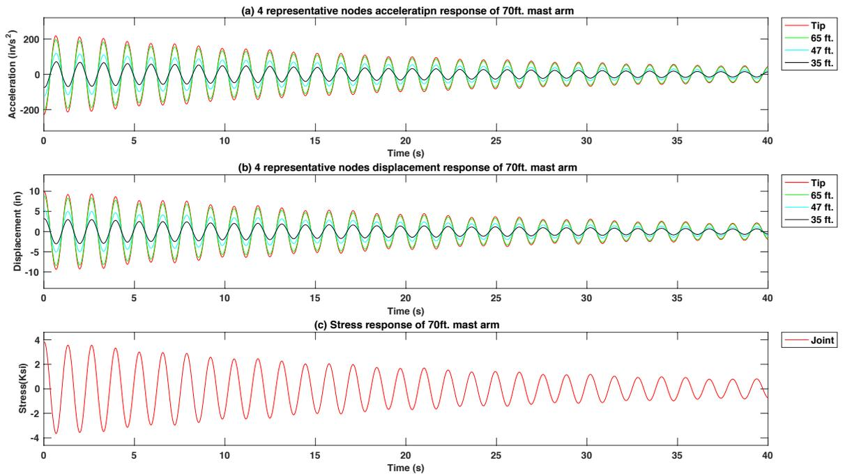
Figure 4-43 Free vibration response of excitation force at tip on the 70 ft. mast arm signal pole structure model with 25 lb. mass TMD using the  $\zeta = 1\%$
