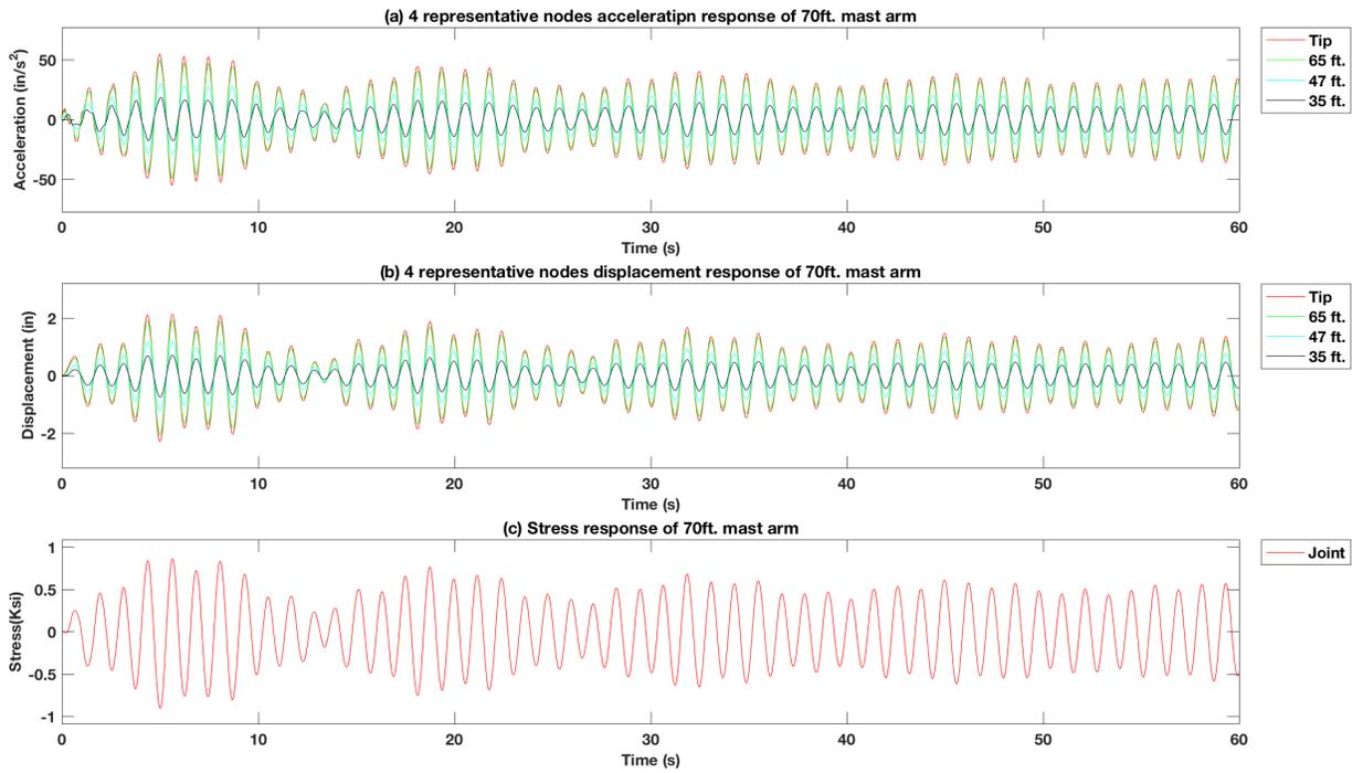
**Figure 4-44 Force vibration response of excitation force at tip on the 70 ft. mast arm signal pole structure model with 25 lb. mass TMD using the  $\zeta = 1\%$ ,  $f_s = 1.1f_n$**
