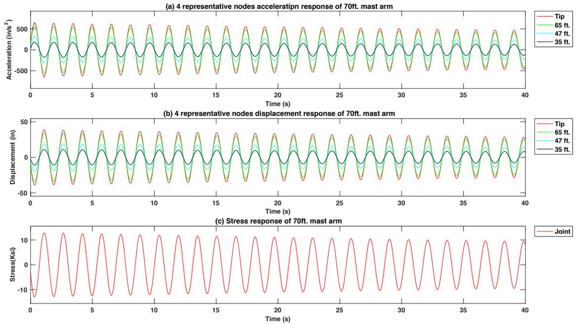
**Figure 4-2 Free vibration response of the 70 ft. arm signal support structure model without TMD**
