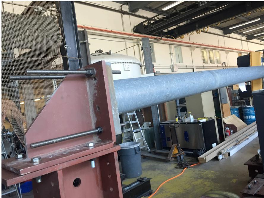
**Figure 5-2 Boundary condition for the mast arm**
