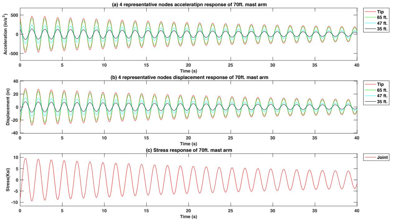
Figure 4-21 Free vibration response of excitation force at tip in the first mode frequency of the 70ft. mast arm signal pole structure model with 15 lb. mass TMD using the  $f_d = 0.5 f_n$
