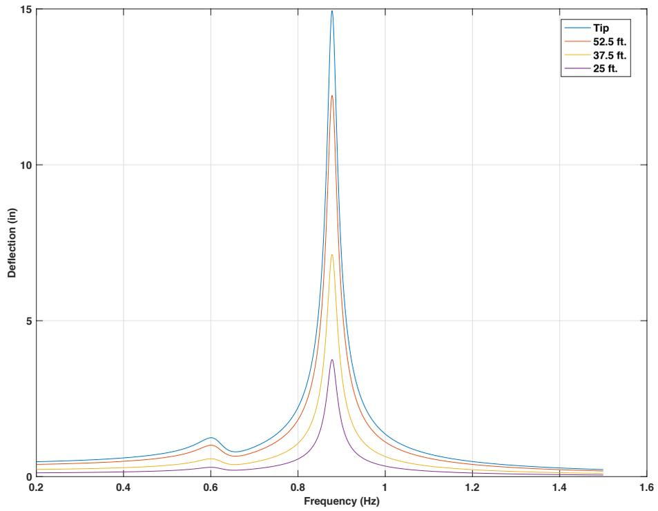
Figure 4-87 Frequency response for 60ft. mast arm with 15lb mass TMD, 5 lbf force on 3 signal heads location,  $f_d = 0.75 f_n$
