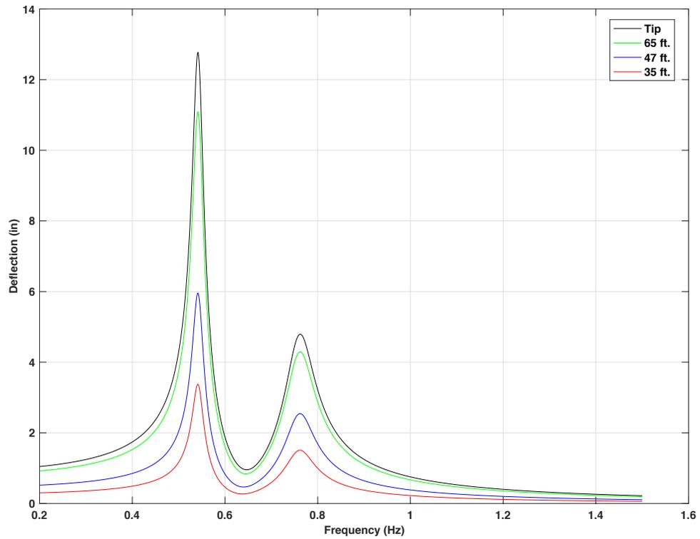
**Figure 4-20 Frequency response for 70ft. mast arm with 25lb mass TMD, force on signal heads' location**
