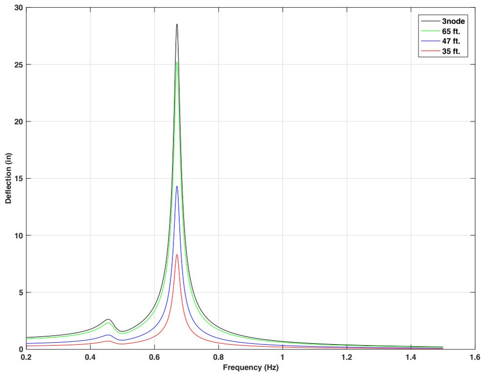
Figure 4-34 Frequency response for 70ft. mast arm with 15lb mass TMD, 5 lbf force on 3 signal heads location,  $f_d = 0.75 f_n$ , (notation 3node means tip deflection under this situation)
