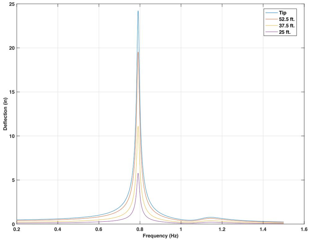
Figure 4-93 Frequency response for 60ft. mast arm with 15lb mass TMD, 5 lbf force on 3 signal heads location,  $f_d = 1.25 f_n$
