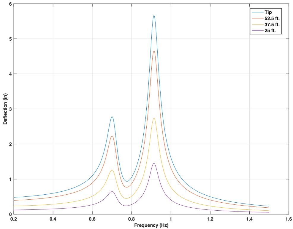
Figure 4-89 Frequency response for 60ft. mast arm with 15lb mass TMD, 5 lbf force on 3 signal heads location,  $f_d = 0.9 f_n$
