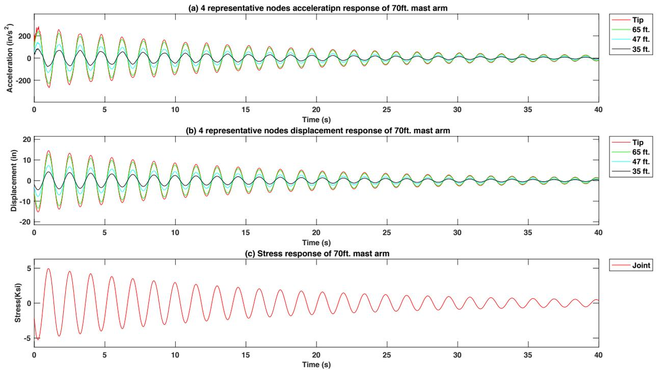
Figure 4-22 Free vibration response of excitation force at tip in natural frequency of the 70 ft. mast arm signal pole structure model with 15 lb. mass TMD using the  $f_d = 0.75 f_n$
