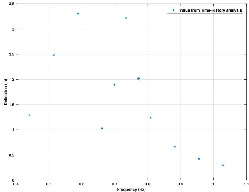
Figure 4-12 Peak value in steady state for different excitation force frequencies, 70ft. mast arm with 15lb mass TMD
