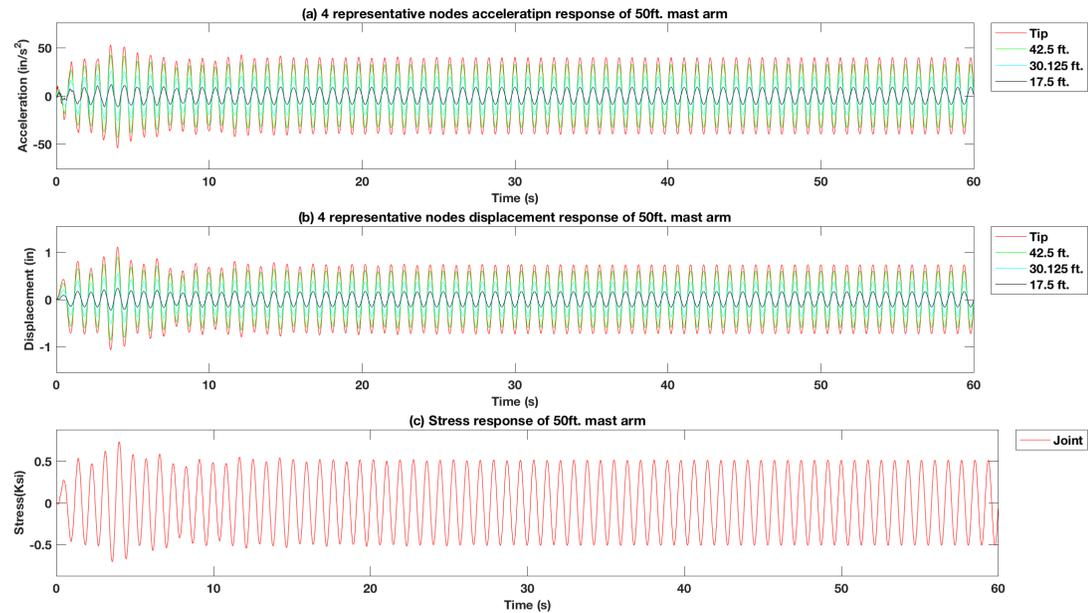
**Figure 4-116 Force vibration response of excitation force at tip of the 50 ft. mast arm signal pole structure model with 15 lb. mass TMD using the  $f_y = 1.1f_n$**
