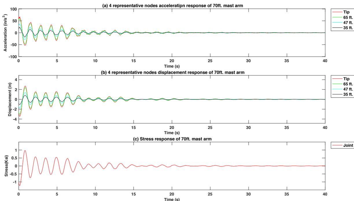
Figure 4-48 Free vibration response of excitation force at tip on the 70 ft. mast arm signal pole structure model with 15 lb. mass TMD at 5 ft from the tip
