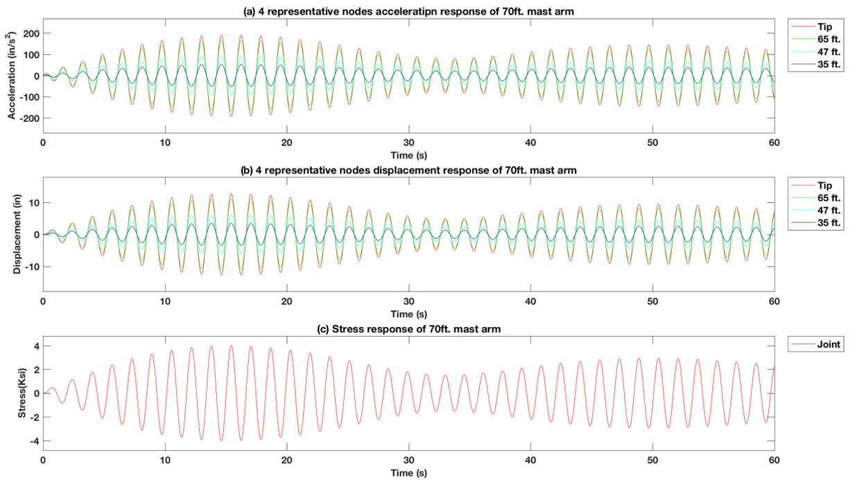
Figure 4-30 Force vibration response of excitation force at 3 signal heads position on the 70 ft. mast arm signal pole structure model with 15 lb. mass TMD using the  $f_d = 1.25 f_n$ ,  $f_y = 1.05 f_n$
