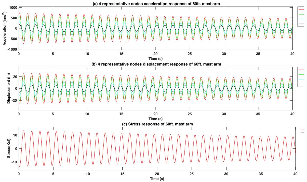
Figure 4-58 Free vibration response of the 60 ft. arm signal support structure model without TMD
