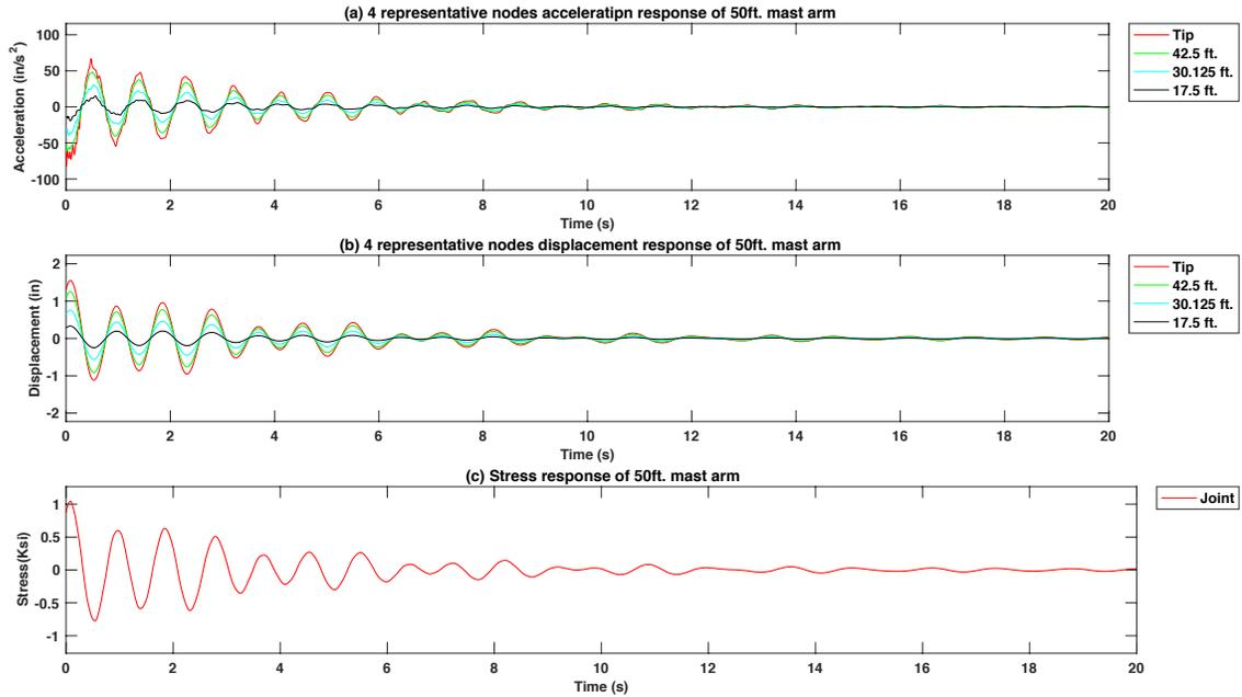
**Figure 4-115 Free vibration response of the 50 ft. arm signal support structure model with 25lb. TMD in the same frequency of the structure**
