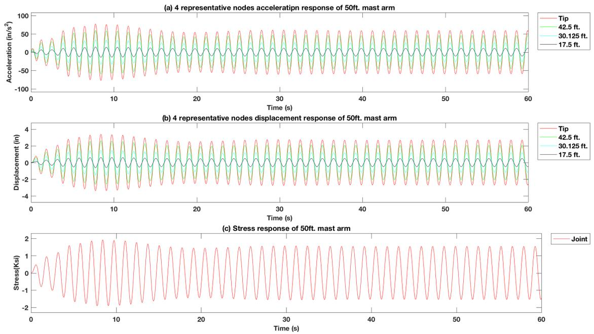
Figure 4-117 Force vibration response of excitation force at 3 signal heads location of the 50 ft. mast arm signal pole structure model with 15 lb. mass TMD using the  $f_y = 0.7f_n$
