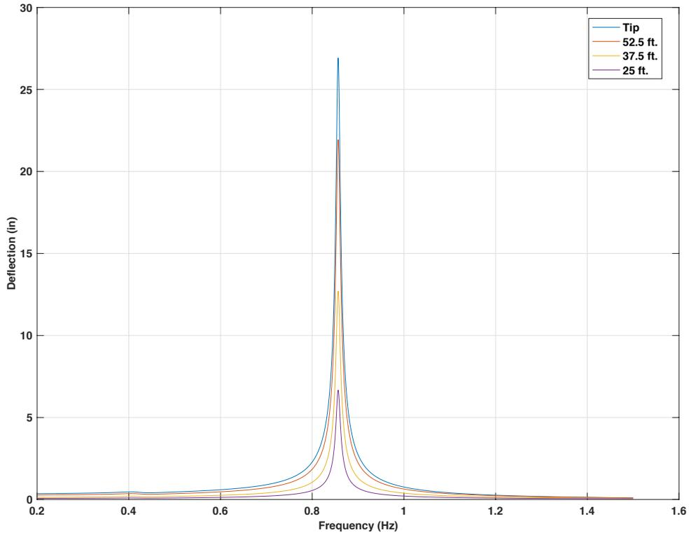
Figure 4-84 Frequency response for 60ft. mast arm with 15lb mass TMD, 5 lbf force on tip,  $f_d = 0.5 f_n$
