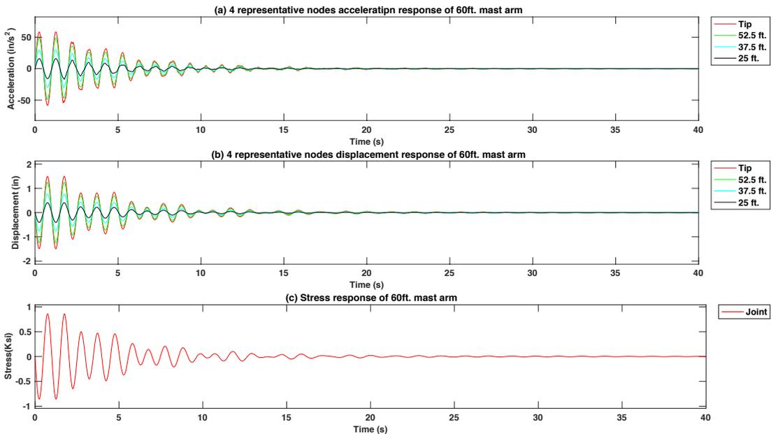
**Figure 4-64 Free vibration response of the 60 ft. arm signal support structure model with 25lb. TMD in the same frequency of the structure**
