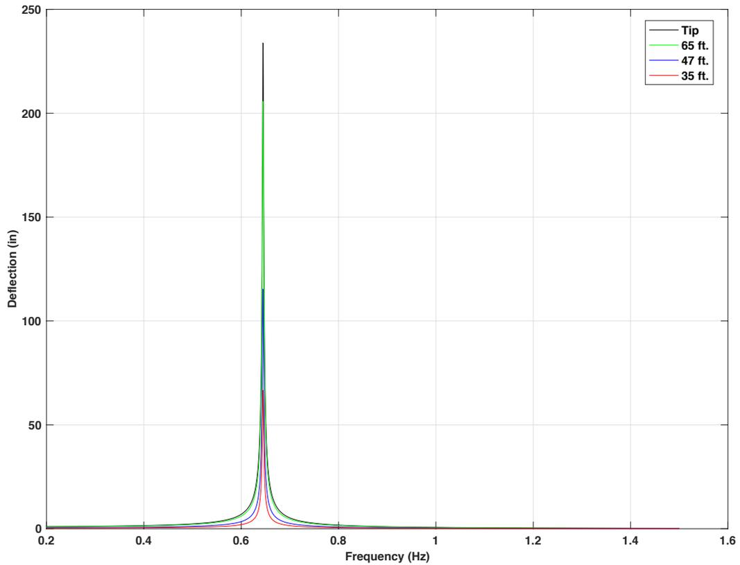
Figure 4-62 Harmonic response for excitation force on the mast arm signal heads locations of the 60 ft. arm signal support structure model without TMD
