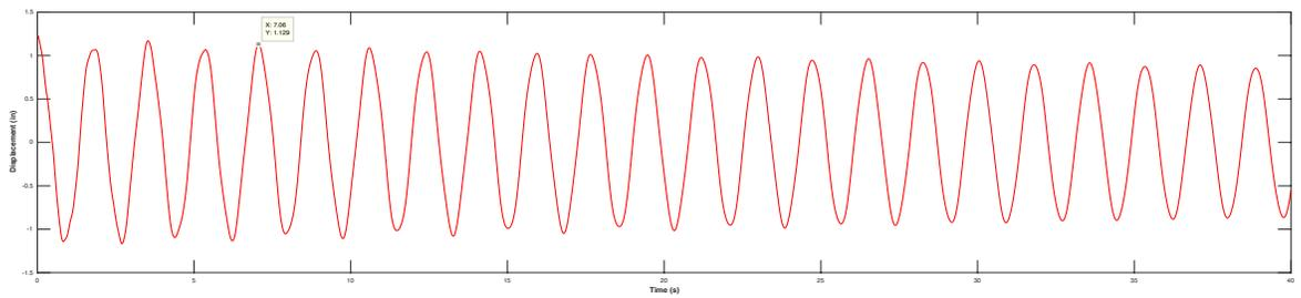
**Figure 3-6 Free vibration displacement response using ANSYS model with lumped mass**
