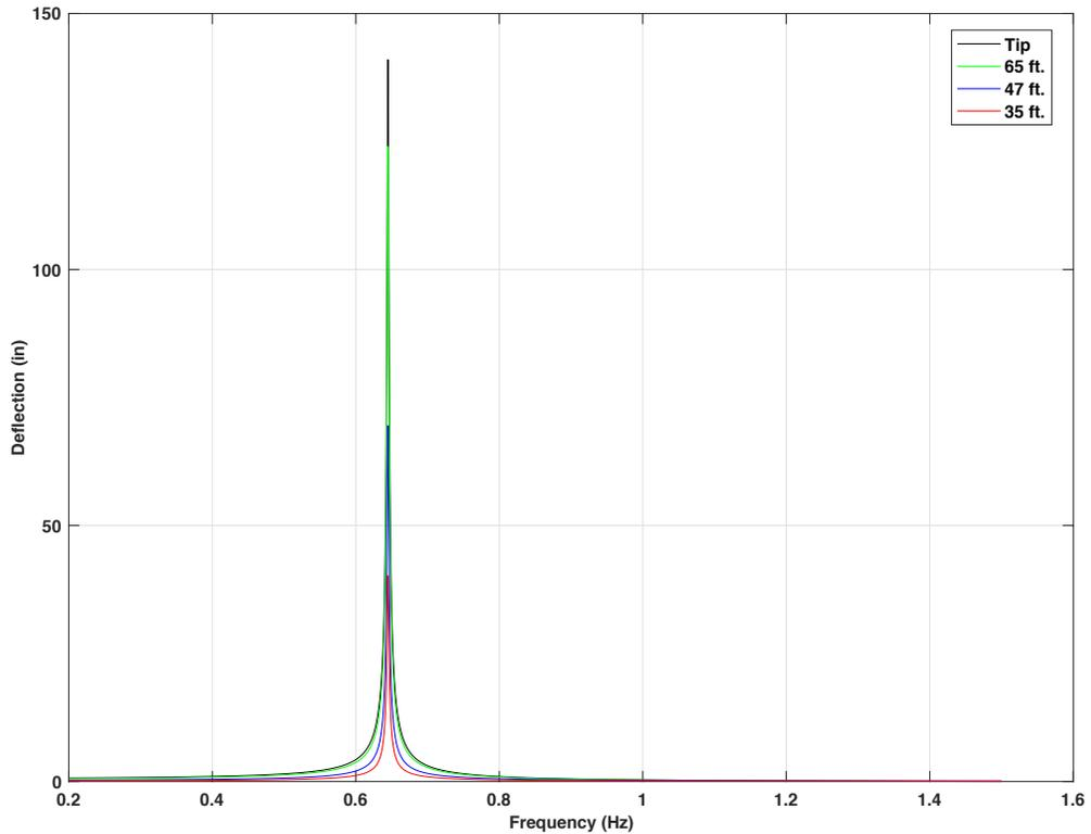
**Figure 4-61 Harmonic response for excitation force on the mast arm tip of the 60 ft. arm signal support structure model without TMD**
