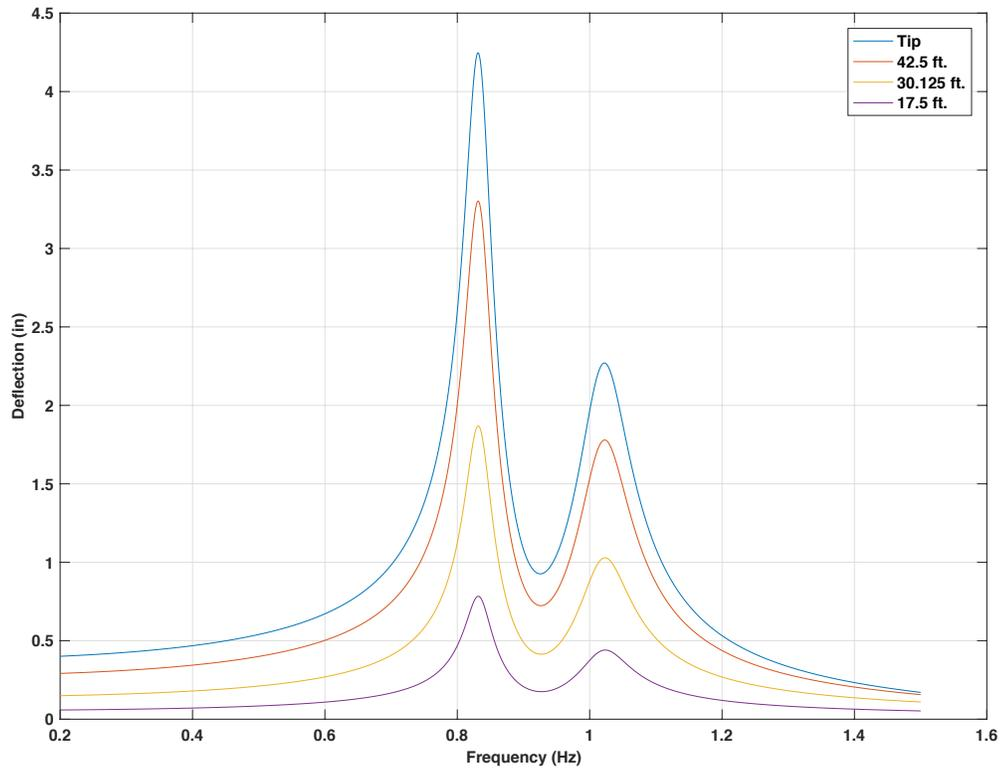
Figure 4-155 Frequency response for 50ft. mast arm with 15 lb. mass TMD at 5 ft from the tip
