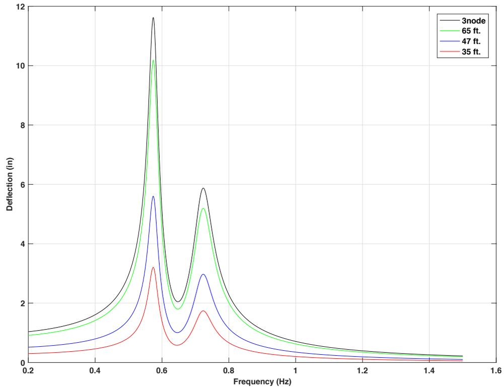
Figure 4-55 Frequency response for 70ft. mast arm with 15 lb. mass TMD at 5 ft from the tip,
