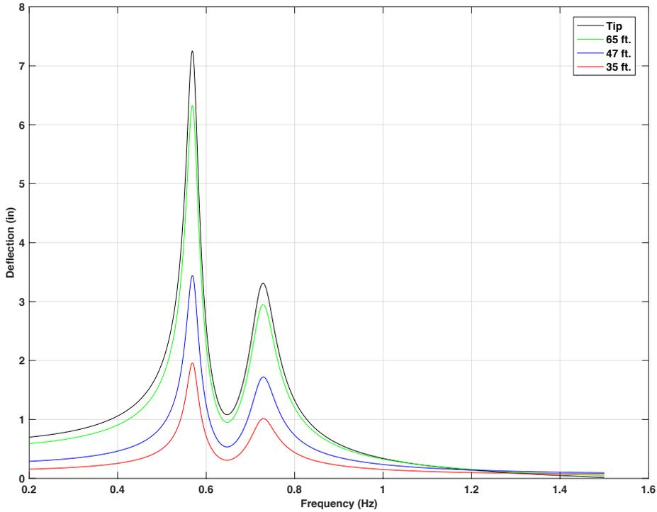
Figure 4-52 Frequency response for 70ft. mast arm with 15 lb. mass TMD at 2.5 ft from the tip  $f_d = 1.0 f_n$  5 lbf force on tip of mast arm
