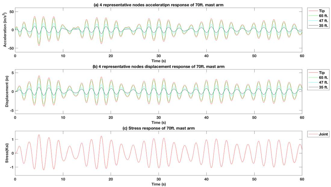
**Figure 4-45 Force vibration response of excitation force at 3 signal heads position on the 70 ft. mast arm signal pole structure model with 25 lb. mass TMD using the  $\zeta = 1\%$ ,  $f_s = 0.6f_n$**
