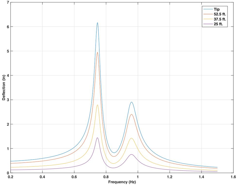
Figure 4-68 Frequency response for 60ft. mast arm with 15lb mass TMD, force on signal heads' location
