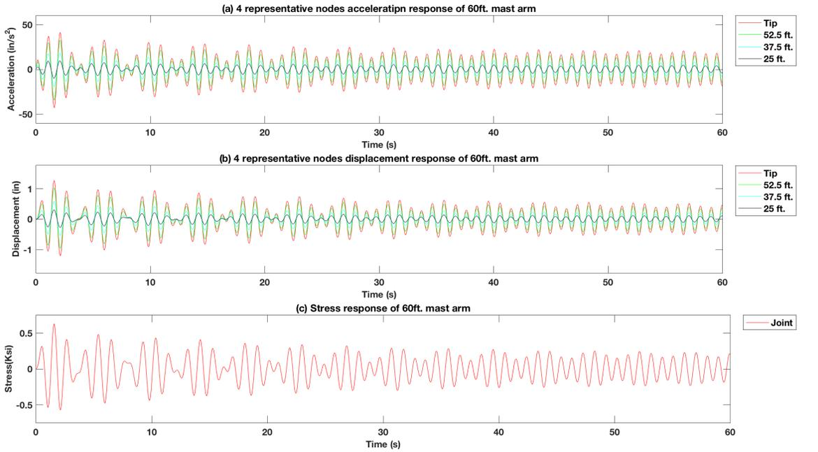
**Figure 4-82 Force vibration response of excitation force at 3 signal heads location of the 60 ft. mast arm signal pole structure model with 15 lb. mass TMD using the  $f_d = 1.25 f_n$ ,  $f_y = 1.3 f_n$**
