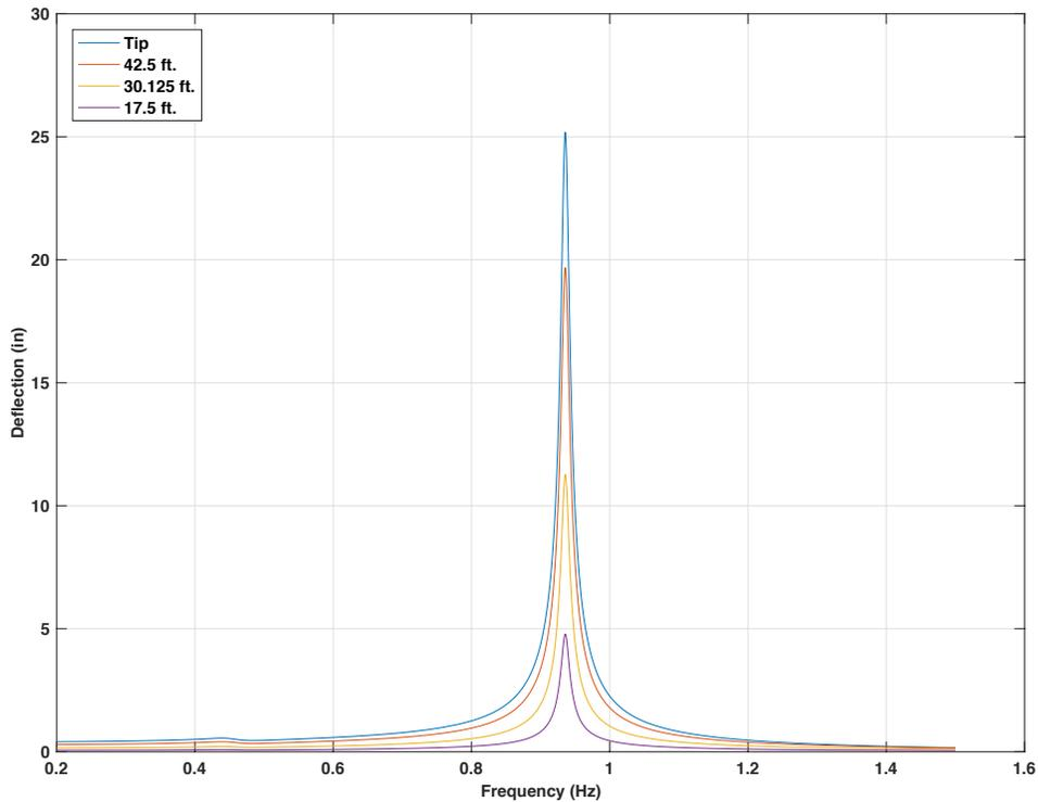
Figure 4-132 Frequency response for 50ft. mast arm with 15lb mass TMD, 5 lbf force on tip,
