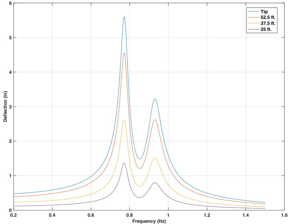
**Figure 4-109 Frequency response for 60ft. mast arm with 15 lb. mass TMD at 2.5 ft from the tip,  $f_d = 1.0f_n$ , 5 lbf force on 3 signal head location**
