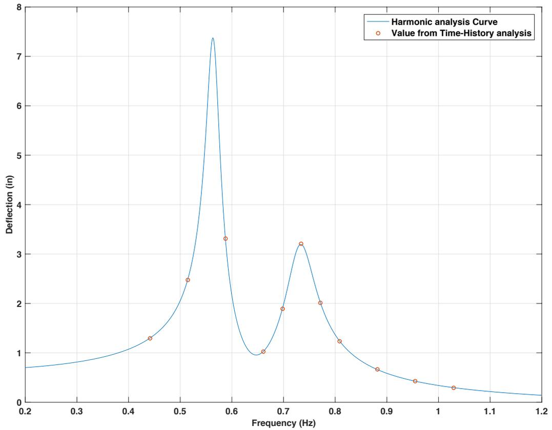
**Figure 4-14 Verification of results from force vibration response and harmonic analysis**
