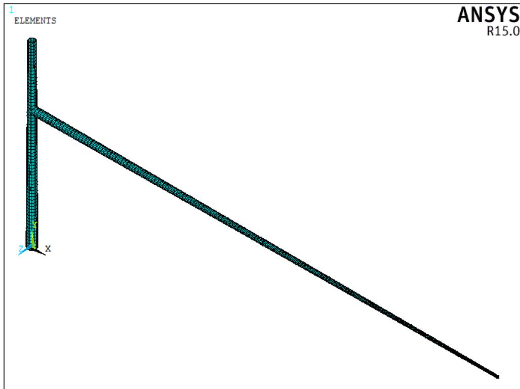
**Figure 3-3 Finite Element Model built in ANSYS for 70 ft. mast arm signal pole structure**
