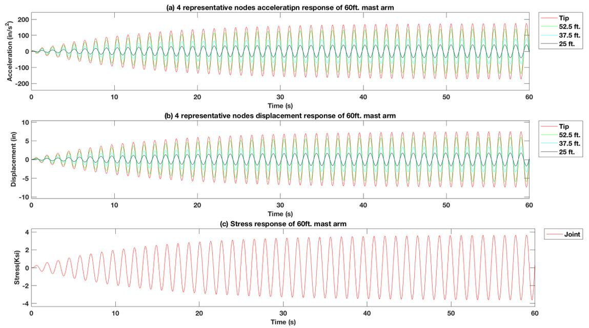
Figure 4-83 Force vibration response of excitation force at tip of the 60 ft. mast arm signal pole structure model with 15 lb. mass TMD using the  $f_d = 1.1 f_n$ ,  $f_x = 1.0 f_n$
