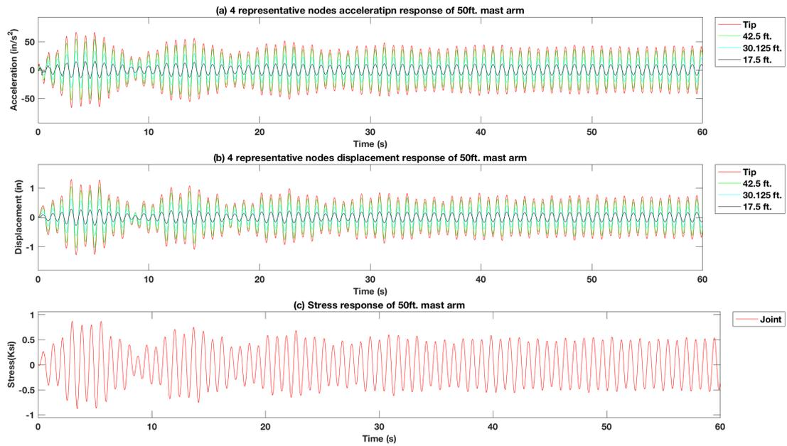
Figure 4-145 Force vibration response of excitation force at tip of the 50 ft. mast arm signal pole structure model with 25 lb. mass TMD using the  $\zeta = 1\%$ ,  $f_d = 1.1f_n$
