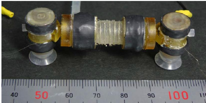
**Figure 2.22:** Inchworm Robot using Electro-conjugate Fluid [57]
