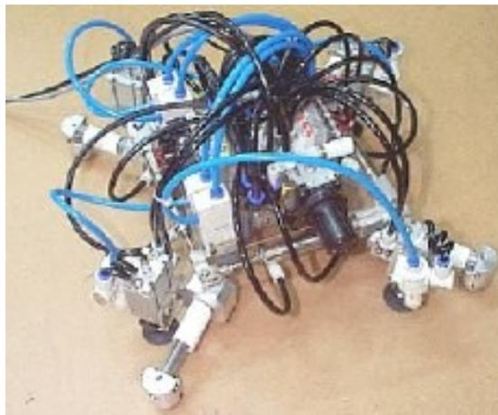
**Figure 2.18:** Planar Inchworm Robot: Planar Walker [50]
