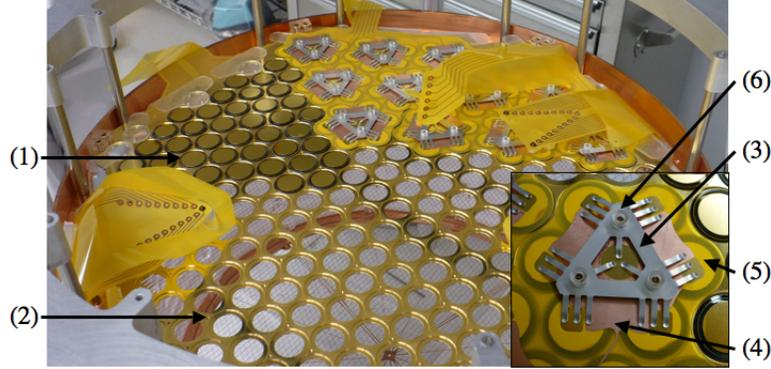
Figure 3.8: Bare LAAPDs (1) placed on a mounting platter (2); in the TPC, the side shown faces away from the drift region. Phosphor-bronze springs (3) anchor each gang of seven LAAPDs to the platter and make electrical contact between the cathodes of the APDs and the copper traces (4) on the flexible signal cabling (5). Acrylic washers (6) electrically decouple the springs from the platter, which is coupled to the anodes of the LAAPDs. From [47].
