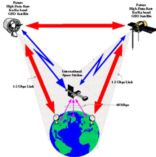
*Figure 2.1. Alternative communications architectures to/from the ISS*
