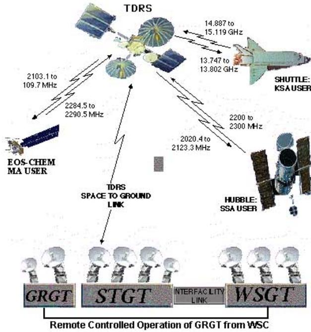
*Figure 2.2. Topology of NASA TDRSS.*
