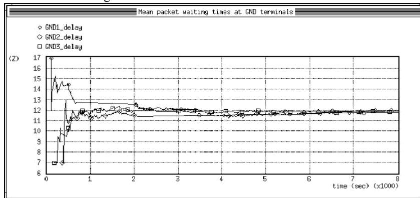
**Fig. 6 Average RX-Queueing Delay at GND stations**
