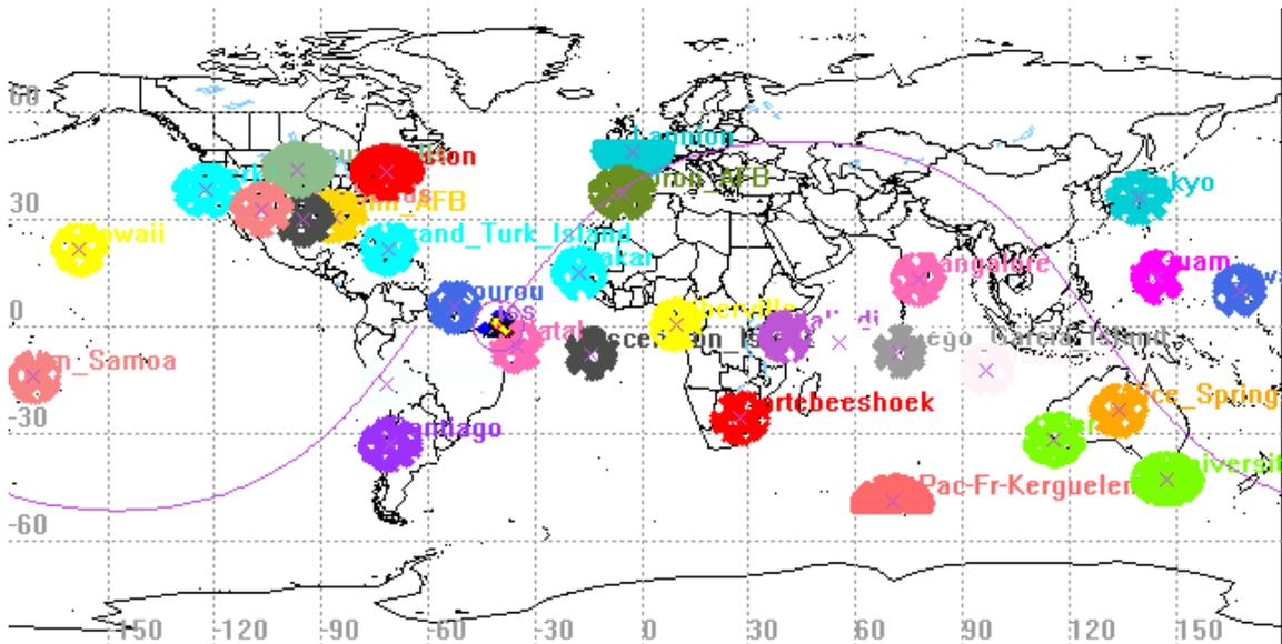
*Figure 4.1. Selection of stations for best coverage with 60 deg scan angle*
