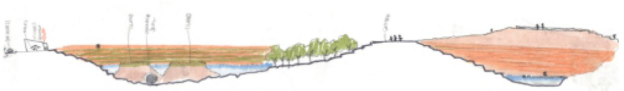
**Figure 20: Section Sketch illustrating the saddle that divides the site, the drainage pipe in the southern gorge and the ephemeral island concept.**
