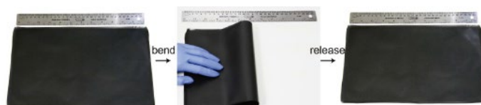
Figure 1.16 Photographs showing the graphite-NFC film retain morphology before and after bending.
