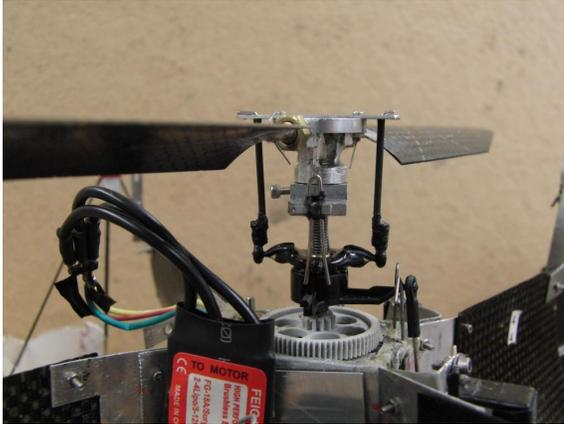
Figure 5.49: Swashplate with cyclic travel of  $\pm 10^\circ$
