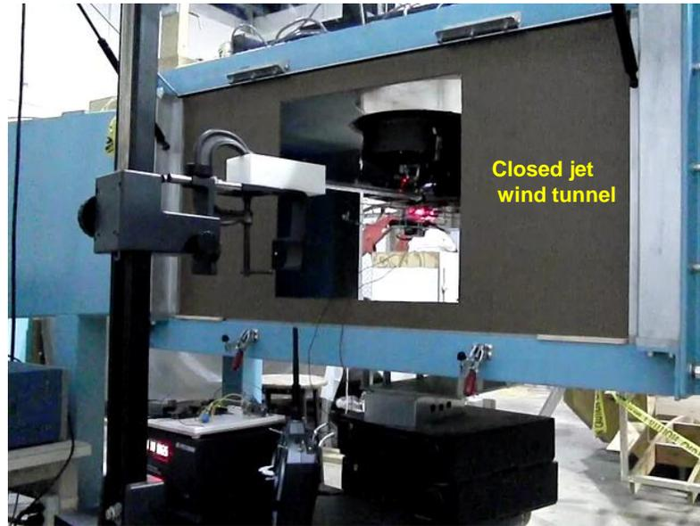
Figure 6.12: Closed jet wind tunnel set-up
