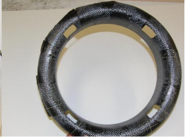
Figure 5.33: Shroud vent design
