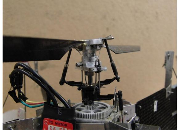
Figure 5.50: Swashplate with cyclic travel of  $\pm 15^\circ$
