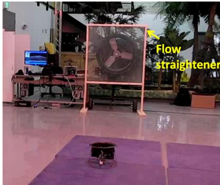
Figure 6.29: 0.75 m diameter fan gust setup
