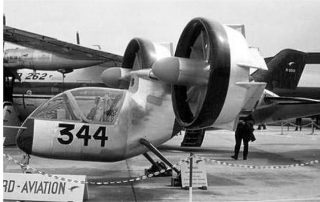
Figure 1.12: Nord 500 Cadet tilt-duct aircraft
