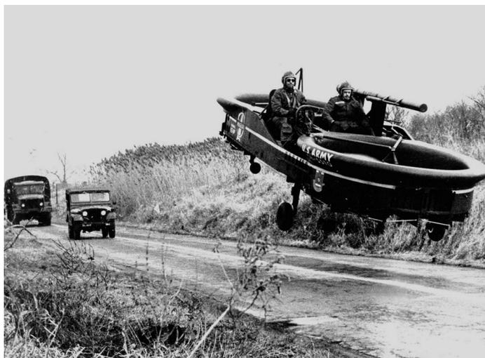
Figure 1.16: Piasecki Airgeep in forward flight
