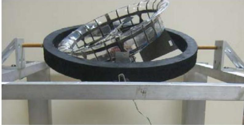
Figure 3.38: Vehicle mounted on gimbal to test pitch/roll control
