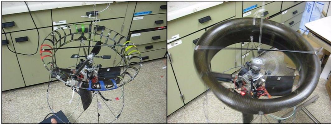
Figure 3.7: Suspended unshrouded and shrouded rotor vehicles
