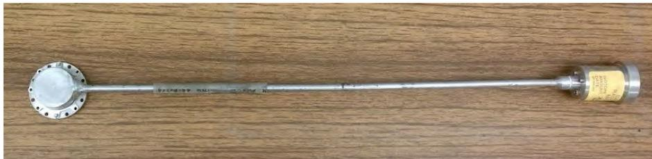
**Figure 6.1-1: NIST-calibrated fission chamber beam monitor [54].**
