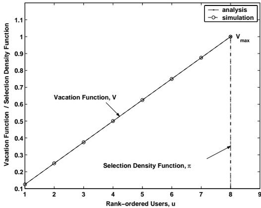
Fig. 4. LWF Scheduler :  $V$  and  $\pi$  for  $\alpha = 1000$
