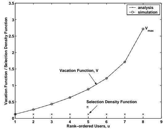
Fig. 5. Maximum SNR Scheduler :  $V$  and  $\pi$  for  $\alpha = 0$
