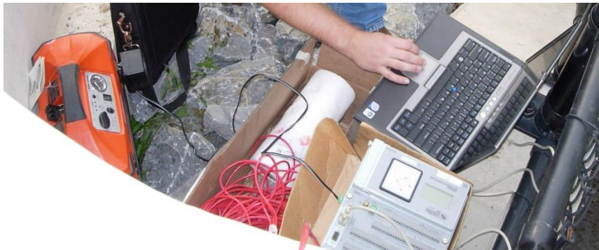
Figure 3-12: Data Acquisition System Monitoring the Strain Gauges During the Live Load Test.
