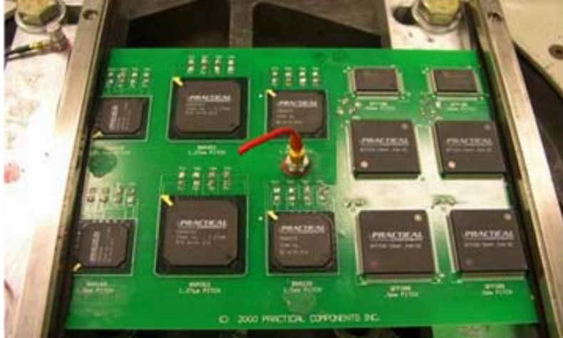
Figure 21. Test board mounted on the vibration shaker
