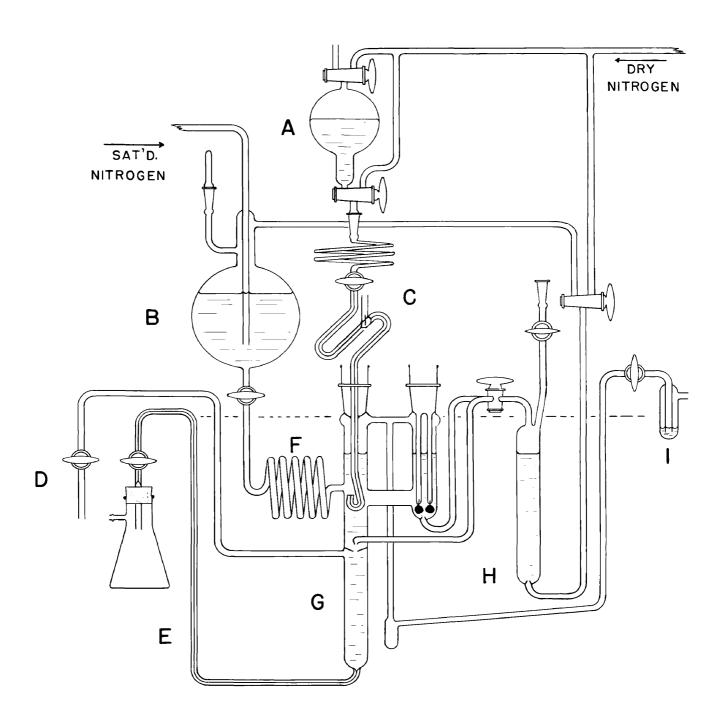
Figure III. Aqueous cell and auxiliary apparatus
