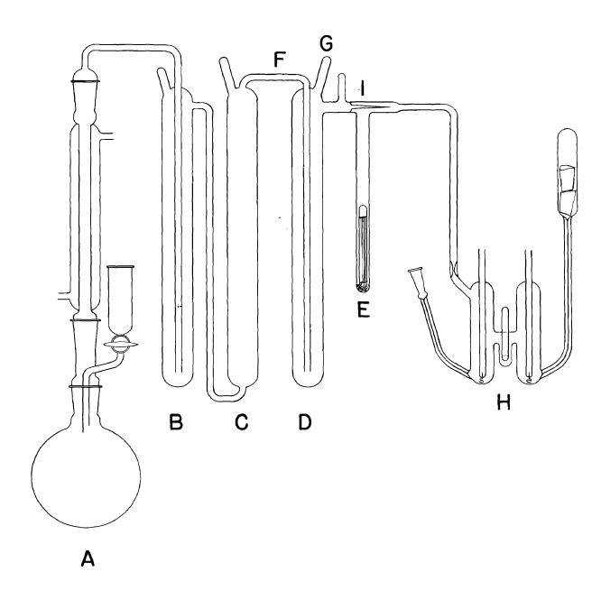
Figure II. Non-aqueous cell and auxiliary apparatus
