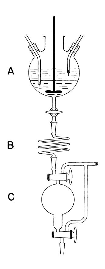
Figure I. Apparatus for preparation of smalgams
