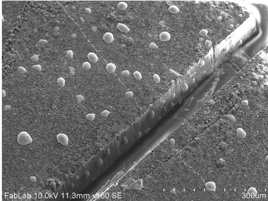
Figure 2.15: SEM image of droplets that formed on the Ag/PDMS sensor after being released from the silicon mold via xenon difluoride. The droplets were found to be hydrofluoric acid via a litmus test and EDS, and has also been seen in other work [6].
