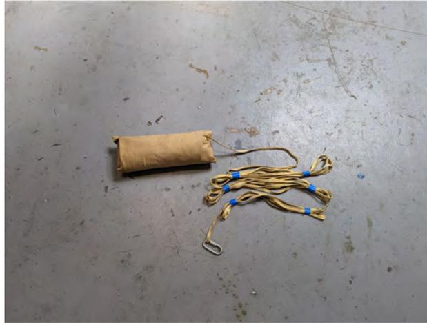
**Fig. 47 Main parachute wrapped in nomex with lines Z-folded**
