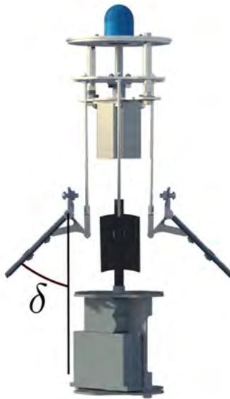
**Fig. 74**  $\delta$  is defined as the flap deployment angle
