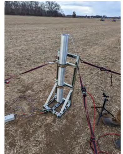
Motor #2 secured in test stand
