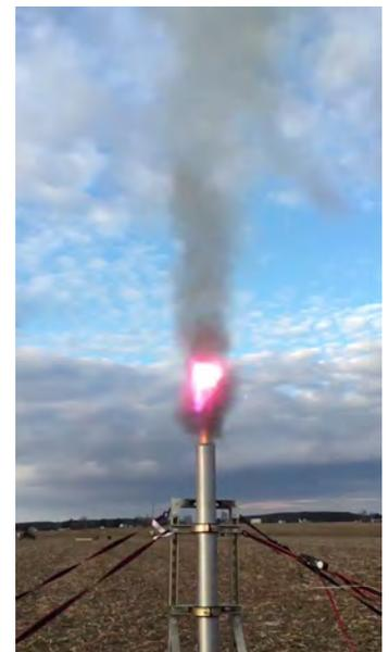
Motor #2 ejecting a casting tube during static test
