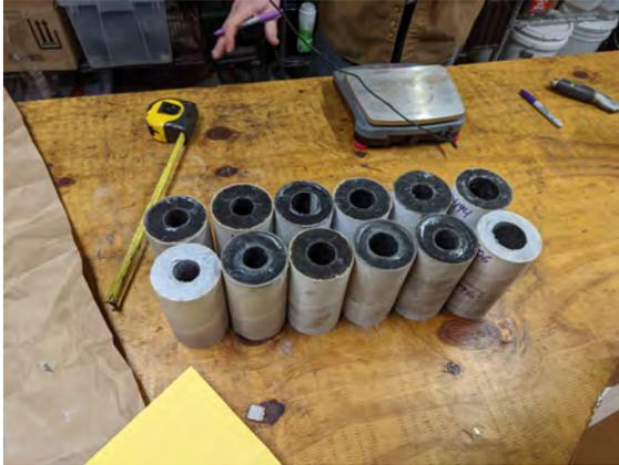
**Fig. 14 Cut Motor Grains**
