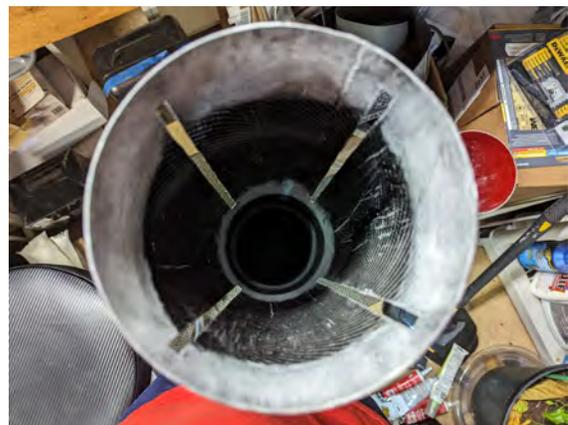
**Fig. 38** Inner diameter of the airframe is sanded for motor mount bonding
