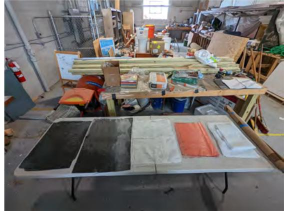
**Fig. 30** Carbon, peel ply, release film, and breather prepared
