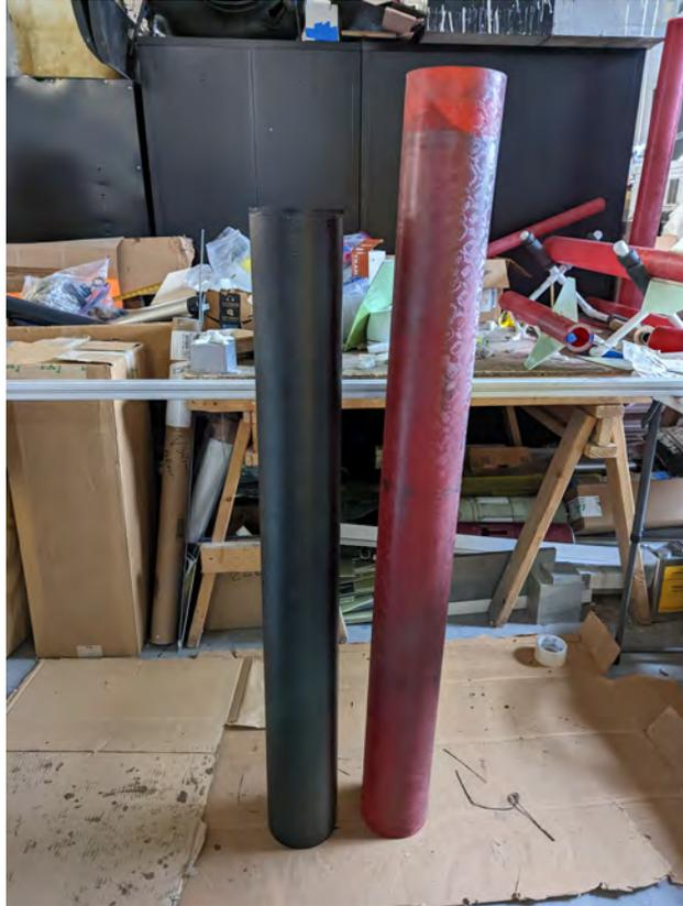
**Fig. 26 Carbon tube after removal from mandrel**
