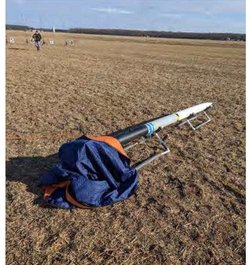
Karkinos set up for ejection testing
