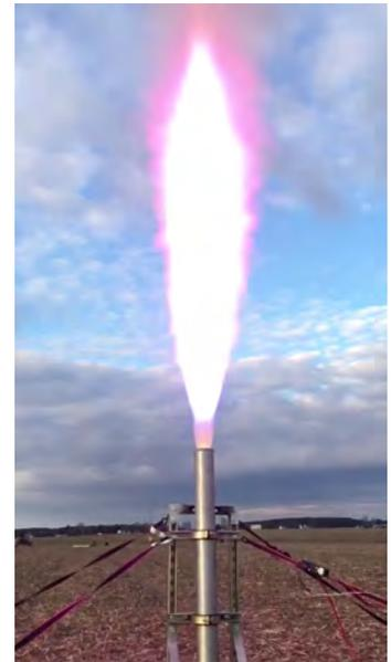
Motor #2 during static test
