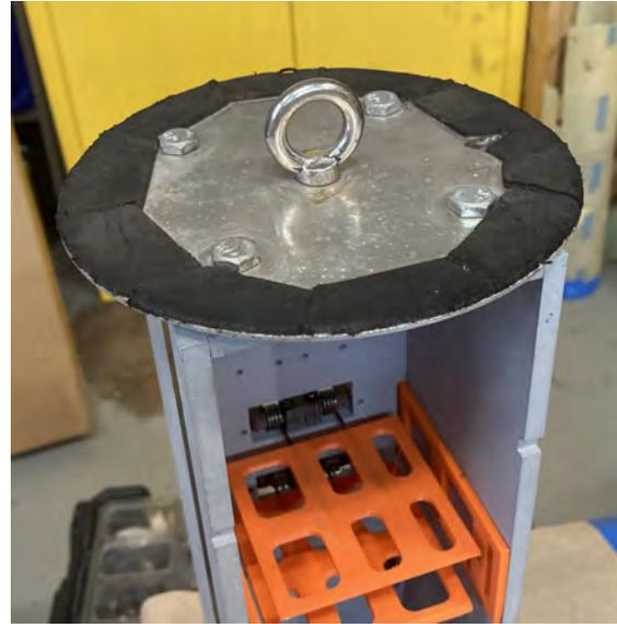
**Fig. 100** Top bulkhead mounted to the release system
