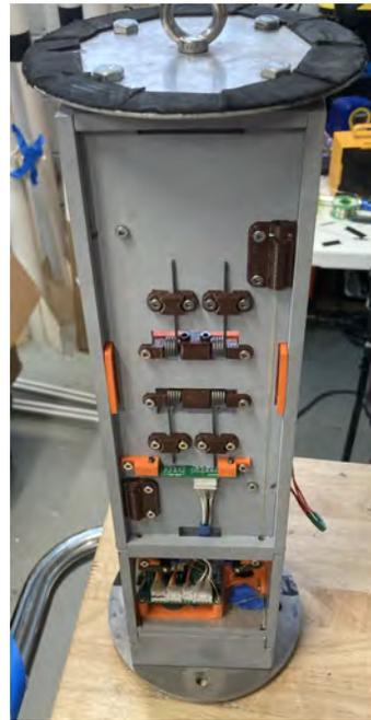
**Fig. 90** Backside of the payload assembly and connecting bulkheads, with Ebay cover panel removed
