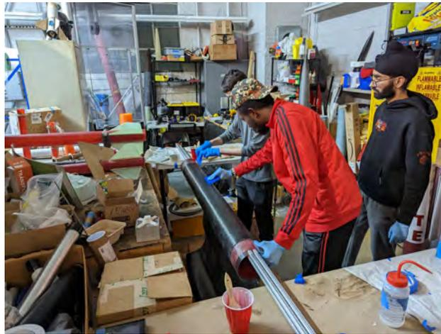
**Fig. 25 Layup of carbon fiber airframe**
