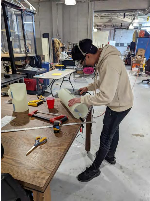
**Fig. 62** Cutting airframe from coupler
