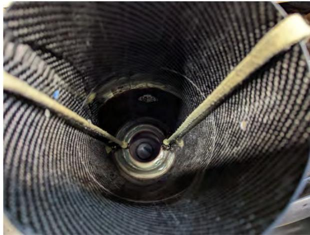
**Fig. 49 Y harness mount in fin can**
