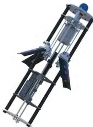
**Fig. 58 Internal CAD of the Air Brake module.**
