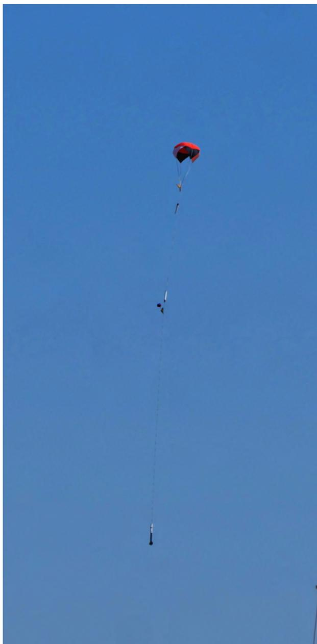
**Fig. 48 Karkinos descending under its main parachute**
