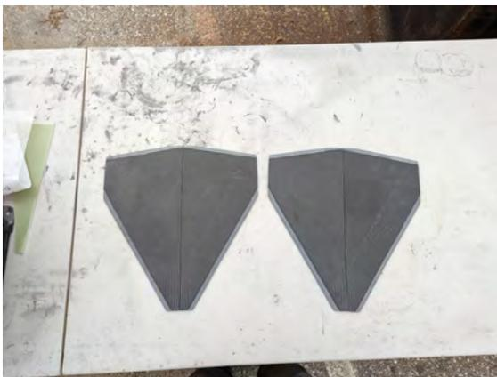
**Fig. 34 Fins after bevelling on router**
