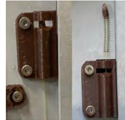
**Fig. 91 Pin release system. Left: Pin in standard configuration. Right: Pin mechanism exploded**
