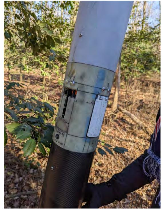
Missing airbrake after flight
