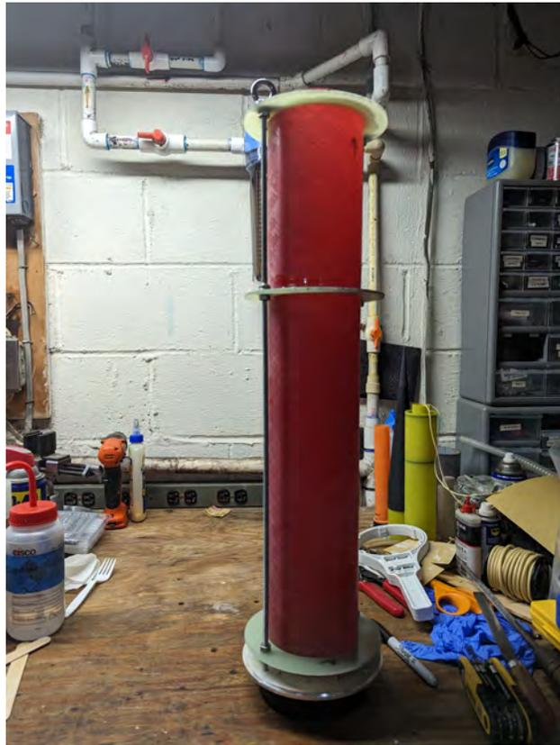
**Fig. 36** Motor mount assembly with forward two centering rings epoxied on
