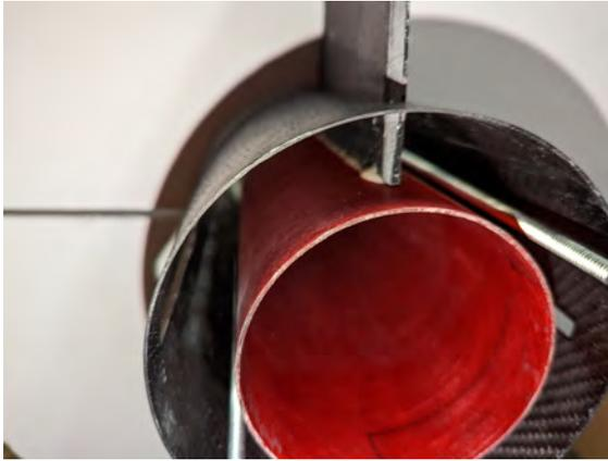
**Fig. 39** A small fillet is formed when the fin is tacked
