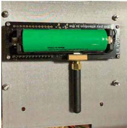
Back of the sled with the radio module mounted
