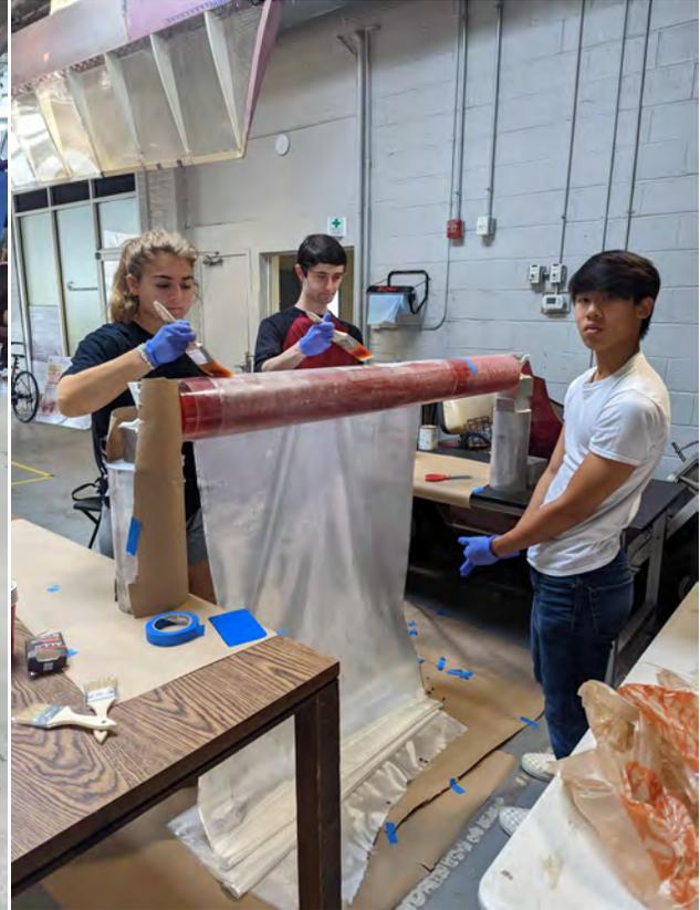
**Fig. 63** Rolling of fiberglass and epoxy resin
