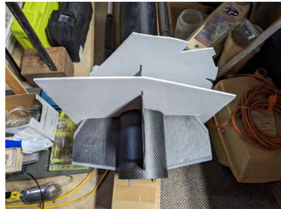
**Fig. 40** All fins tacked on with fin guides
