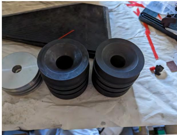
**Fig. 7 Nozzles and Forward Closure**
