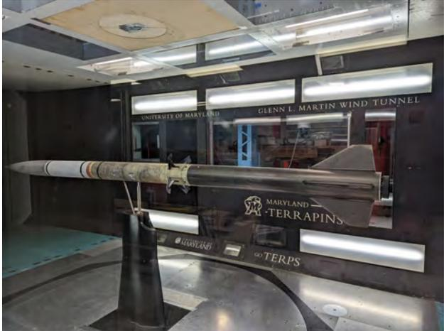
**Fig. 88** Karkinos mounted in the wind tunnel
