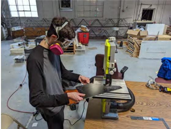
**Fig. 29** Cutting the rough shape of the fins on a bandsaw
