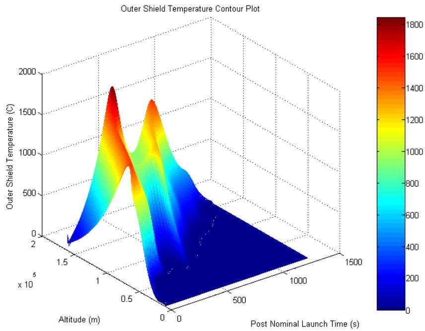
**Figure 5.8 Three Dimensional Mesh Plot of Shield Temperature vs Altitude and Time**
