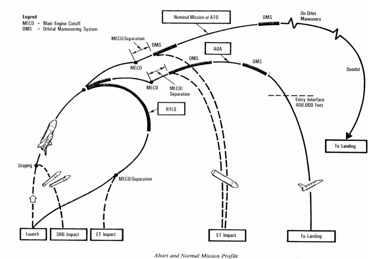
**Figure 2.5 Shuttle Intact Abort Modes [8]**
