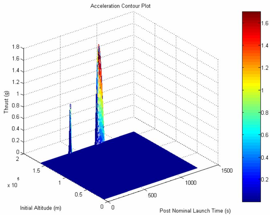
**Figure 5.10 Three Dimensional Mesh Plot of Required Thrust vs Altitude and Time with Maximum Acceleration set to 8 g's**
