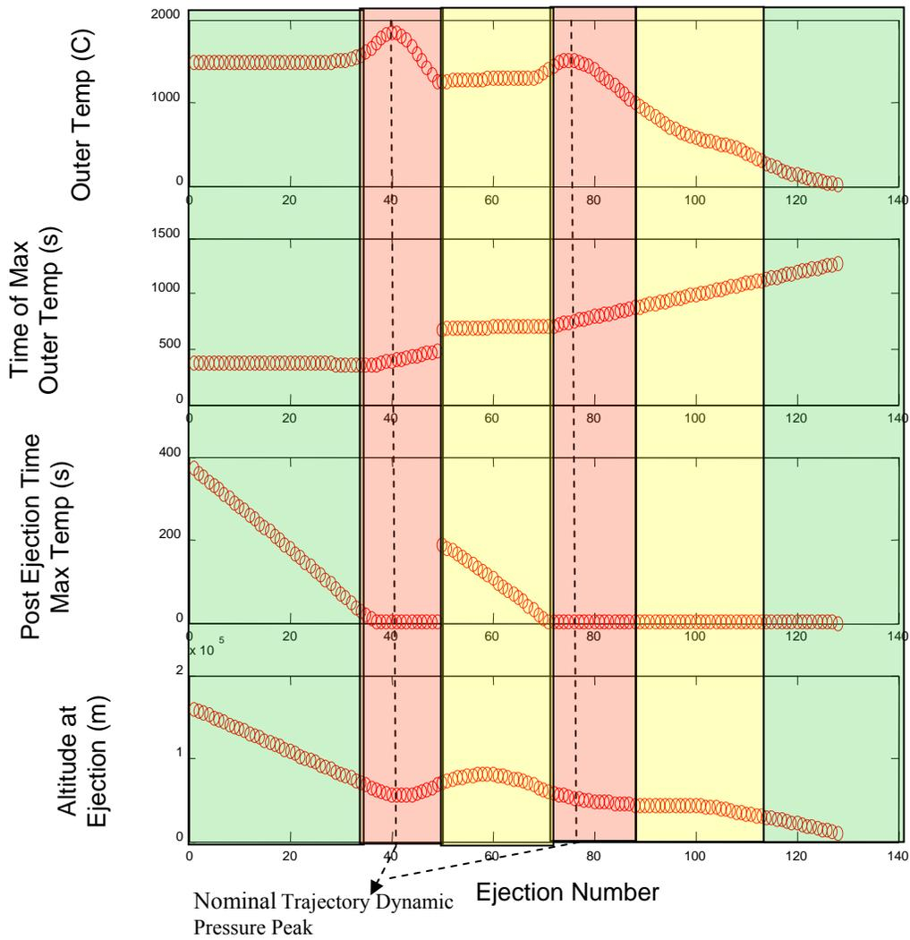
Figure 5.14 Temperature Based Ejection Zones. Zone 1 is Green, Zone 2 is Yellow and Zone 3 is Red
