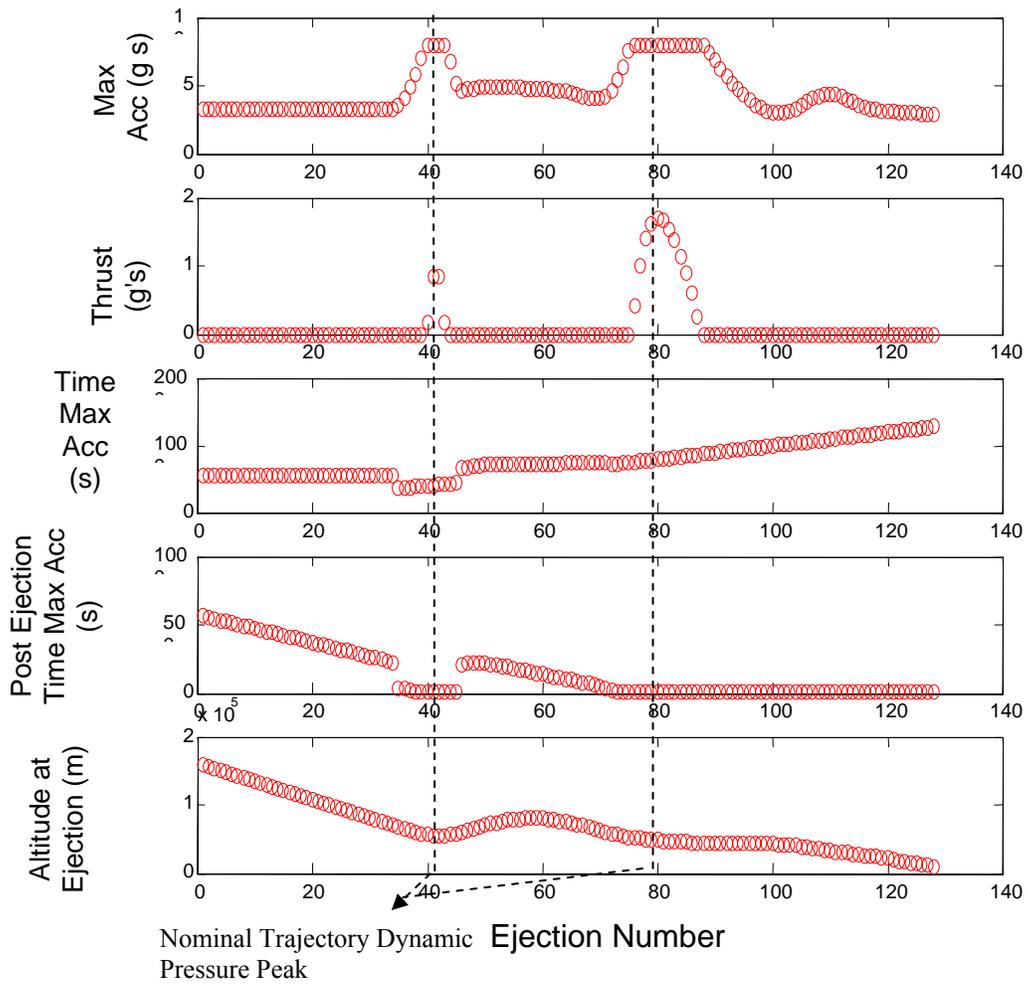
Figure 5.11 Worst Acceleration Occurrence Per Ejection Trajectory
