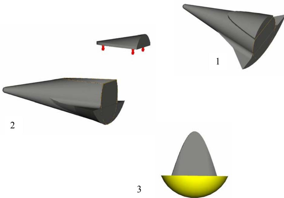
**Figure 1.1 Conceptual Escape Sequence. 1. Lifeboat begins attached to nominal vehicle. 2. Lifeboat ejects from nominal Vehicle during emergency. 3. Lifeboat deploys heatshield to continue reentry away from doomed nominal vehicle**
