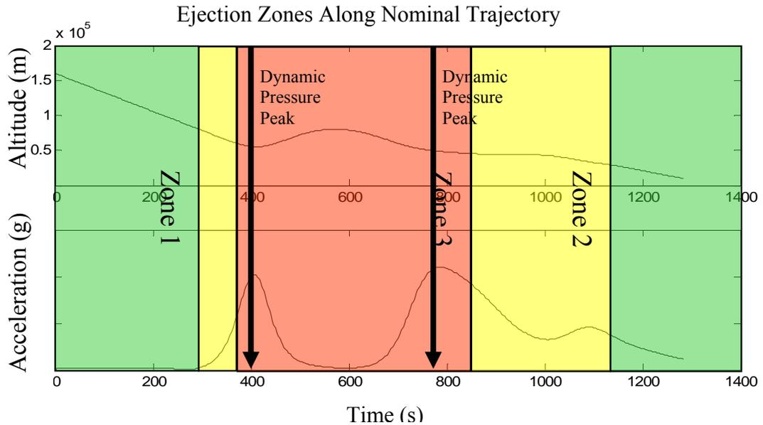
**Figure 4.2 Defined Ejection Zones Along Nominal Vehicle's Entry Trajectory**
