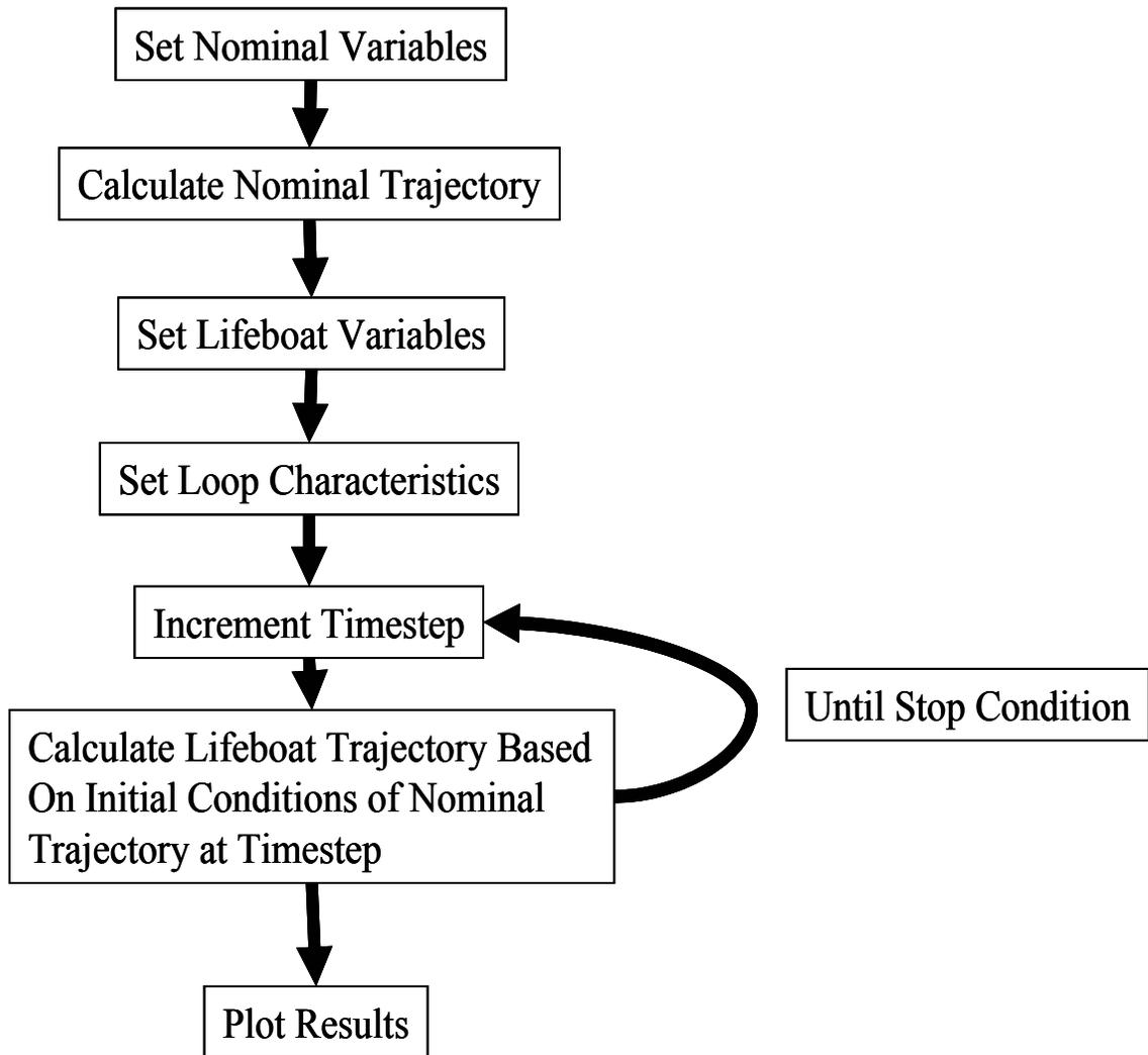
Figure 4.4 Algorithm used in computer simulation
