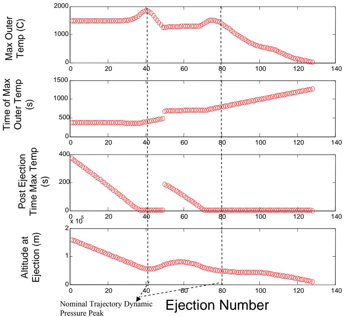
Figure 5.12 Worst Temperature Occurrence Per Ejection Trajectory
