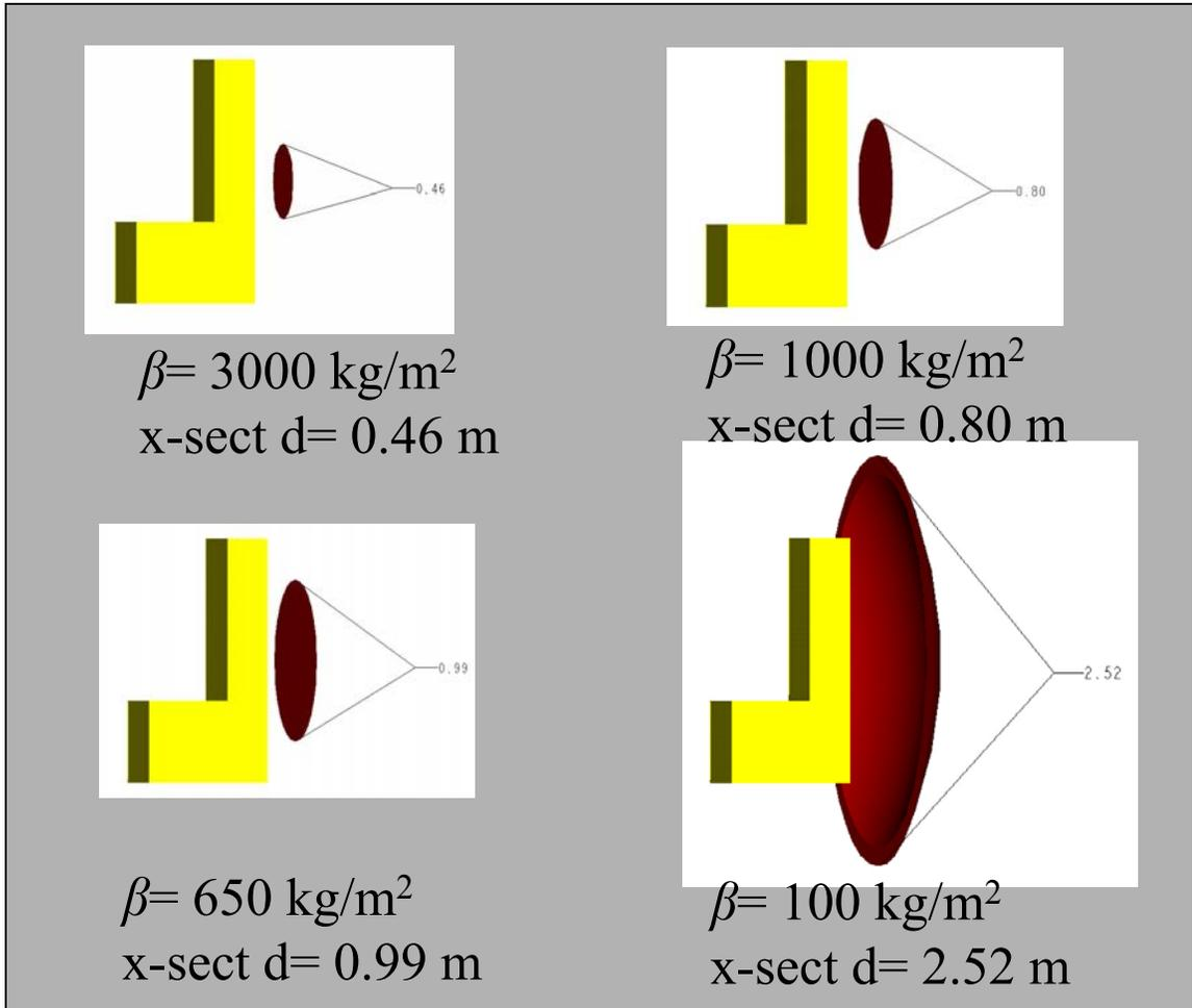
**Figure 5.4 Heat Shield Sizes for 1000 kg Lifeboat with varying ballistic coefficients. Couch dimensions are 1.5 m tall by .5 m wide.**
