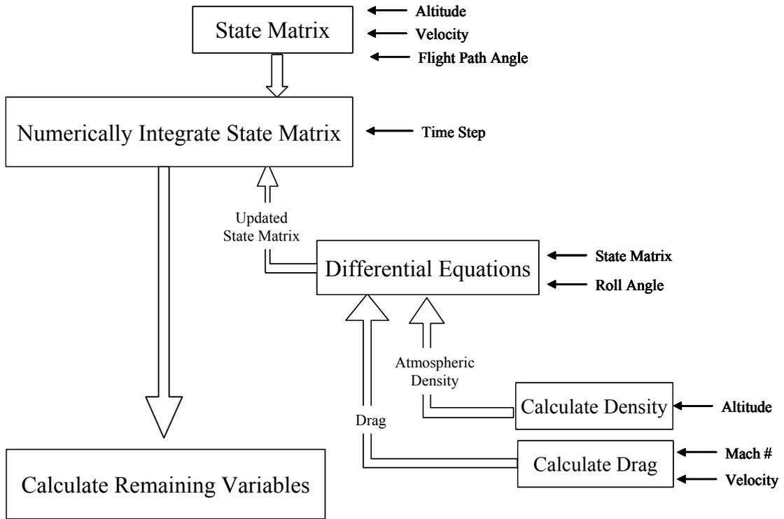
Figure 4.3 Algorithm used for Trajectory Calculations
