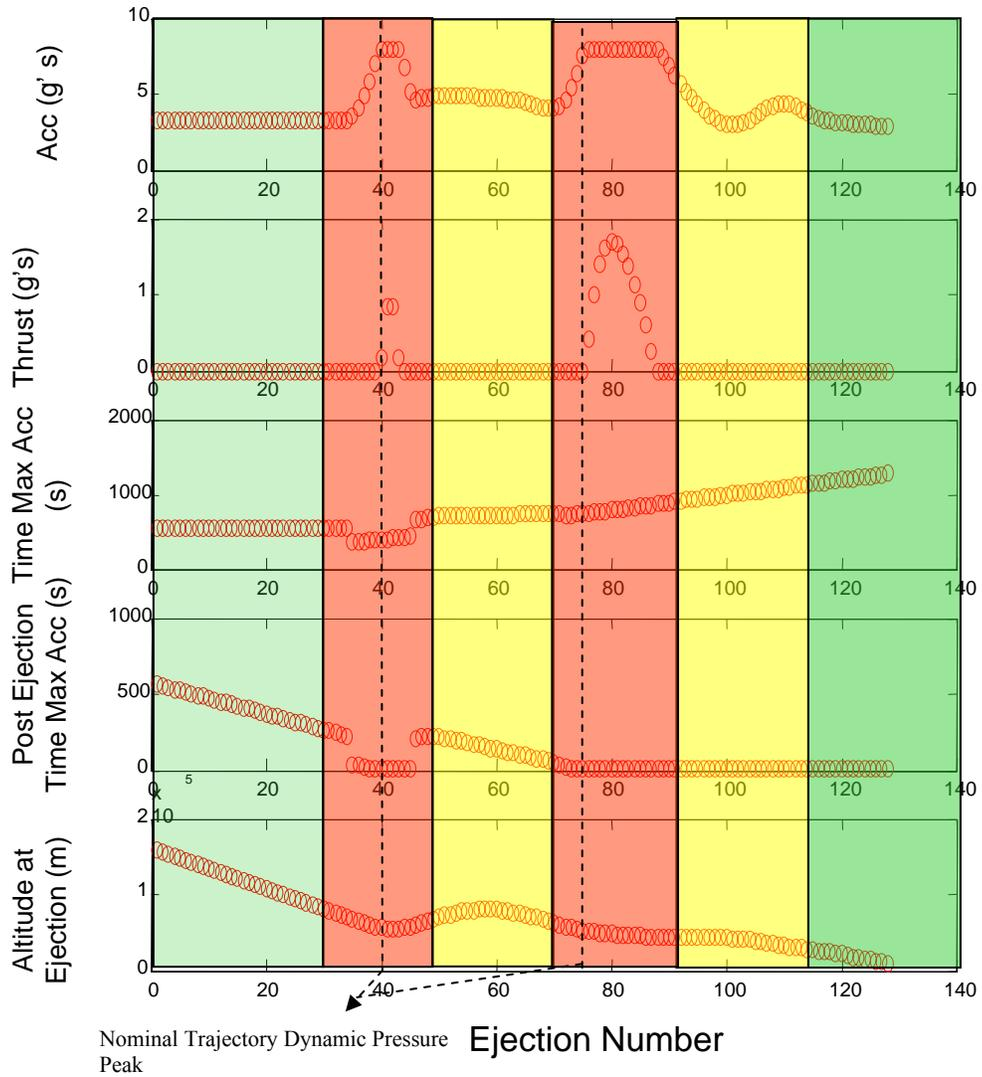
Figure 5.13 Acceleration Based Ejection Zones. Zone 1 is Green, Zone 2 is Yellow and Zone 3 is Red
