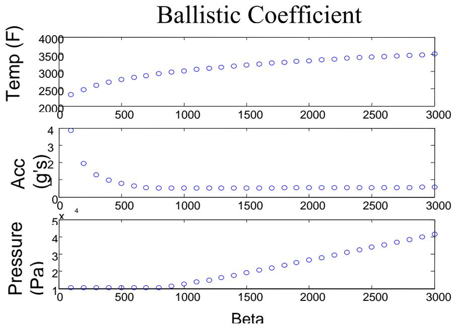
Figure 5.5 Results of Optimum Ballistic Coefficient Search
