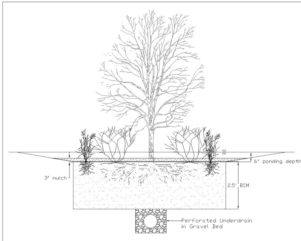
Figure 1.1: Schematic of a typical rain garden, consisting of a 2.5-foot-deep layer of bioretention soil medium (BSM), topped with a 3-inch layer of mulch, planted with a variety of native plants, shrubs and trees. The system is designed to allow a 6-inch ponding depth at the soil surface, and is often outfitted with an underdrain leading to a stormwater discharge.
