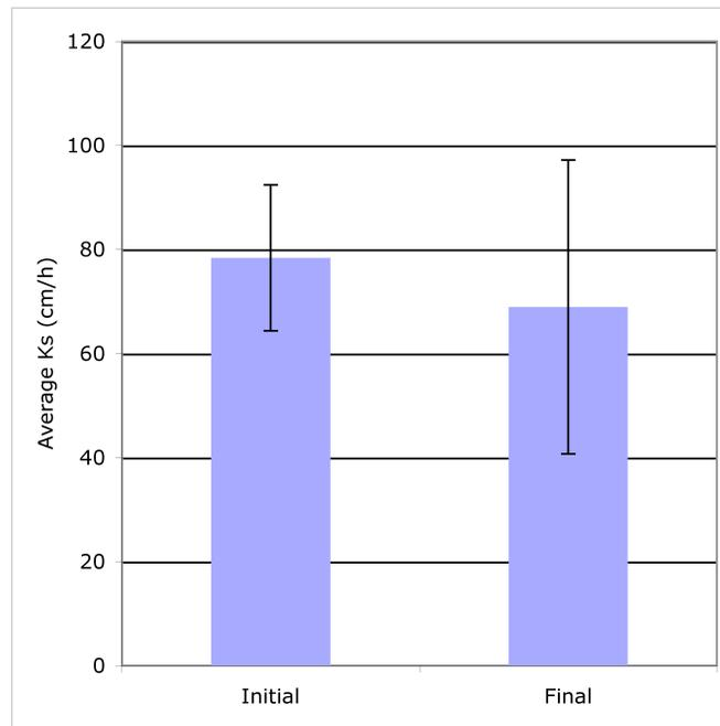
Figure 3.5: Average saturated hydraulic conductivity for Treatment 1 group. Error bars indicate the standard deviation from the mean. Average initial saturated hydraulic conductivity was  $78 \pm 14$  cm/h. Average final saturated hydraulic conductivity was  $69 \pm 28$  cm/h.
