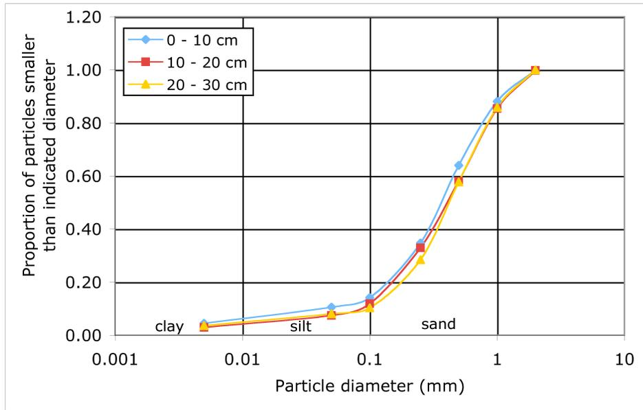
Figure 2.22: UMCP particle size distribution.
