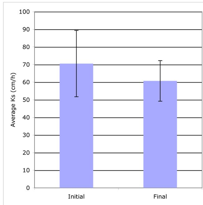
Figure 3.7: Average saturated hydraulic conductivity for Treatment 2 group. Error bars indicate the standard deviation from the mean. Average initial saturated hydraulic conductivity was  $71 \pm 19$  cm/h. Average final saturated hydraulic conductivity was  $61 \pm 12$  cm/h.
