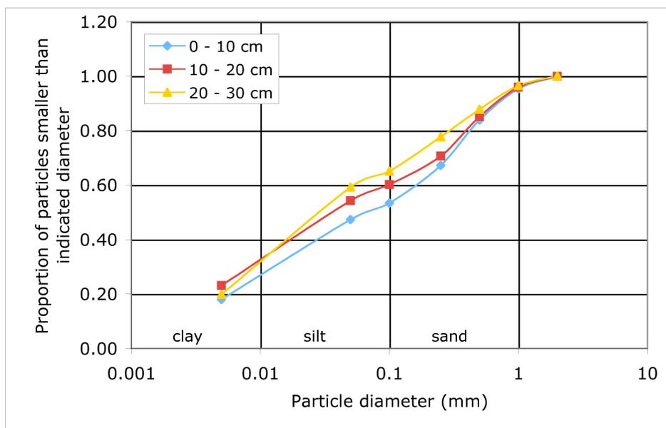
Figure 2.49: LRH particle size distribution.
