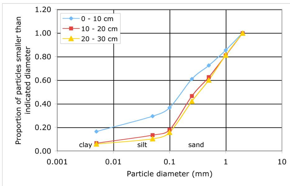
Figure 2.37: PP particle size distribution.
