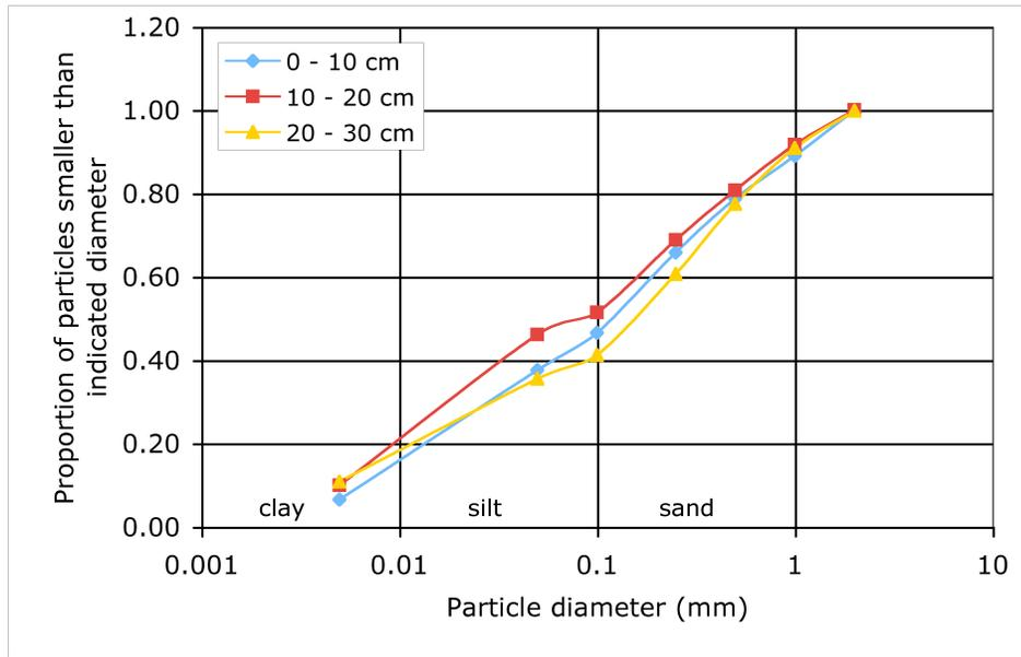
Figure 2.43: CC particle size distribution.
