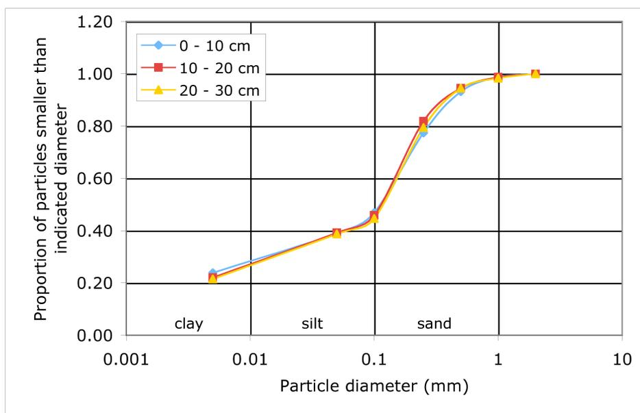
Figure 2.31: CBF particle size distribution.
