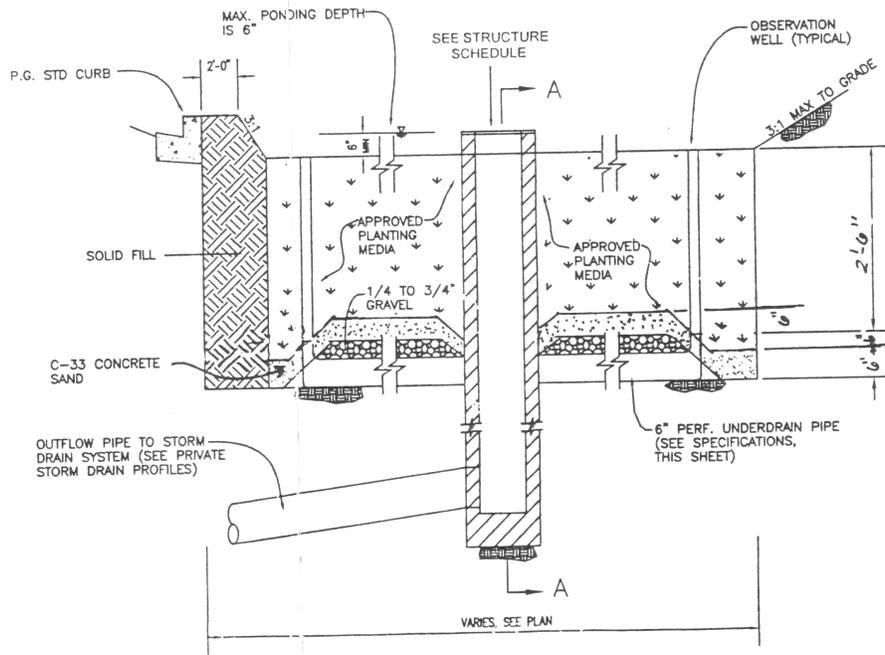
TYPICAL SECTION THROUGH BIORETENTION FACILITY
