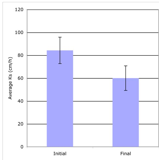
Figure 3.3: Average saturated hydraulic conductivity for Control group. Error bars indicate the standard deviation from the mean. Average initial saturated hydraulic conductivity was  $84 \pm 12$  cm/h. Average final saturated hydraulic conductivity was  $60 \pm 11$  cm/h.
