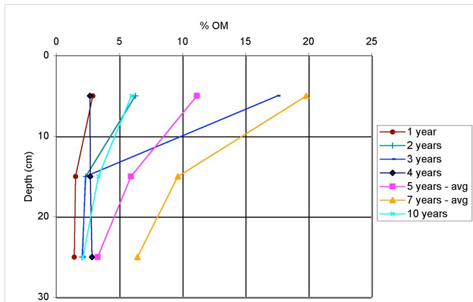
Figure 2.57: Soil organic matter profile development over time. Data series are plotted with organic matter increasing to the right, and depth increasing downward, so that the soil surface is at the top of the chart. The 5-year profile was derived by averaging data from the CBF and NWHS sites. The 7-year profile was derived by averaging data from the CC and BP sites.
