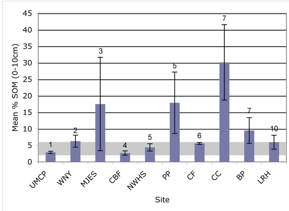
Figure 2.55: Mean upper layer % SOM for all sites. Error bars show standard deviations. The shaded area represents the expected organic matter content of a typical BSM soil medium (2–6%).
