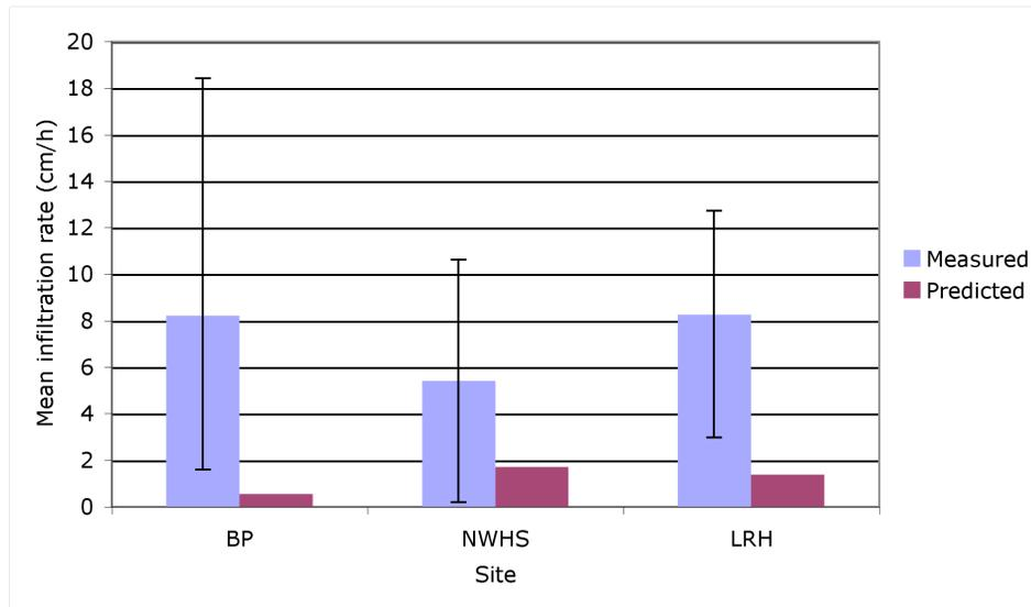
Figure 2.56: Comparison of measured versus predicted infiltration rates for the sites sampled. The measured value is the mean, and the error bars represent the maximum and minimum measured values. Predicted values represent the effective infiltration rate for the soil textures measured onsite, based on Rawls et al. (1982).
