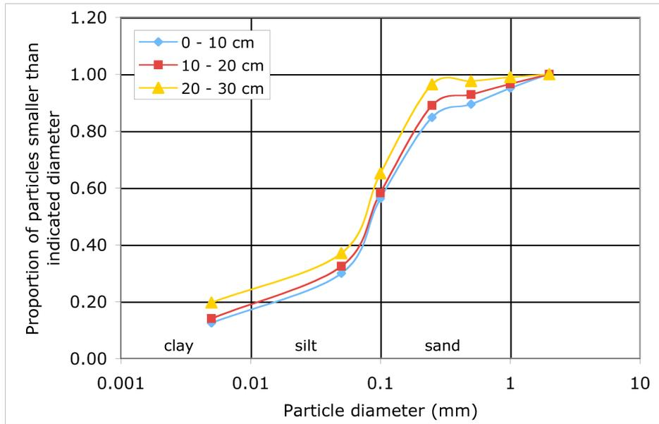
Figure 2.40: CF particle size distribution.
