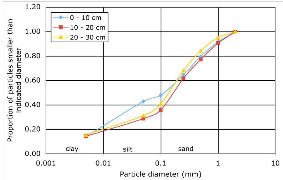
Figure 2.28: MJES particle size distribution.
