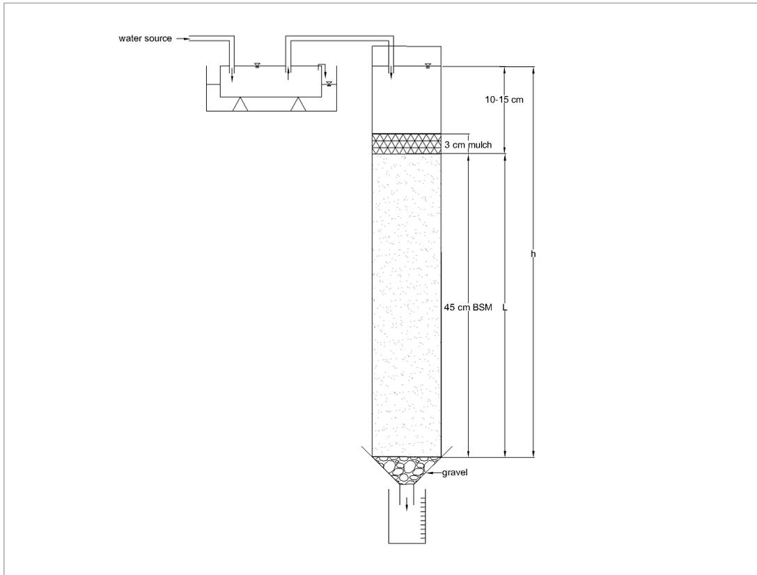
Figure 3.2: Diagram of setup to establish constant head for infiltration testing.
