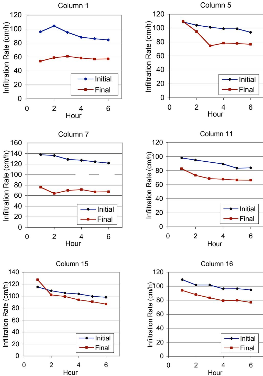
Figure 3.12: Results of initial and final infiltration tests for Control group showing declining infiltration rates over the course of the tests.
