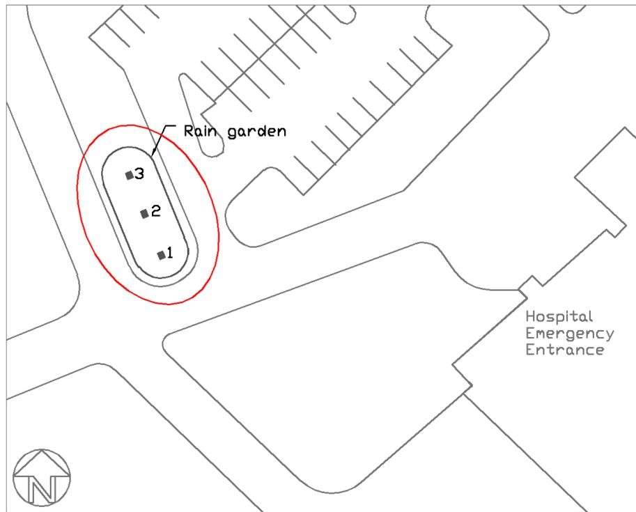
Figure 2.21: LRH site planview. The rain garden of interest is circled, and the sampling locations (1,2, and 3) are indicated.
