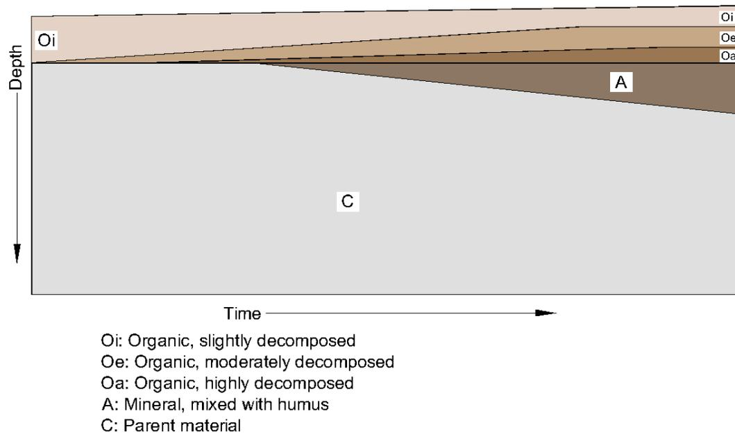
Figure 1.2: Initial stages of pedogenesis, after Brady and Weil (2002). An organic horizon (O) forms at the soil surface, and is gradually broken down and incorporated into the uppermost soil layer, forming an A horizon.
