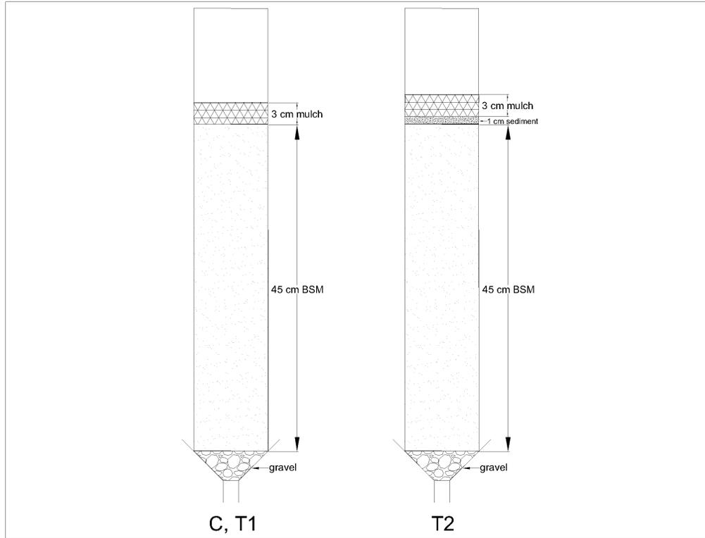
Figure 3.1: Diagram showing microcosm setup.
