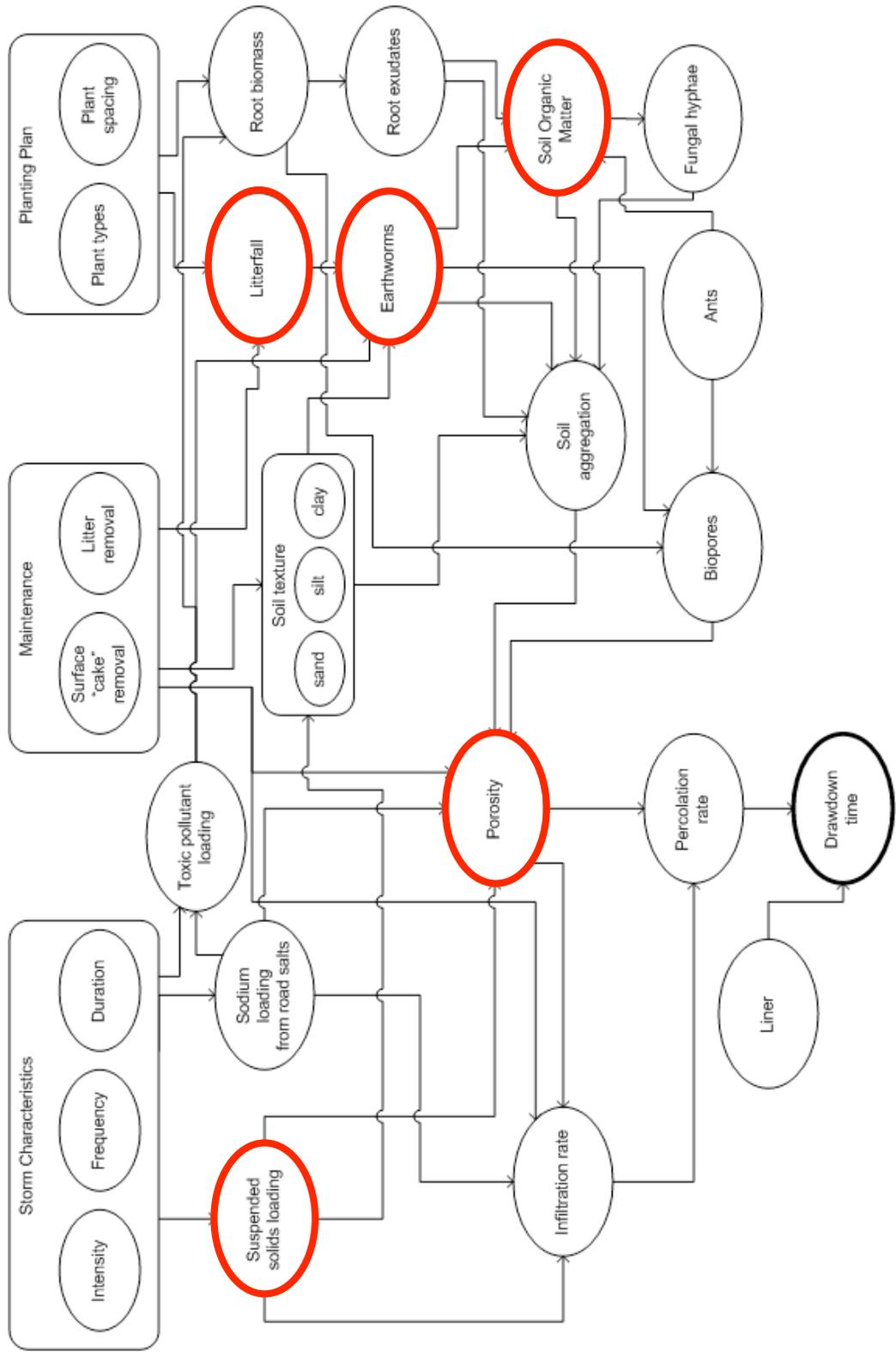
Figure 5.1: Factors influencing the drawdown time of a rain garden, with emphasis on those factors included in the simulation model.
