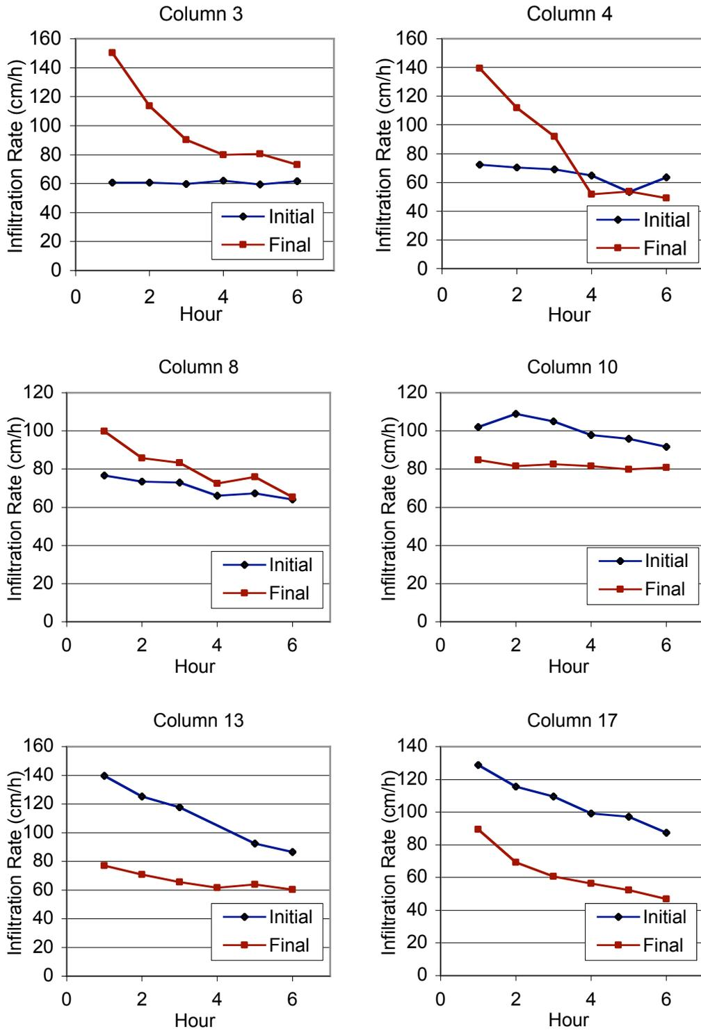
Figure 3.14: Results of initial and final infiltration tests for Treatment 2 group showing decreasing infiltration rates over the course of the tests.
