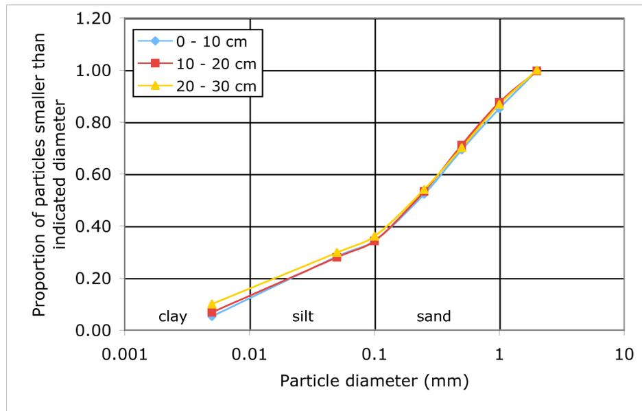
Figure 2.25: WNY particle size distribution.
