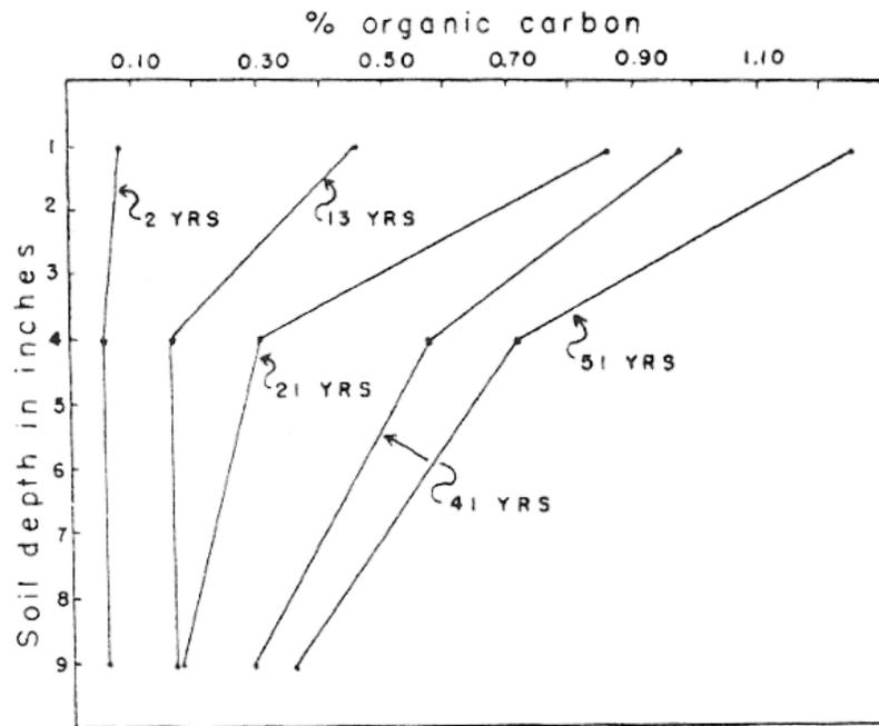
Figure 2.58: Organic carbon profile development in a mine spoil chronosequence (Leisman, 1957).
