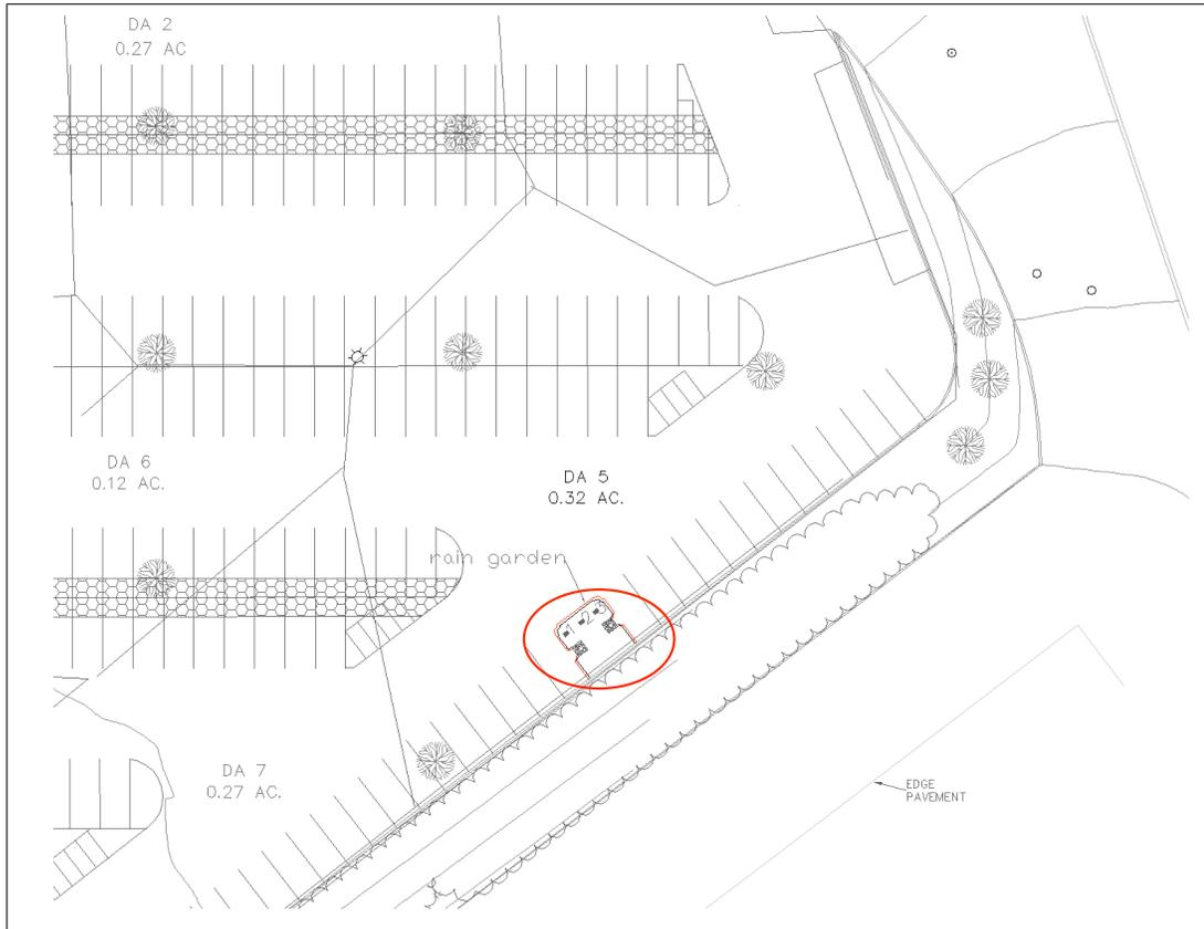
Figure 2.5: WNY site planview (source: The Low Impact Development Center, Inc.). The rain garden of interest is circled, and the sampling locations (1,2, and 3) are indicated.
