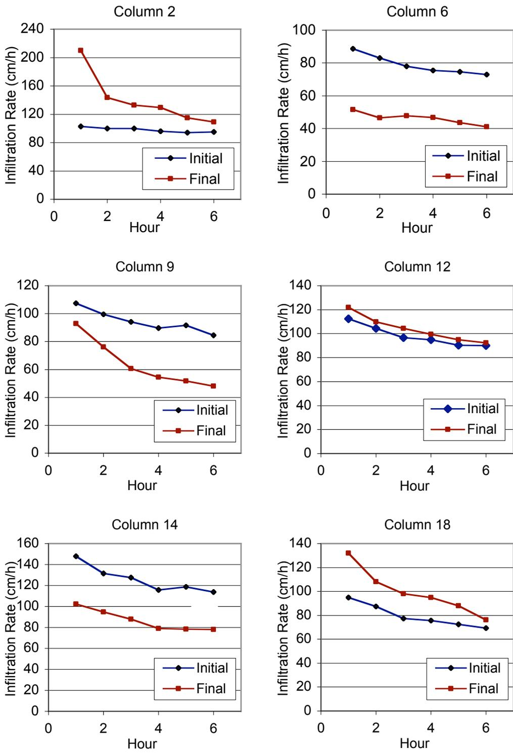
Figure 3.13: Results of initial and final infiltration tests for Treatment 1 group showing declining infiltration rates over the course of the tests.
