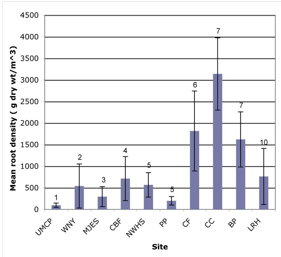
Figure 2.52: Mean root density for all research sites. Error bars represent the standard deviation between sampling locations. Numbers above each column indicate the age of the rain garden in years at the time of sampling.
