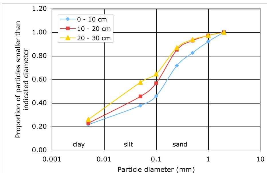
Figure 2.46: BP particle size distribution.
