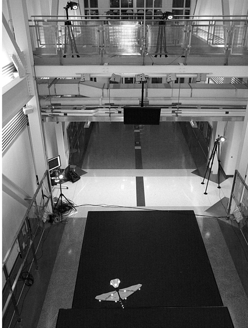
Figure 4.5: Flight testing experimental setup for wing aerodynamics modeling
