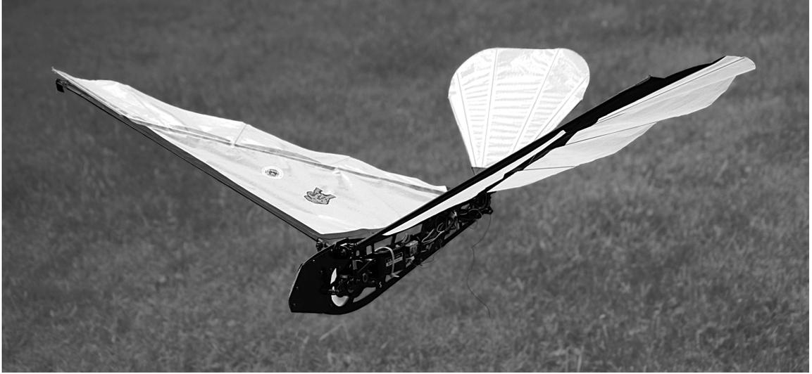
Figure 2.2: Ornithopter flight test platform
