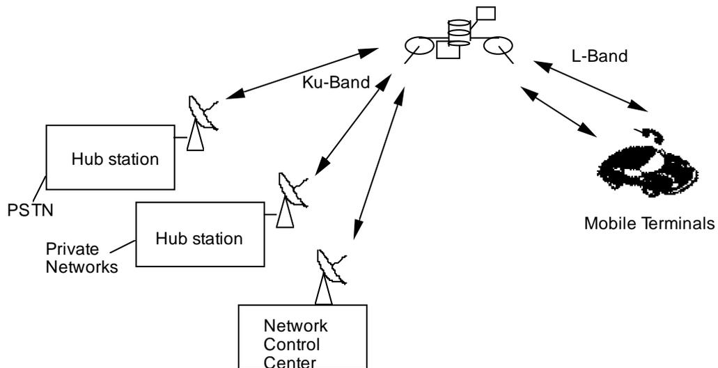
**Figure 17. Mobile Satellite Network**
