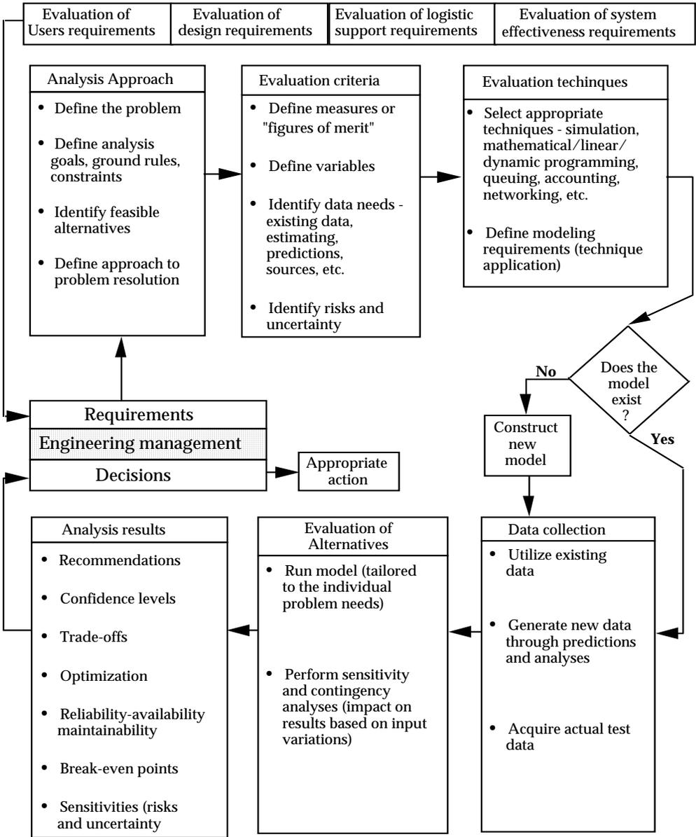
Figure C..1 The systems analysis process (Blanchard and Fabrycky, 1985)
