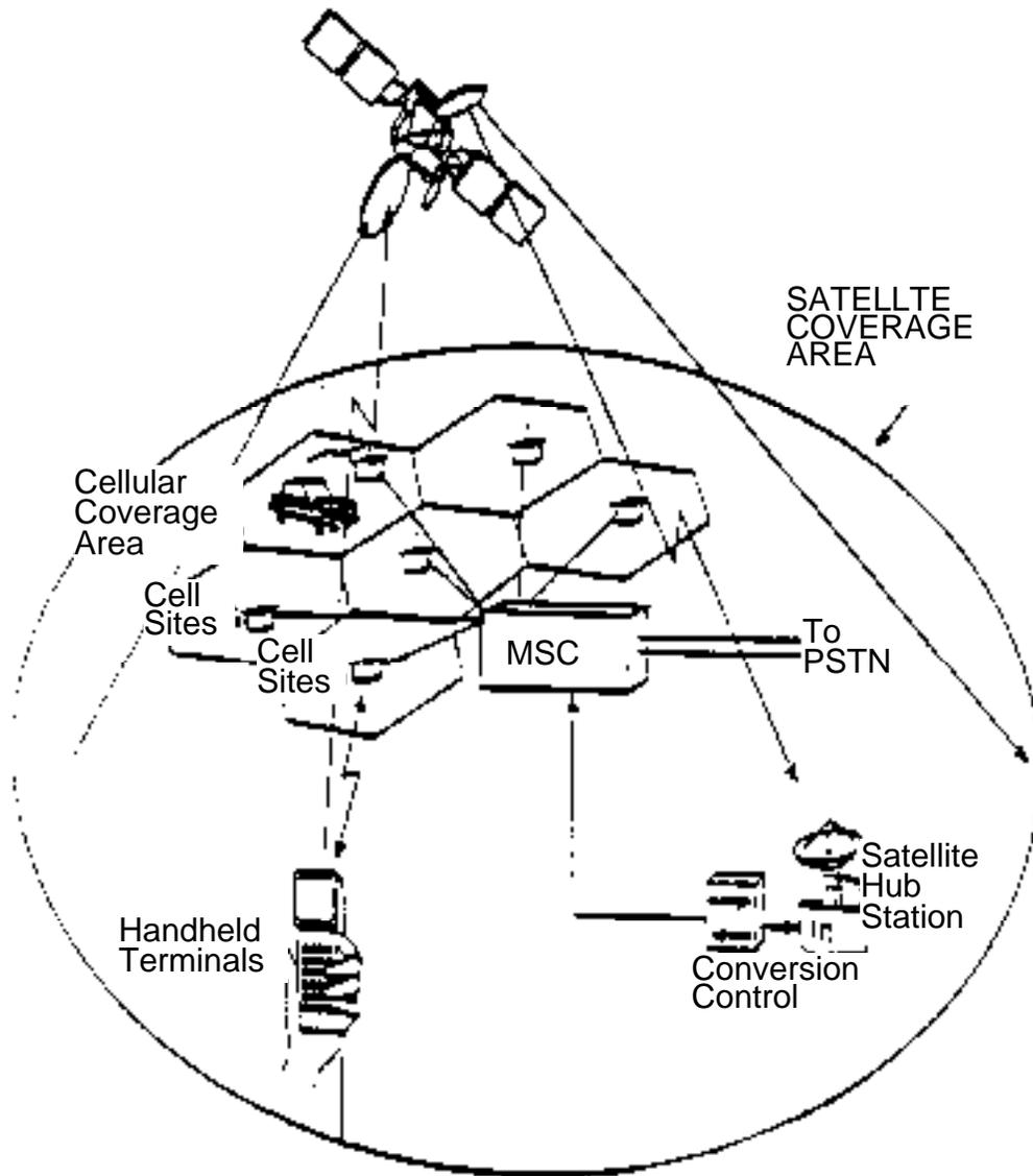
**Figure 18. Hybrid Cellular Satellite Network**
