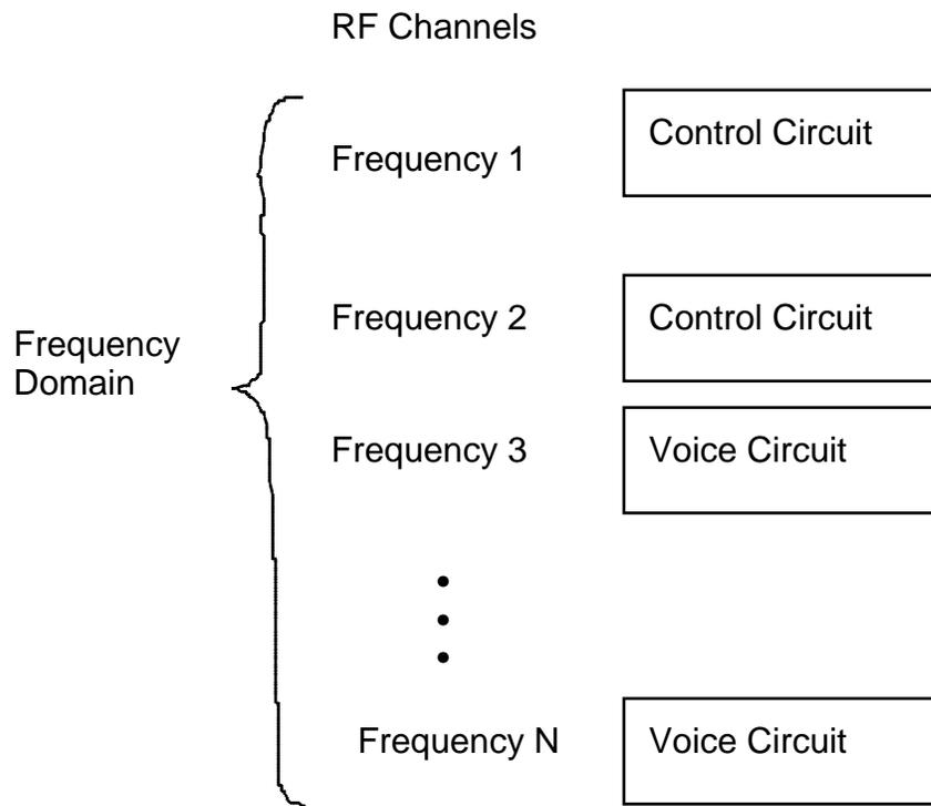
**Figure 4. FDMA Cellular System Architecture**
