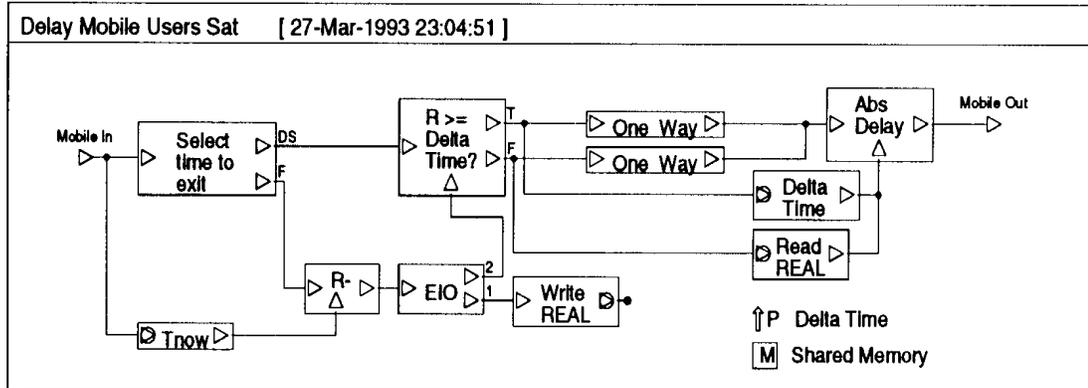
**Figure 36. Delay Sat Mobile Users**
