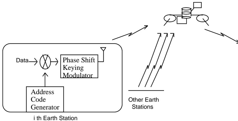
**Figure 16. CDMA Satellite System Architecture**
