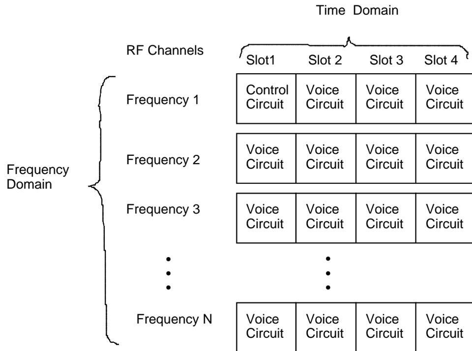
**Figure 5. TDMA Cellular System Architecture**
