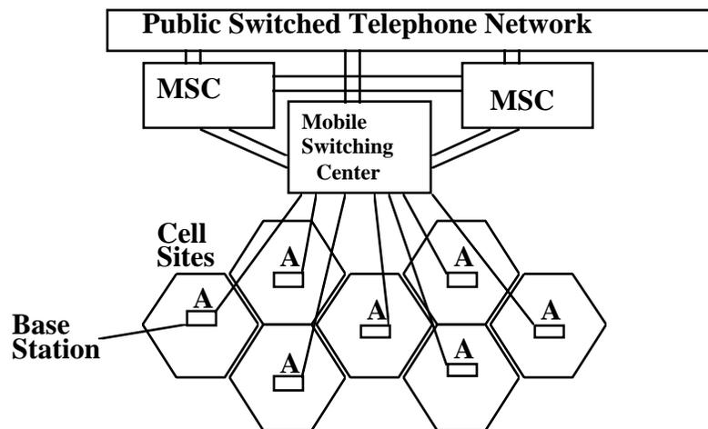
Figure 1. Cellular System Structure
