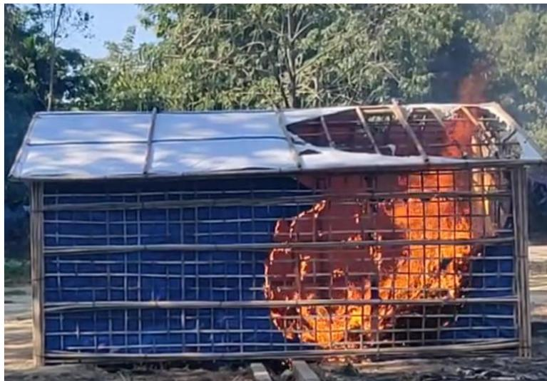
Figure 4-1. The Shelter 2 tarp on the roof and walls has burnt away, and the flame tip extends past the height of the roof. Timestamp: 62.45 seconds.
