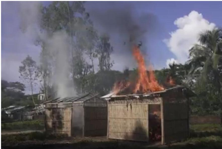
Figure 1-8. Burn tests with shelters built with bamboo framing, woven-bamboo walls, and a tarp roof (photo ownership Mehedi Rahman).
