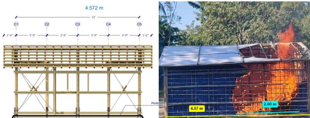
Figure 3-2. NFI Shelter plans (left) were used to calibrate measurements of Shelter 2 in Kinovea (right).
