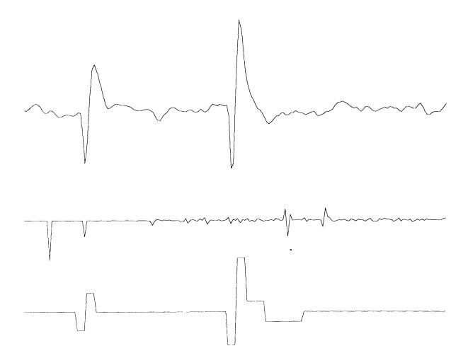
Figure 2: Spikers Detected by the Haar Transform: a) The origional trance. b) The transform domain equivalence, large components imply that there are spikes. c) Reconstructed spikes in the time domain, the noise is filled out, the spikes are detected by zero-crossing detection.
