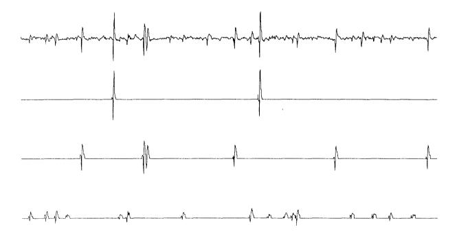
Figure 3: Spikers Classified by the System: a) The original trance. b) Class 1. c) Class 2. d) Rest of spikes.
