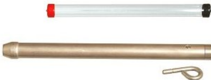
Figure 2.3 – The zero-contamination plastic tube is inserted in the metal bottom part of the sampler to hold the composite soil samples.
