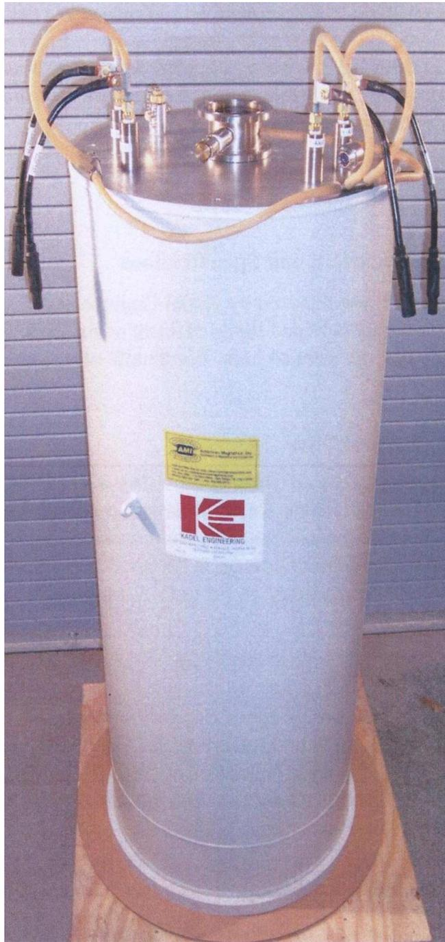
Figure 1.14: Two axis superconducting magnet dewar.
